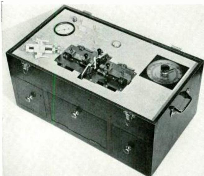
Fig. 3—Soldering machine designed for making wire-supported crystals
