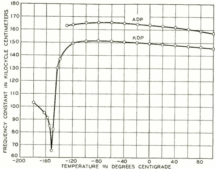
Fig. 2—Frequency constants of ADP and KDP plates, with variations in temperature. The dip in the KDP curve at -151 degrees C. indicates the incidence of "Ferroelectric" coupling
