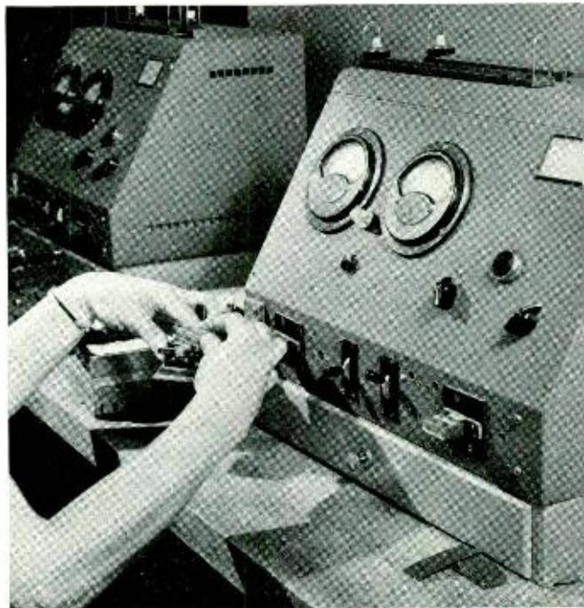
Fig. 2—The crystals are calibrated in test positions, where calibrators as shown above are connected by coaxial cable to the sub-harmonic generators. The calibrating circuit is shown in Fig. 3
