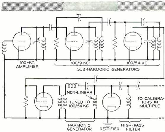
Fig. 1—Simplified schematic of the circuit of the sub-harmonic generator used in deriving a fifty-fourth sub-multiple frequency
