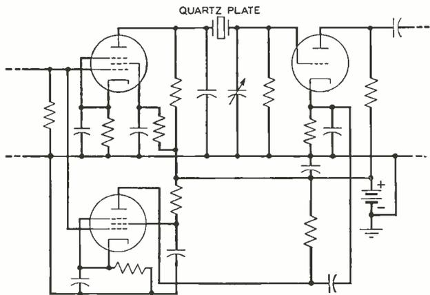
Fig. 4—Schematic of the filter
