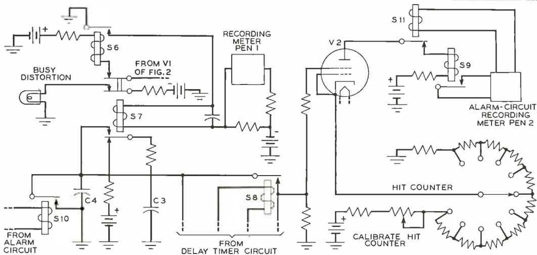
Fig. 3—Simplified schematic of the hit counter circuit
