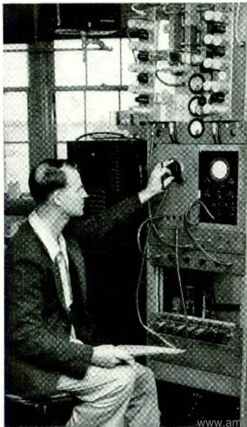
L. E. Hunt of Radio Research, at work in our Deal laboratory. He is using a microwave generator arranged to sweep through a range of several megacycles. By putting a synchronized sweep voltage on one set of plates of an oscilloscope, and the output of a circuit under test on the other set, the experimenter can see on the 'scope a transmission-vs.-frequency curve of the circuit.
