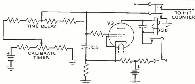
Fig. 4—Simplified schematic of the delay timer circuit
