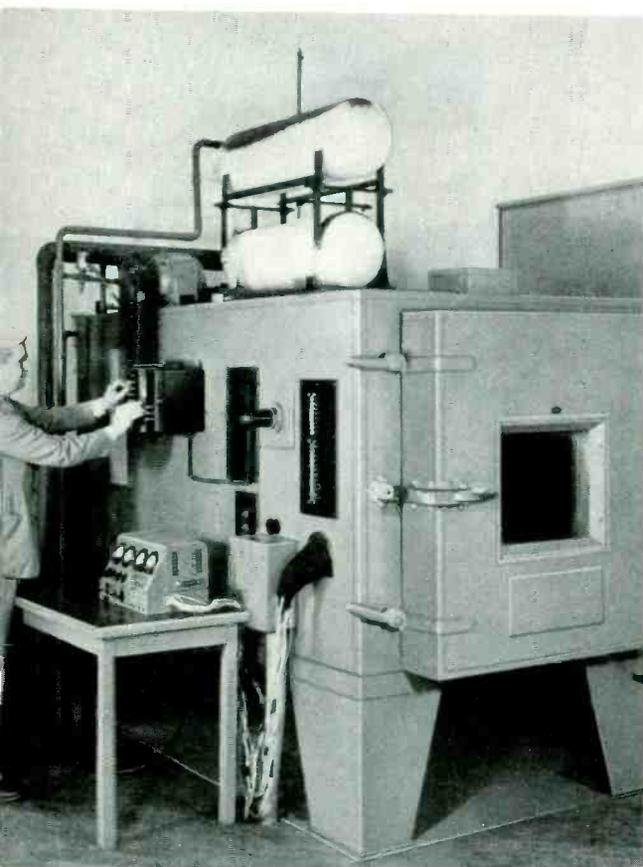
chipped "dry ice" in a tank of Varsol, and then pumping the cold Varsol into a cooling tank in the top of the chamber. It is used for tests requiring temperatures between  $-40$  degrees F. and  $+180$  degrees F. and relative humidities up to 95 per cent at 150 degrees F. This chamber also has found application for tests on components and small assemblies, and long-term relative humidity tests, many of them involving altitude and temperature cycling.
