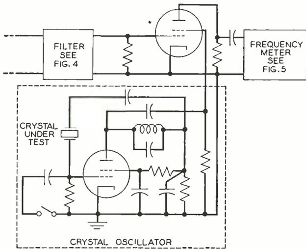
Fig. 3—Simplified schematic of the calibrator circuit
