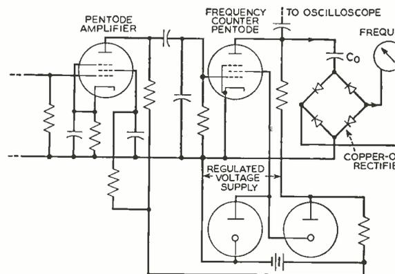
Fig. 5—Schematic of the frequency meter
