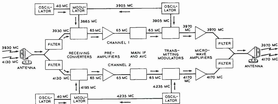
Fig. 3—Block schematic of two-channel repeater
