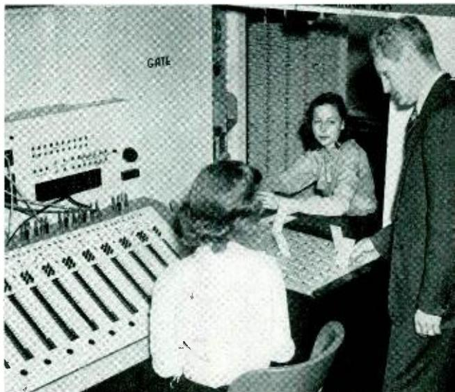
R. I. Wilkinson observing the process of starting a call in the machine on which the load carrying capacity of No. 5 exchanges is being explored. With him are left, Catherine Durnan, who handles the marker position, and Mary Tracy, who originates the calls and determines which subscriber lines are idle or busy
