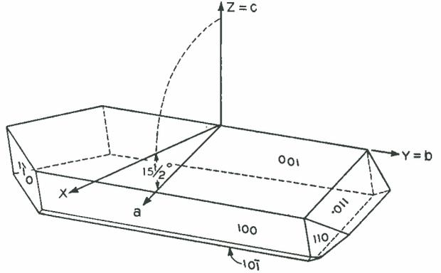
Fig. 1—EDT crystals are classified as monoclinic. They have two axis, a and c, with a 105-degree angle between them and a third axis, b, perpendicular to the others and parallel to the crystal's length
