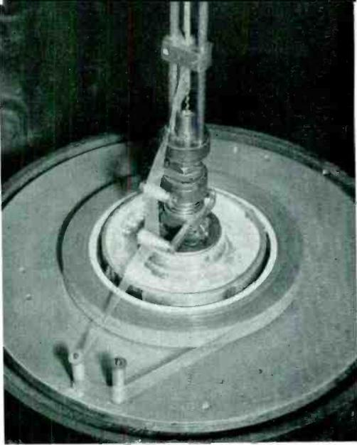
*Fig. 4—Close-up of the tape insulator showing the application of the polyethylene tape over the string insulated wire*
