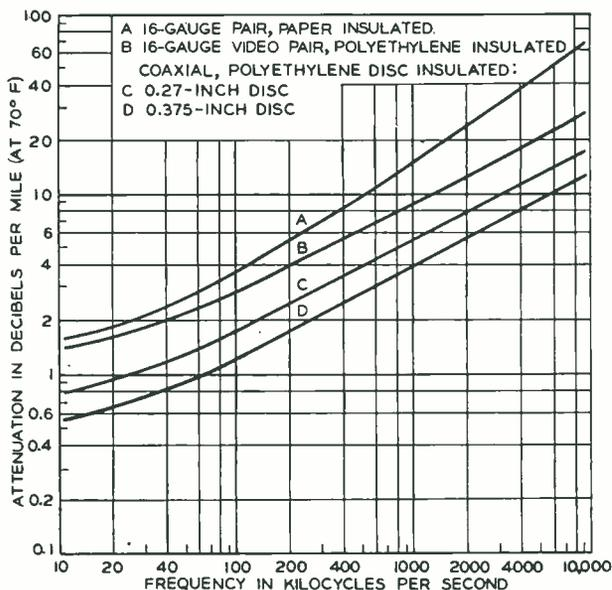
Fig. 6—Attenuation of a video pair compared with other types of circuits at video frequencies
