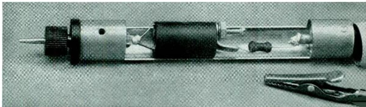
Fig. 1—The 598A tool for high impedance probing
