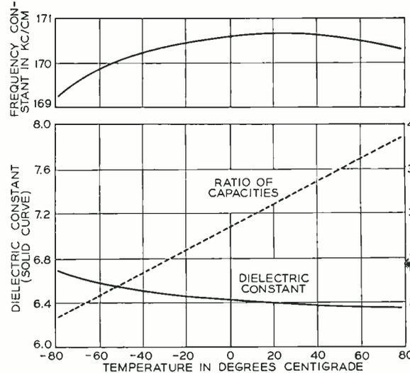
Fig. 5—Characteristics of the A cut EDT crystal. frequency variation with changes of temperature is half that of the Y cut
