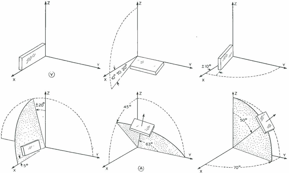
Fig. 2—There are six orientations in EDT crystals at which crystal plates with zero temperature coefficients can be cut. Two have been designated A and Y.
