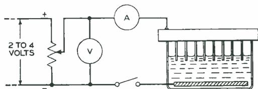
Fig. 4—Electropointing circuit. A potential difference is maintained between the tungsten wires and the cathode throughout the pointing action
