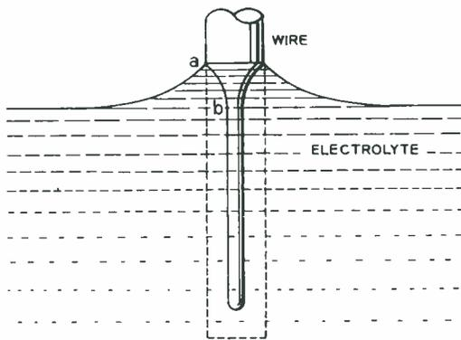
Fig. 2—Drawing of tungsten wire at one stage of the pointing action. The decreased rate of solution inside the meniscus results in the taper between a and b
