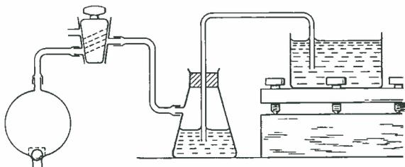
Fig. 5—Pump-siphon apparatus for variation of the level of the electrolyte. Pressure from the rubber bulb forces liquid from the auxiliary container into the main vessel. Reversing the stopcock permit the liquid to siphon back
