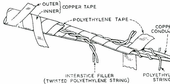
Fig. 2—Section of video pair showing construction details of the various elements
