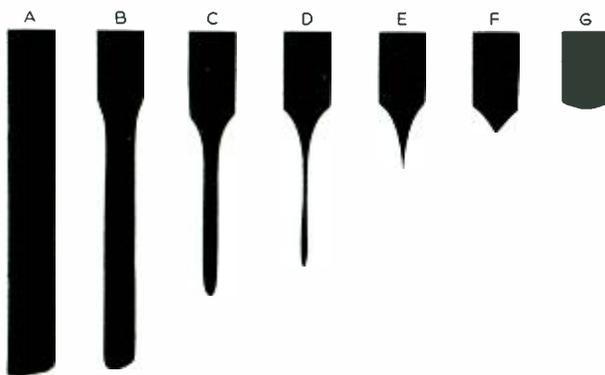
Fig. 3—Photomicrographs of 0.005 inch tungsten wires at successive stages of anodic solution. Contour F is most representative of those used in point contact rectifiers. Magnification—100X
