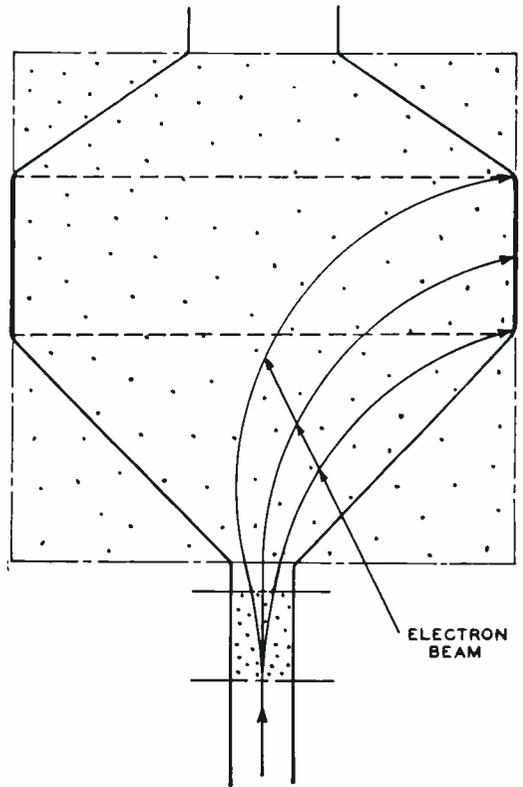
Fig. 3—Cross section of the tube in the plane of electron beam showing schematically the bending the beam
