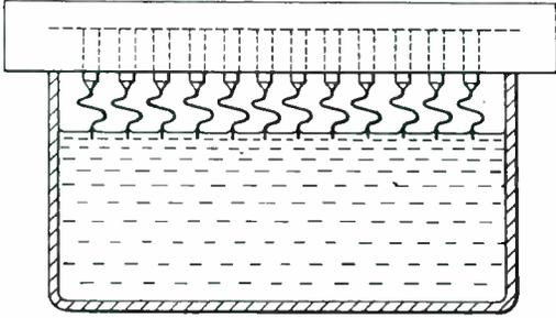
Fig. 6—Method of mounting spring assemblies. If the holder is horizontal all the springs will have the same length when pointed. In practice 40 to 100 wires are pointed simultaneously
