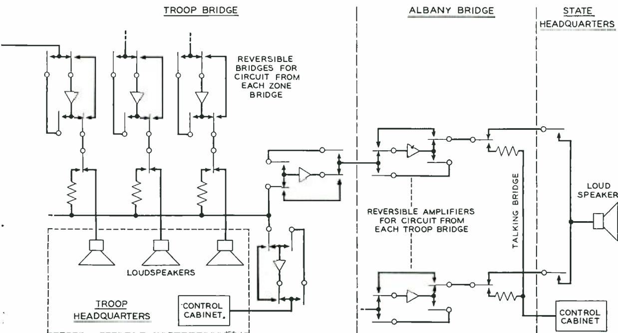
Albany asks an operator for the troop desired, and that circuit is then transferred through its relay to the Albany bridge. Should the person wish to talk to a particular zone rather than to an entire troop area, he can direct the required switching at the troop bridge.
