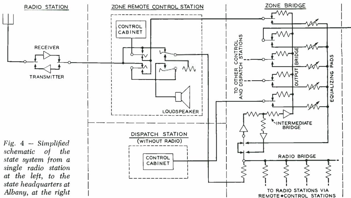
Fig. 4 - Simplified schematic of the state system from a single radio station at the left, to the state headquarters at Albany, at the right
