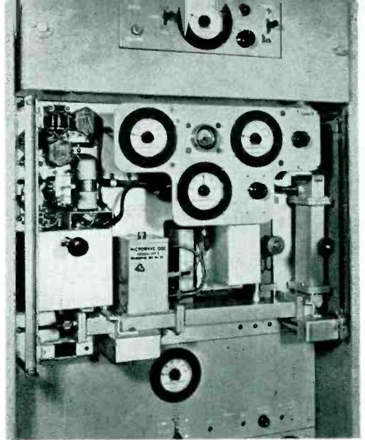
Fig. 6—Front view of stabilized microwave oscillator panel
