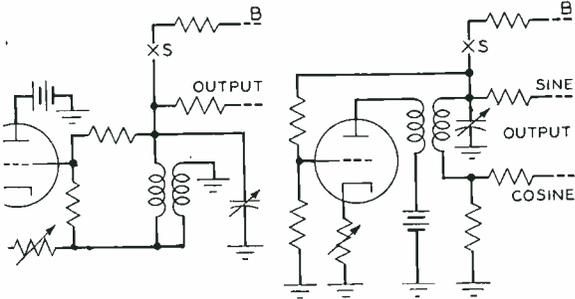
Fig. 1—Two forms of the start-stop oscillator circuit
