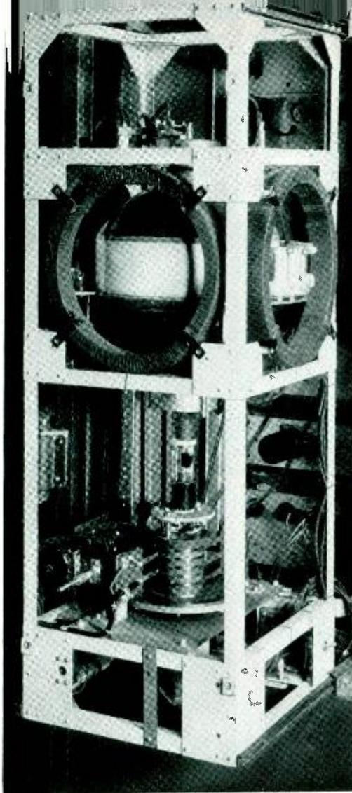
Fig. 2—With the mounting rack removed from the equipment cabinet the translator is seen positioned in its carriage. All but the viewing section, within the area of the forefront of the control coils, is covered during normal equipment operation
