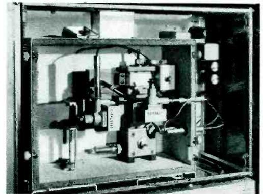
Fig. 7—Rear view of stabilized oscillator panel
