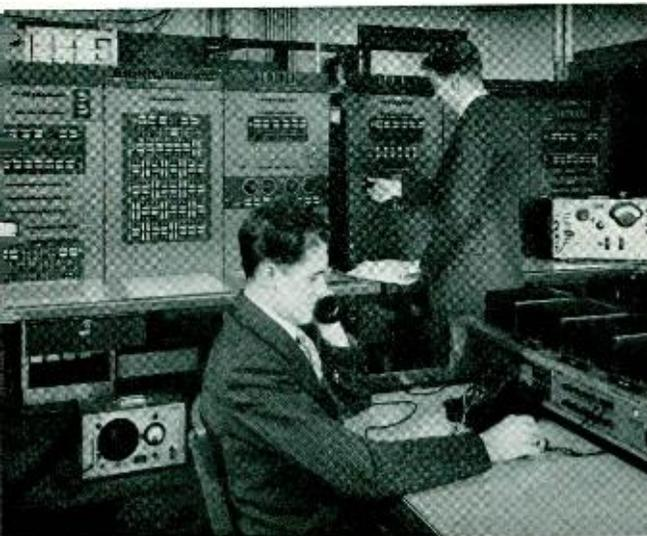
*Fig. 2—The circuit simulator panels at the rear and a terminal position in the right foreground*
