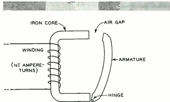
Fig. 1—Generalized form of relay
