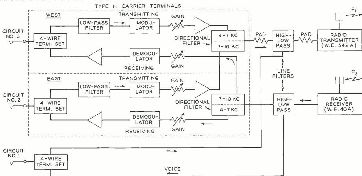
Fig. 2—Application of two Type-II systems to a radio terminal
