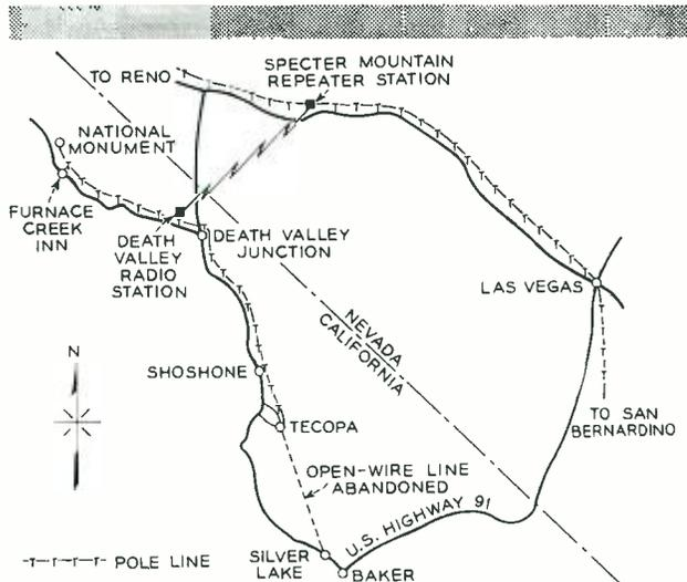
Fig. 1—How the radio link is integrated into the wire network. Telephones in Death Valley can ring each other; operator assistance is given in San Bernardino
