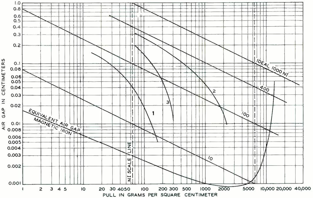
Fig. 2—Curves for studying relay operation
