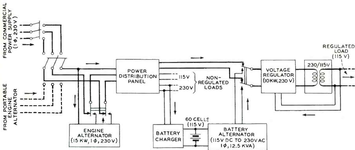
Fig. 8—Power supply diagram for the repeater stations
