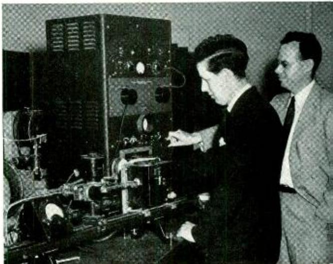
*C. Kittel demonstrates magnetic resonance absorption in a paramagnetic salt to Dr. Bleaney of the Clarendon Laboratory of the University of Oxford*
