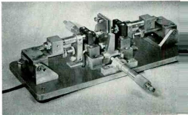
*Fig. 8—Lead wire soldering tool with a plate holder containing an EDT crystal plate, with disks already attached, in center position. This tool, by interchangeable noses, is also used to attach the combination adhesive disks to the plate. Each headed wire registers in accurate alignment on its corresponding disk and is soldered in a radiation heat cycle for minimum thermal stress*
