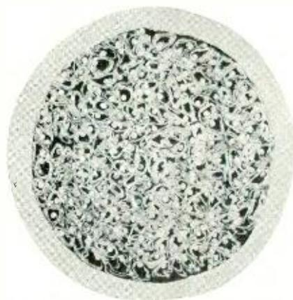
*Fig. 2—Cross-section of 100-pair, No. 19 gauge, dry-core paper-insulated cable of 1892, with an extruded lead sheath*
