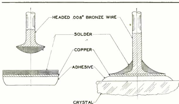
Fig. 4—Left, below, combination adhesive disk before cementing to EDT plate. Left, above, headed wire that will be soldered to the disk's solder layer. Right, combination adhesive disk after cementing to EDT plate and after headed wire has been soldered to the solder layer. Note overlap of adhesive that furnishes proper surface for electrical continuity between mounting wire and gold electrode
