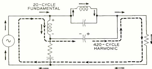
Fig. 6—Current paths for fundamental and harmonics
