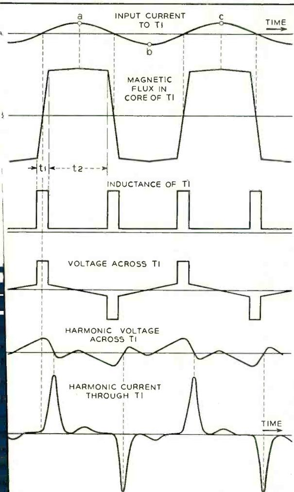
Fig. 4—Idealized curves of current, voltage, and inductance referred to in the description of audible ringing generation
