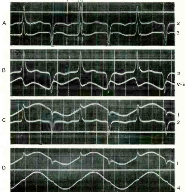
Fig. 5—Oscillograms of currents and voltages in harmonic generator network. Numbers at right indicate points at which measurements were made
