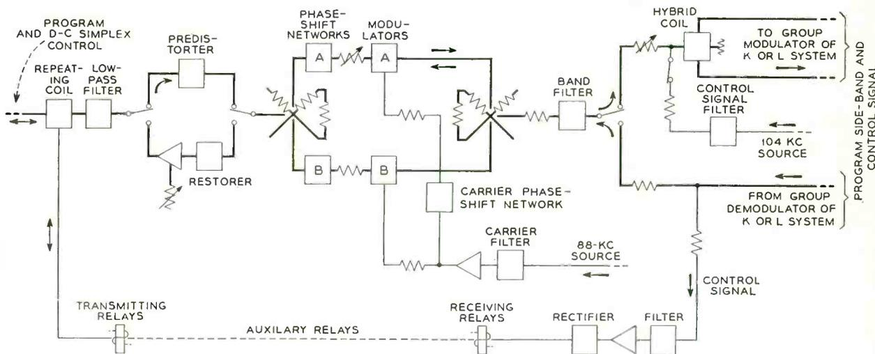
Fig. 4—Block schematic of a reversible terminal
