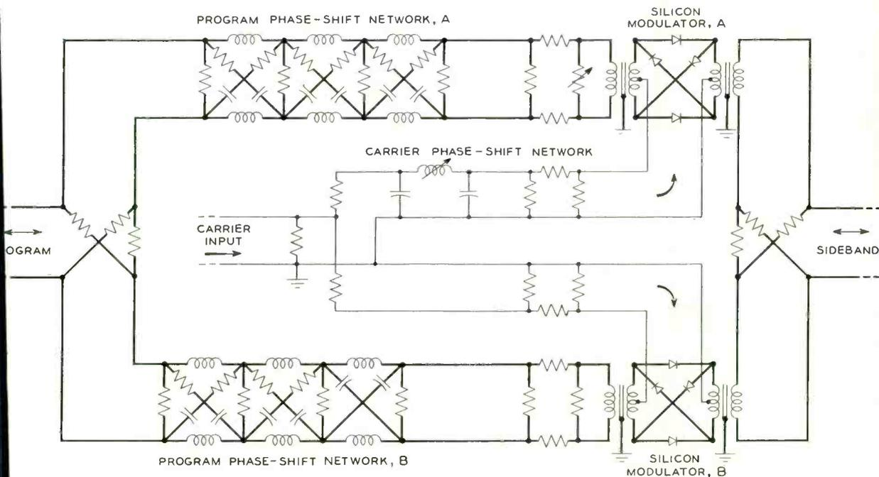
Fig. 1—Modulating circuit for the 15-kc program terminal
