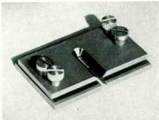
*Fig. 6—An EDT plate holder in which plates are friction held. It accommodates any size of plate up to 1½ inches in length, 1¼ inches in width, and 3/16 inch in thickness, provides the mechanical protection needed by the plate, and insures a more uniform heating and cooling rate to minimize plate fracture from thermal heat*
