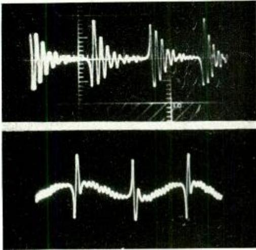
Fig. 8—Oscillograms of ringing voltage applied to the calling subscriber. The no-load condition is shown above and full load, below
