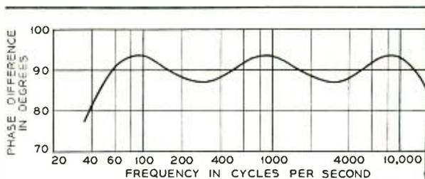
Fig. 3—Difference in insertion phase between networks A and B
