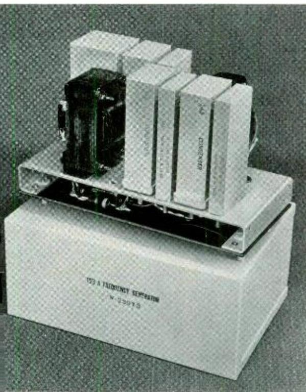
Fig. 1—The 103A frequency generator resting on the case in which it is housed when in use
