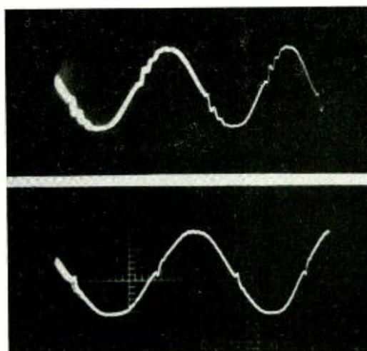
Fig. 7—Oscillograms of voltage at generator output terminals. The no-load condition is shown above and full load, below
