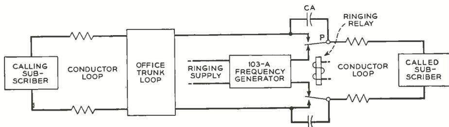
Fig. 2—Method of applying ringing current to the called line and audible ringing to the calling line
