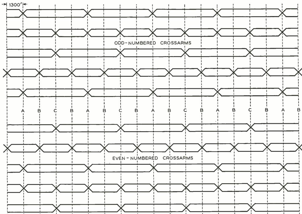
Fig. 1—The ABC transposition system, shown above, was the first to result commercially from Barrett's invention
