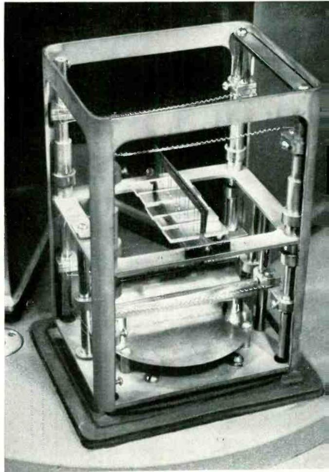
*Fig. 10—Inside view of vacuum chamber showing arrangement used to vapor plate gold electrodes on EDT crystal plates. The small diameter wire coils, two of which are visible at top of fixture, are tungsten heaters in which solid gold wire is threaded. After high vacuum is attained, these heaters are made incandescent and the gold evaporates to cover the crystal plates with a film approximately 15 millionths of an inch thick*
