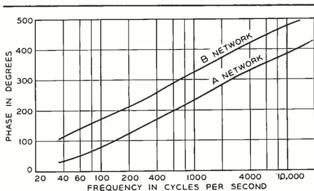
Fig. 2—Insertion phase shift of networks A and B
