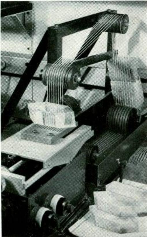
*Fig. 2—Laboratory production, by multiple wet-string saw, of Y-cut wafers from an EDT crystal bar. From these wafers, plates are shaped to required dimensions by additional wet abrasive methods*
