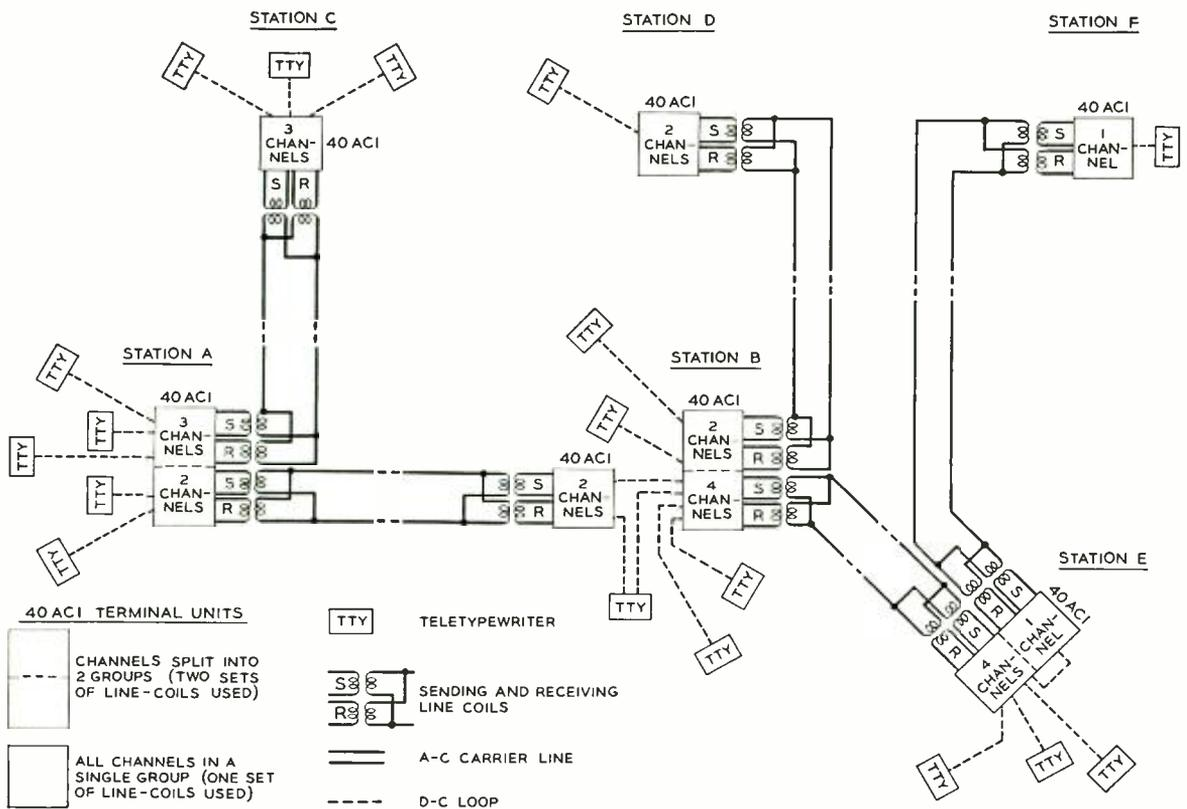
Fig. 2—Typical layout employing 40AC1 terminals
