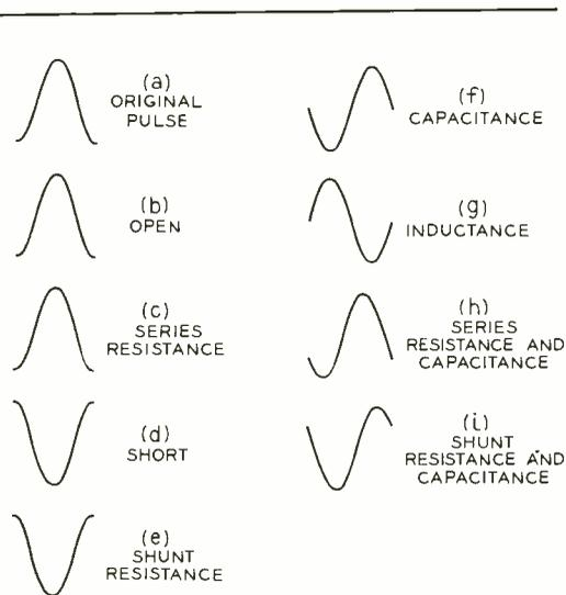
Fig. 6—Reflections or echoes resulting from various types of irregularities.
