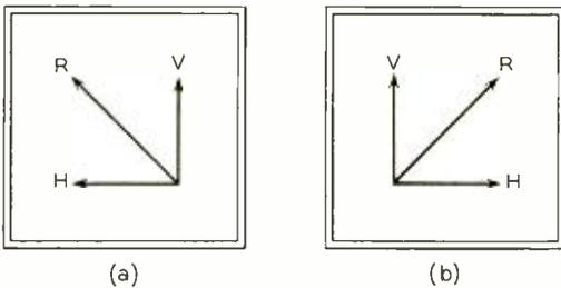
Fig. 6—Cross-section of hybrid unit showing resolution of diagonally polarized waves.
