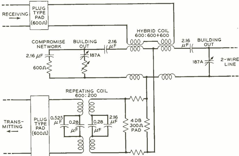
Fig. 6—Circuit schematic of the earlier four-wire terminating set. In this circuit, the differences described in the article may also be seen.
