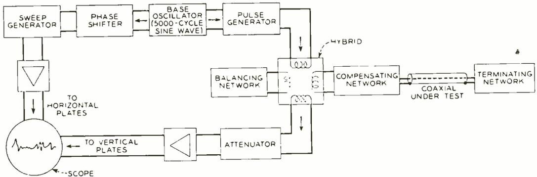
Fig. 2—Block diagram of pulse echo set.
