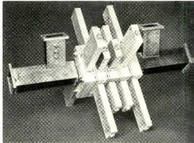
Fig. 7—A waveguide hybrid unit on each side of a delay and reflecting unit is the equivalent of Figure 2.
