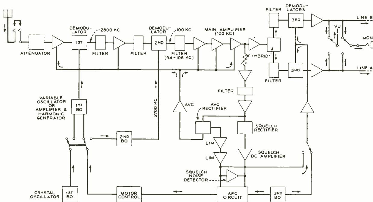
Fig. 1—Block schematic of the LD-R1 single sideband radio receiver.
