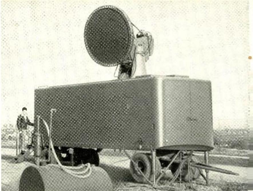
Development of a new and far more effective fire-control system for automatically aiming anti-aircraft artillery has been announced by the Laboratories, with the approval of the Army Ordnance Corps for whom the project was undertaken.
