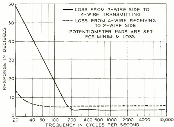
Fig. 2—Loss frequency characteristics of the new set measured between 600-ohm lines.
