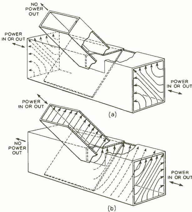
Fig. 5—Perspective drawing of the waveguide hybrid unit showing its effect on entering waves polarized in two directions.
