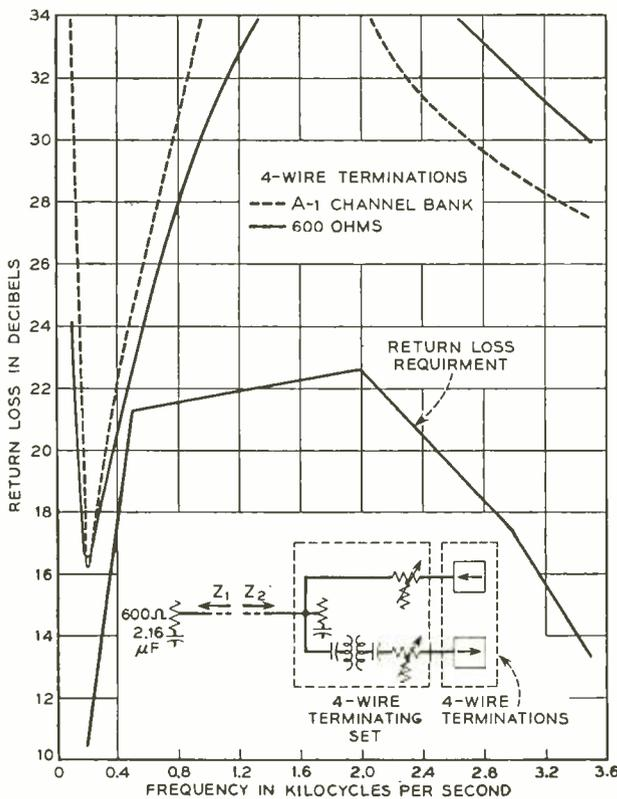
Fig. 5—Return loss characteristics: with channel bank termination; and with 600-ohm termination. The characteristics are well above the requirements.
