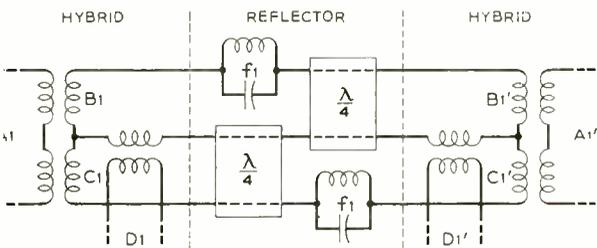
Fig. 2—A wire circuit analogy of the chain of a separating or combining filter unit.
