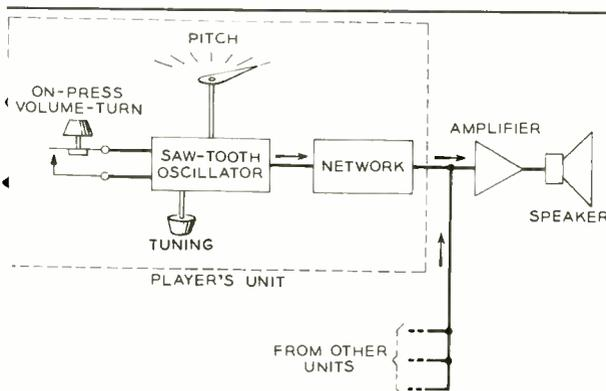
*Wobble arm controls pitch by varying potentiometer. Two other potentiometers control volume and tuning.*
