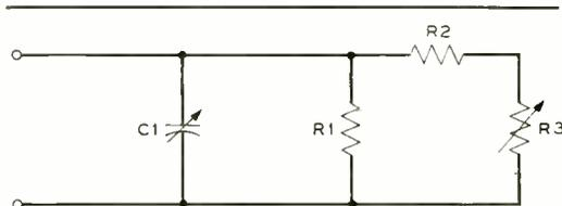
Fig. 5—Balancing network.
