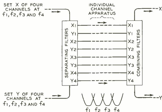
Fig. 1—A set of four incoming channels is connected to one end of the separating filter chain, and another set of four to the other end, and the eight individual channels are separated by the filter. In a similar manner, the chain of combining filters takes eight individual channels and forms two groups of four.
