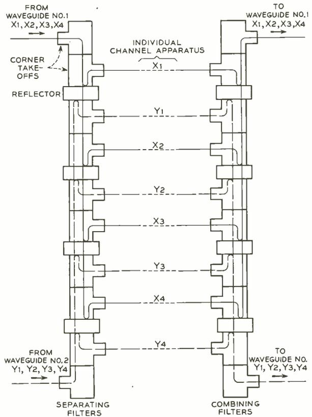
Fig. 8—Arrangement of waveguide units corresponding to Figure 1.
