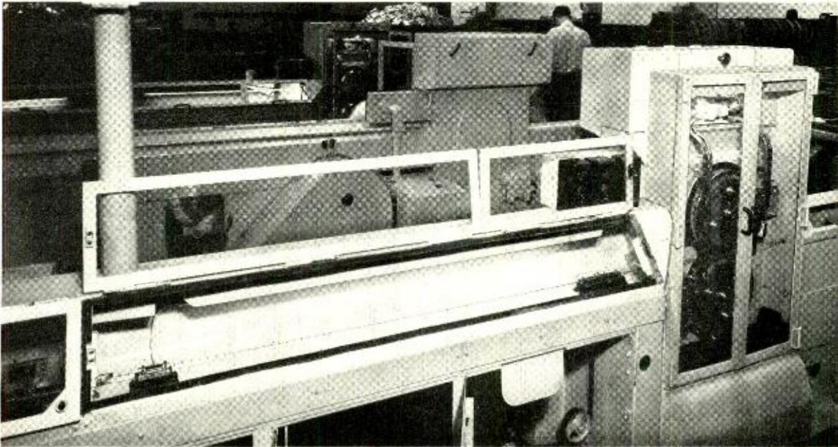
*Fig. 1—Coaxial forming machine showing insulated center conductor (lower foreground) passing through high-voltage electrodes.*
