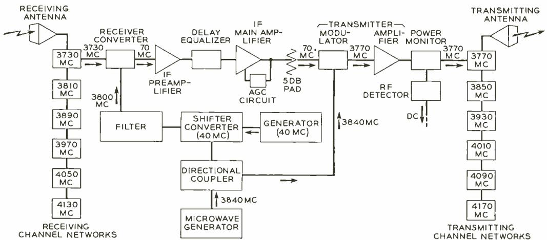
Fig. 1—Block schematic for an auxiliary repeater station.
