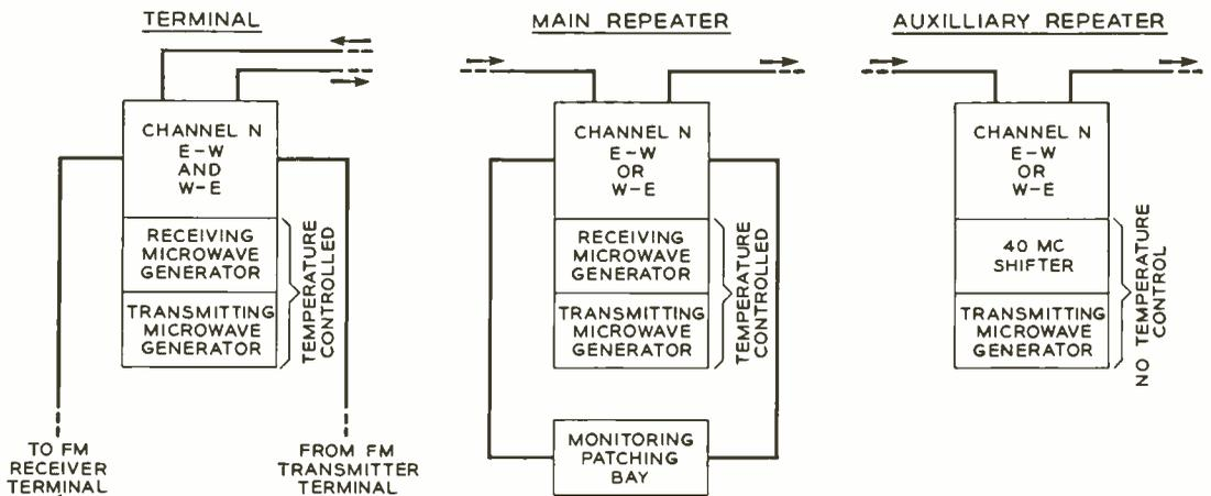
Fig. 4—Block schematic indicating the arrangement of the transmitter-receiver bay at terminal, main repeater station, and auxiliary repeater station.
