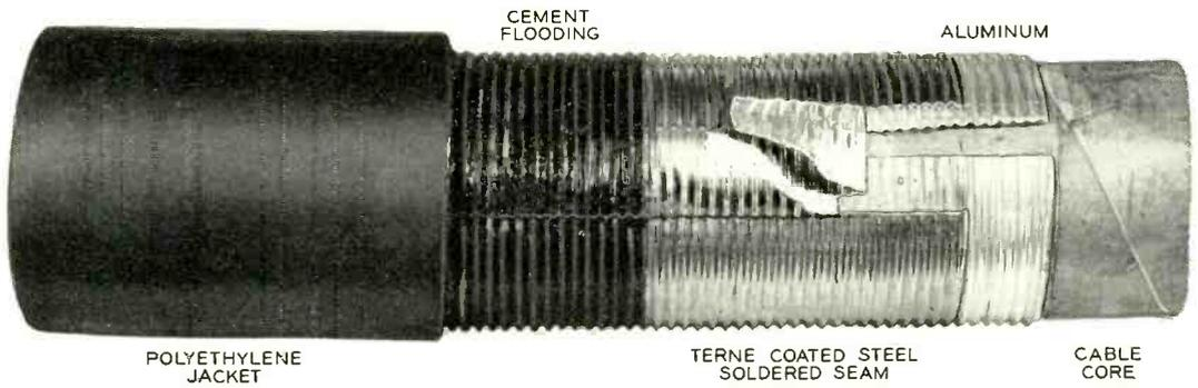
*In Stalpeth, a layer of terne plated steel is applied over the aluminum, and the seam is soldered.*
