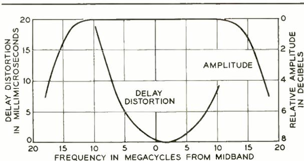
Fig. 2—Amplitude and delay characteristics of the repeater.
