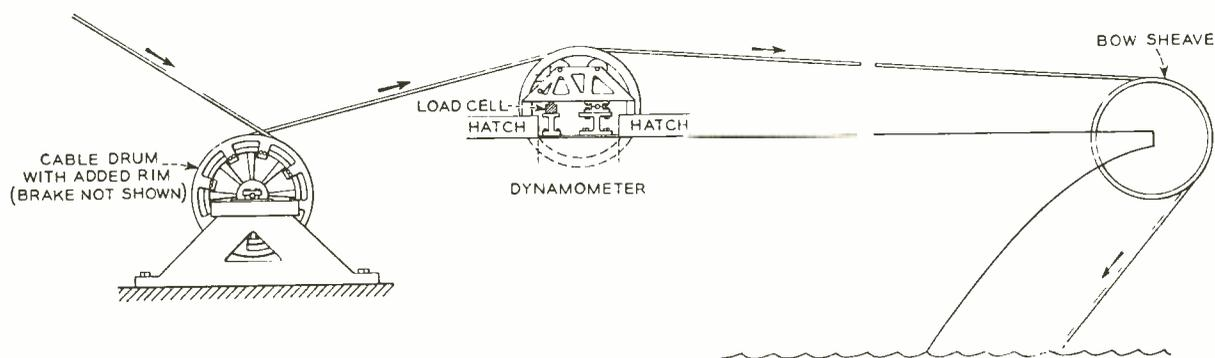
Fig. 3—Schematic of the improved dynamometer.
