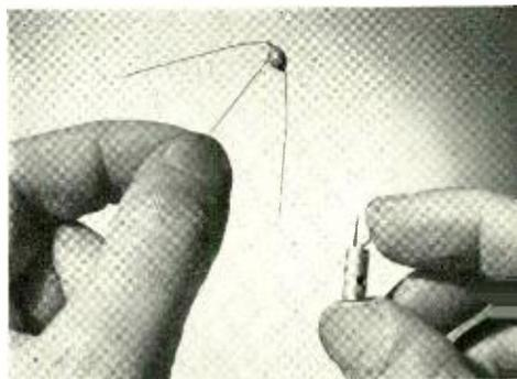
Significant advances in the development of the transistor, a tiny amplifying device which has been called the first serious rival of the vacuum tube, were recently announced by Bell Telephone Laboratories. The transistor was invented here three years ago. Most important of these advances is the construction of operating samples of a radically new type of transistor which has astonishing properties never before achieved in any amplifying device.
