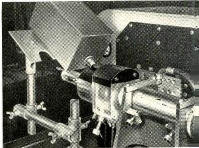
Fig. 3—Viewing unit in place for controlling a braze on a copper tube.
