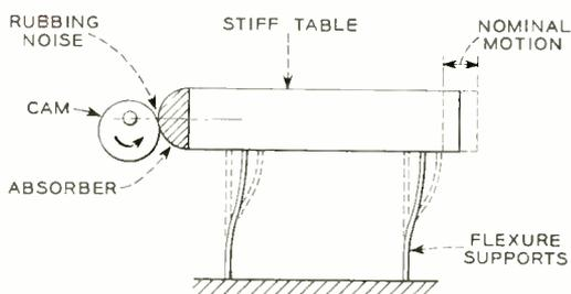
Fig. 4—Schematic arrangement of new leaf spring machine.
