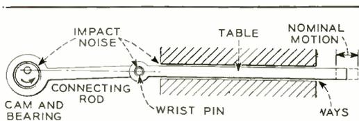
Fig. 2—Reciprocating vibration testing machine with table supported by guides or ways.
