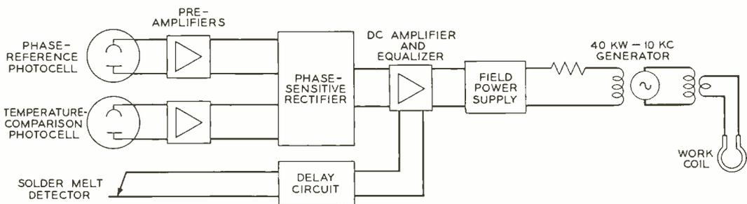
Fig. 5—Block diagram of temperature control system.
