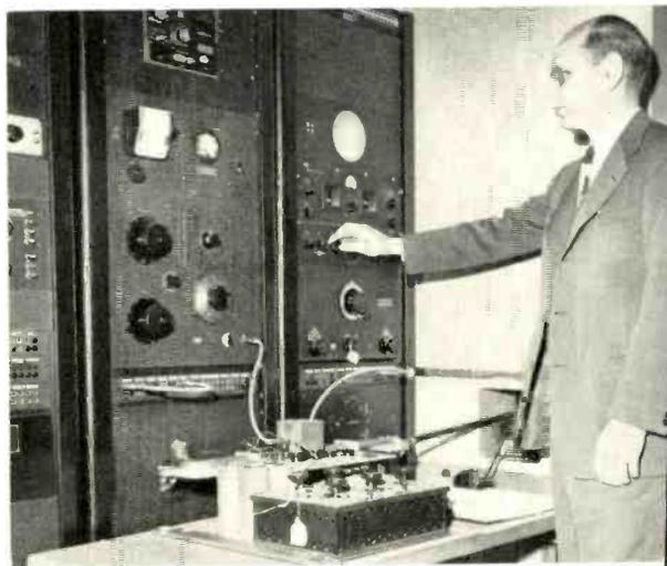
*Right, center, A. S. Windeler is making 140 kc frequency measurements of inductance and capacitance on an experimental shielded quad.*
