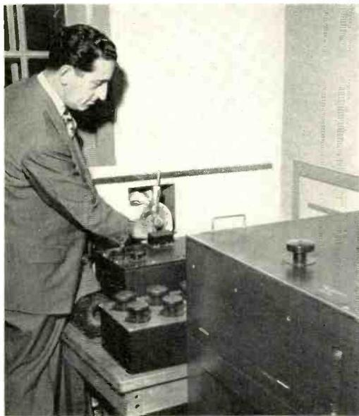
*Above right, G. I. Schaible is making connections to a cable under test preparatory to measuring the primary constants, i.e., inductance, resistance, capacitance, and conductance. These measurements will be made over a wide temperature range and at a frequency between 1 kc and 350 kc.*
