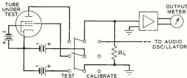
Fig. 1—Schematic circuit used for vibration tests.
