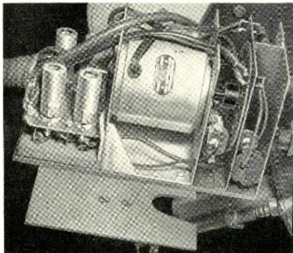
tions in the electrical circuit. With the disc rotating at 1800 rpm, the reference wave has a frequency of 600 cycles per second.
