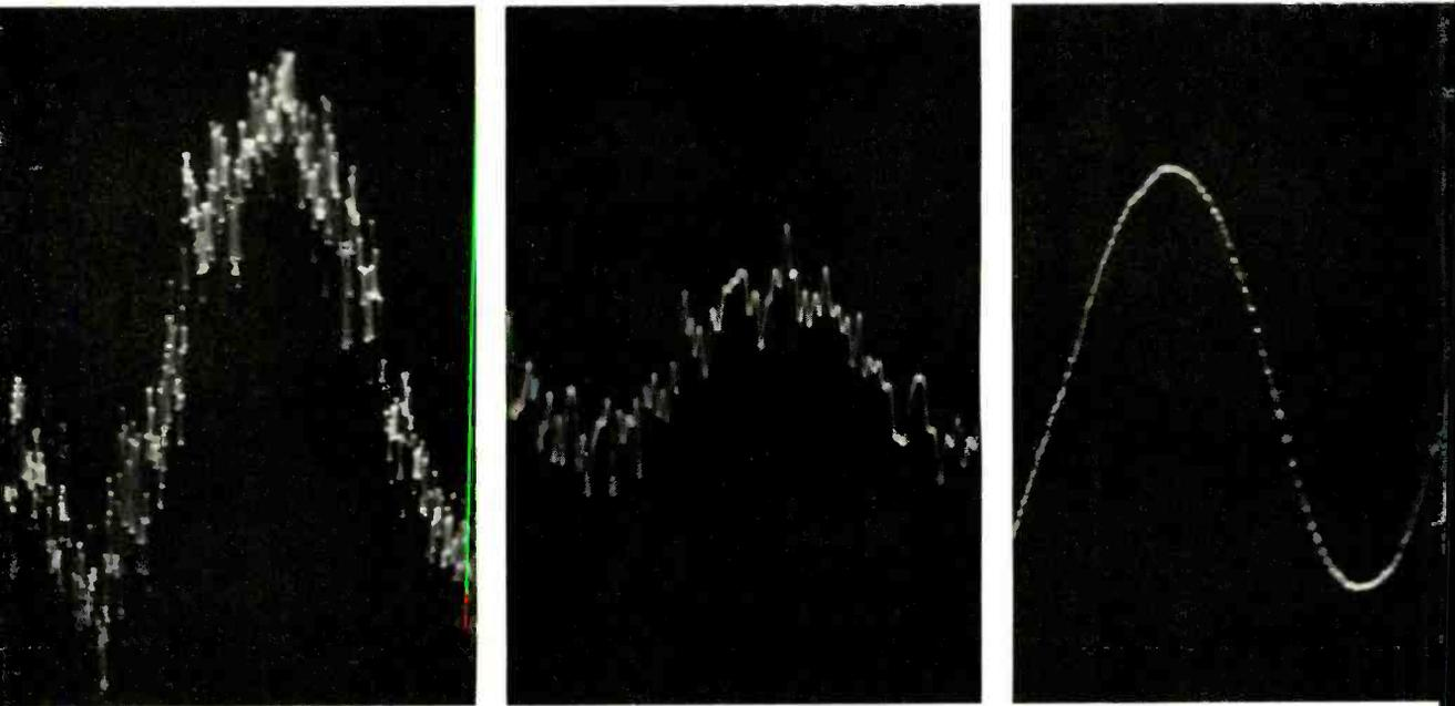
Fig. 6A—Oscillographic record of vibration testing machine of Figure 2; Fig. 6B—Record of machine of Figure 3; and Fig. 6C—Record of machine of Figure 4.
