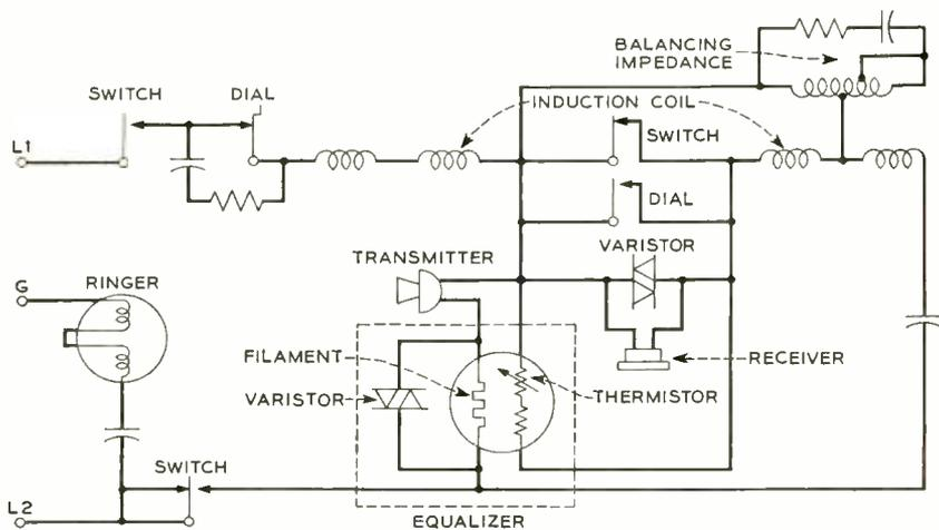
Fig. 2—Schematic of 500 type telephone set.
