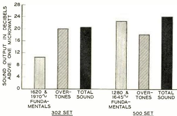
Fig. 6—Ringer sound output spectrum.
