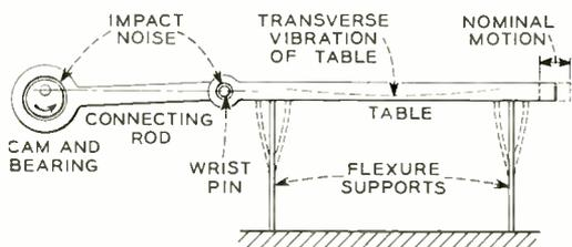
Fig. 3—Reciprocating vibration testing machine with table supported by flexure plates.
