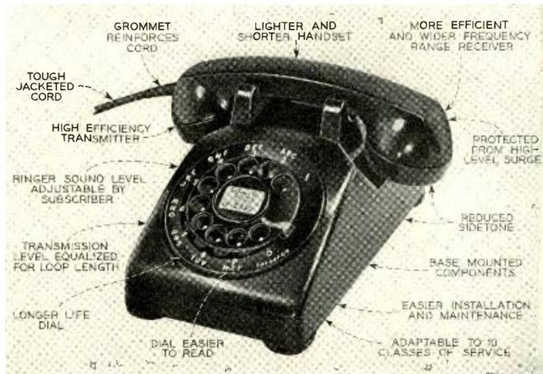
of the war that if a completely new set could be developed as an integrated unit, taking full advantage of improvements in structures, materials and design techniques, as related to service requirements, it would be possible to provide a new telephone set that would be still better than the 302. The development was started; the new set was ready for its first field trials by 1948, was placed in limited production in 1949, and production has been steadily increasing since then.
