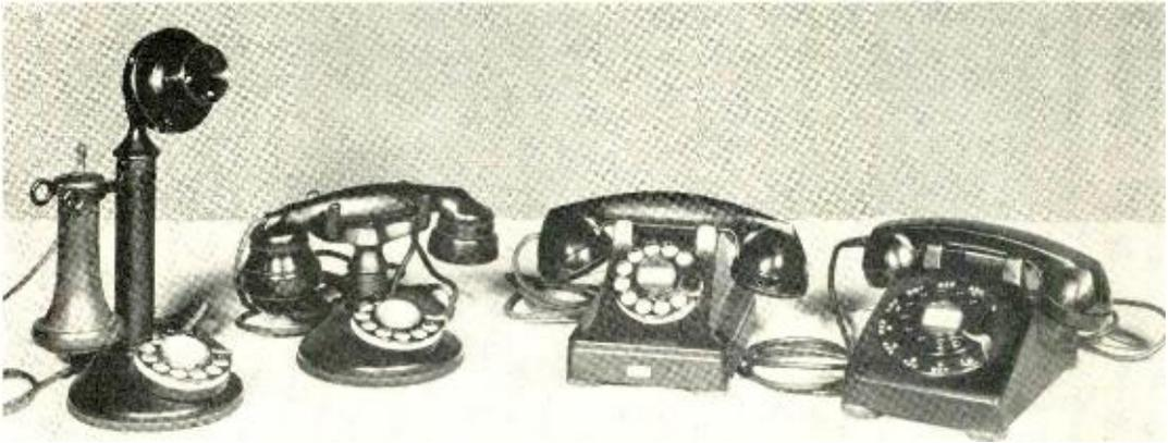
Fig. 1—Left to right, the deskstand of 1919, the handset of 1927, the combined set of 1937, and the 500-type set of 1950.
