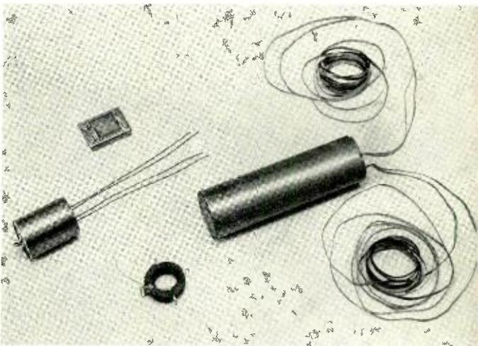
Fig. 1—Some of the components built for the submarine cable repeaters. The unit at the left contains three capacitances and a resistance hermetically sealed in an oil-filled container. The inductance below is combined with a resistance, and the mica capacitor contains two capacitances with a common terminal. The high voltage capacitor on the right has long tapes to avoid as many soldered connections as possible in the repeater.
