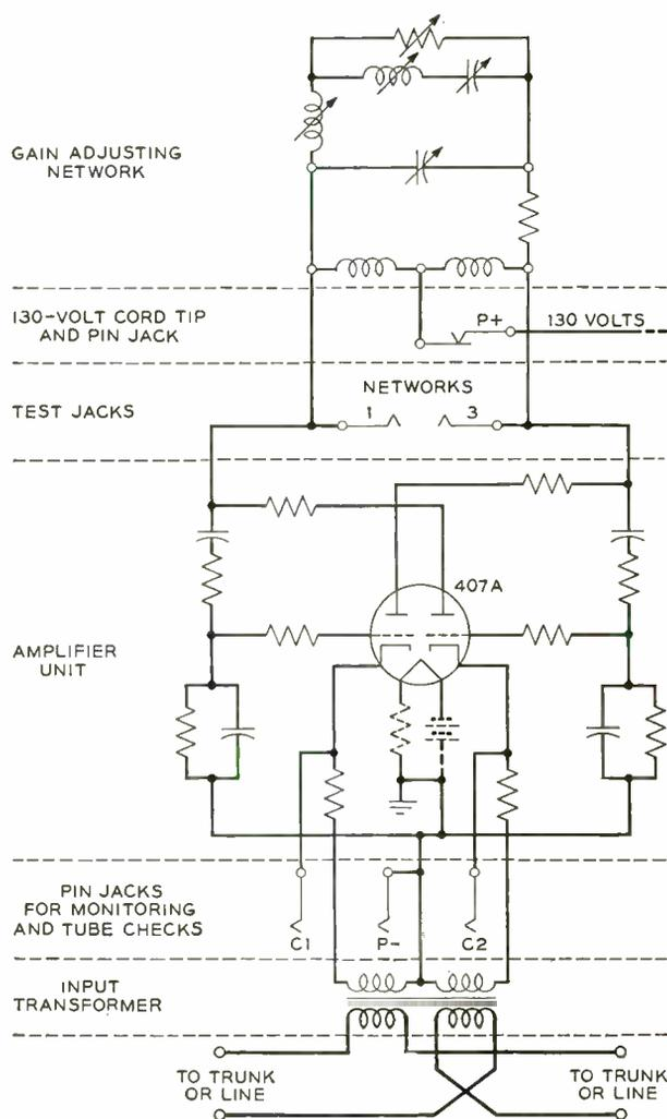
Fig. 4—Simplified schematic of the E1 circuit.
