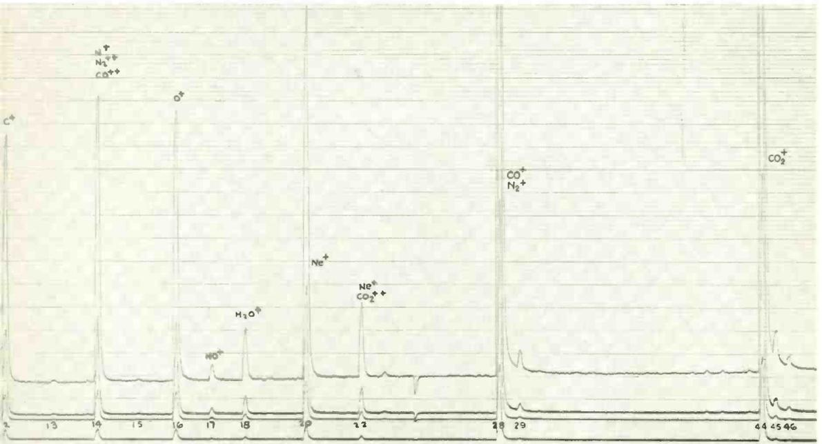
Fig. 3—Mass spectrum of a mixture that is composed of neon, carbon dioxide, carbon monoxide, nitrogen and water.
