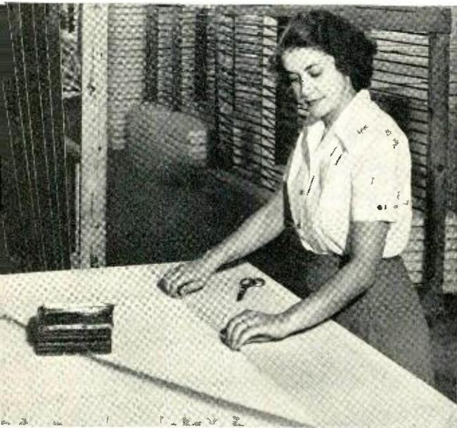
Fig. 3—Placing the aluminum strips in the slots.
