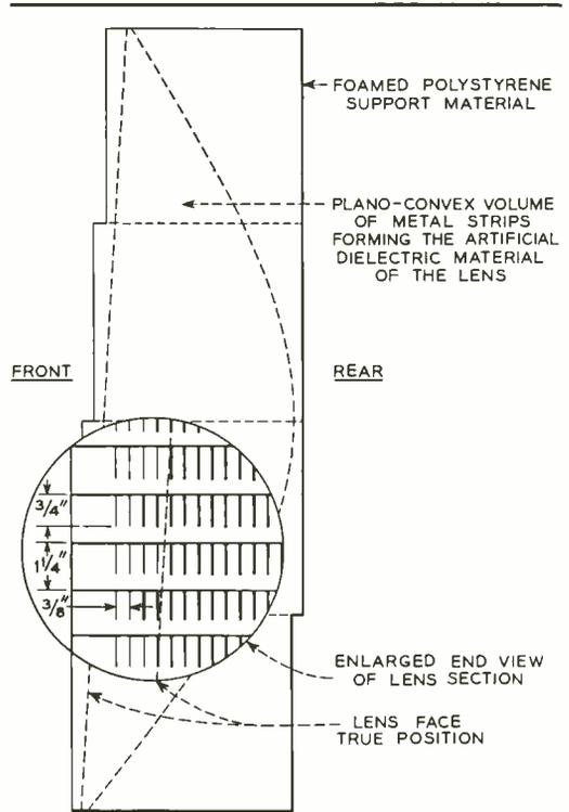
Fig. 4—Cross-section of lens with enlarged inset showing placing of strips to form front of lens. The slots into which the aluminum strips are placed are indicated by heavier lines.
