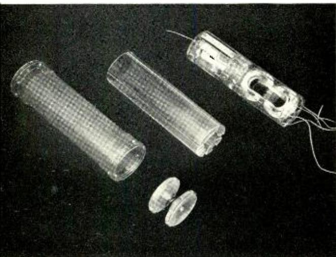
Fig. 2—Two small cores in a "figure-8" arrangement make possible a core of large cross sectional area for mounting in the restricted space.
