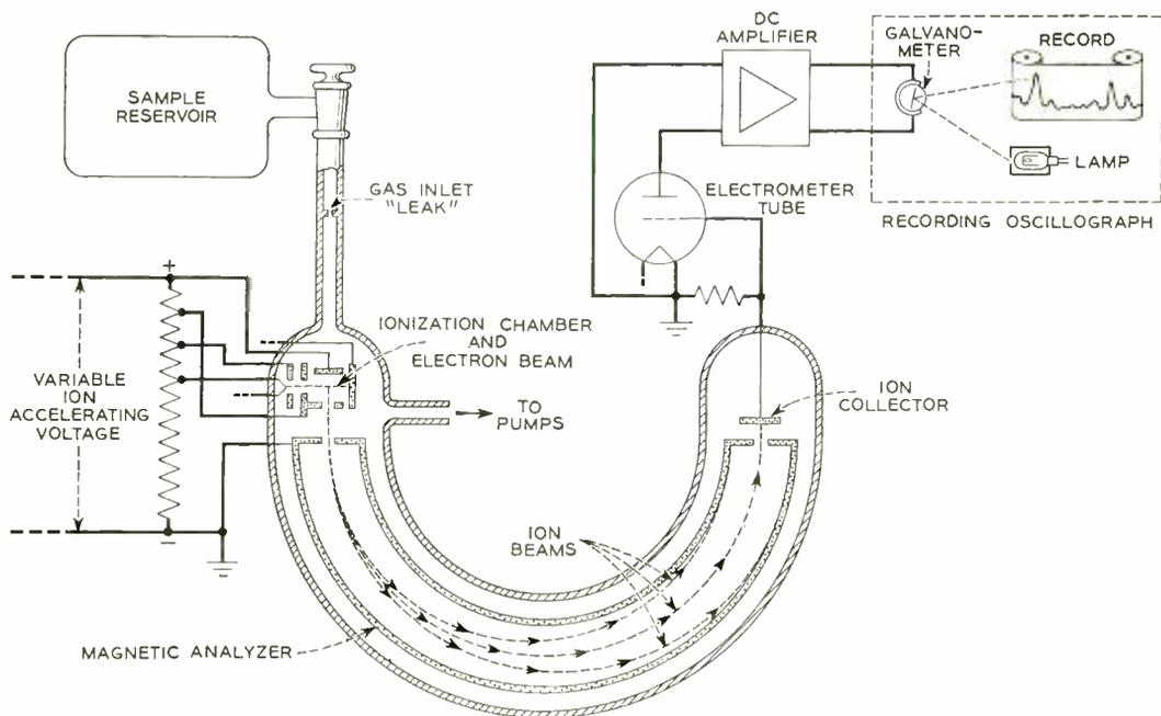
Fig. 2—Schematic diagram indicating the principles of operation of a mass spectrometer.
