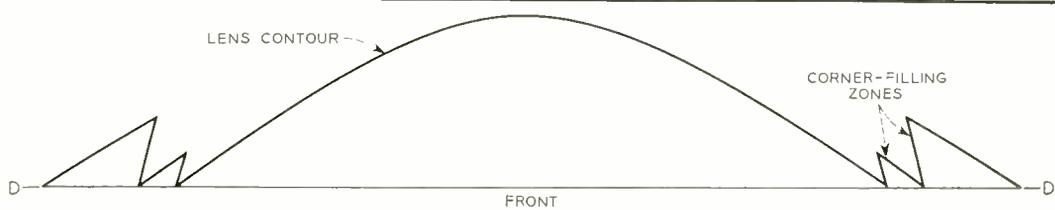
Fig. 5—Cross-section of lens along D-D (in upper left of Figure 1) showing corner lens sections.
