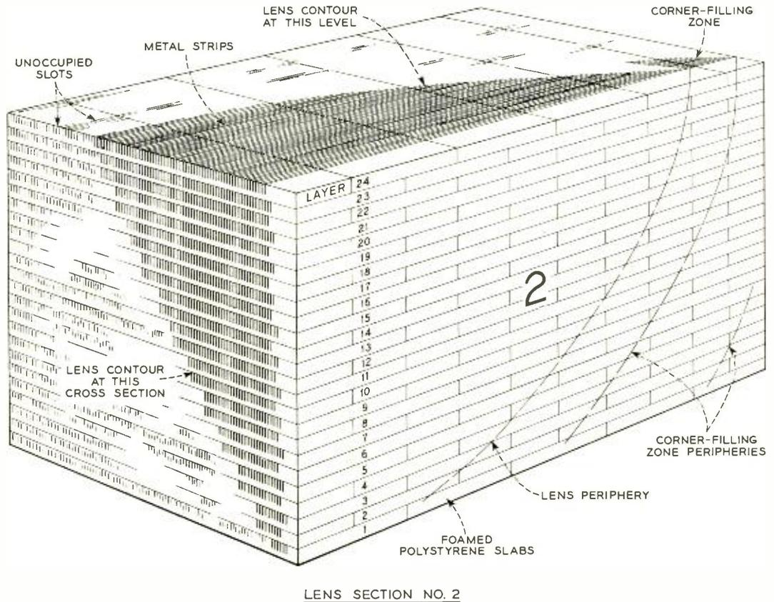
Fig. 1—Construction features of the delay lens antenna.
