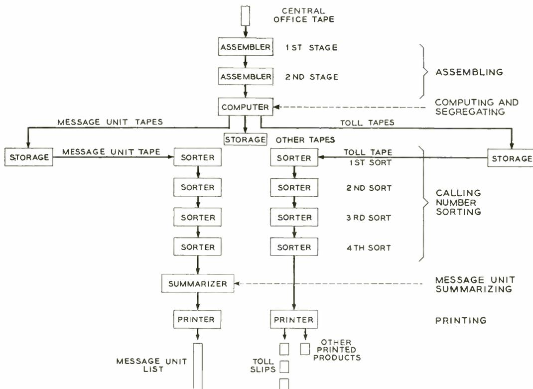
Fig. 5—Block diagram of an accounting center.
