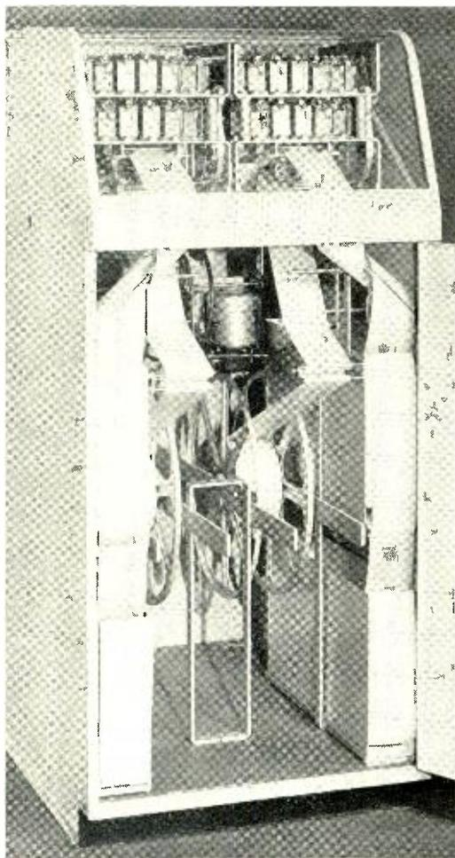
*Fig. 2—A perforator cabinet houses two perforators and their tape supplies. Below the perforators on either side are the paper input bins, and between them are the motor-driven reels for storing the output tape from the perforators.*
