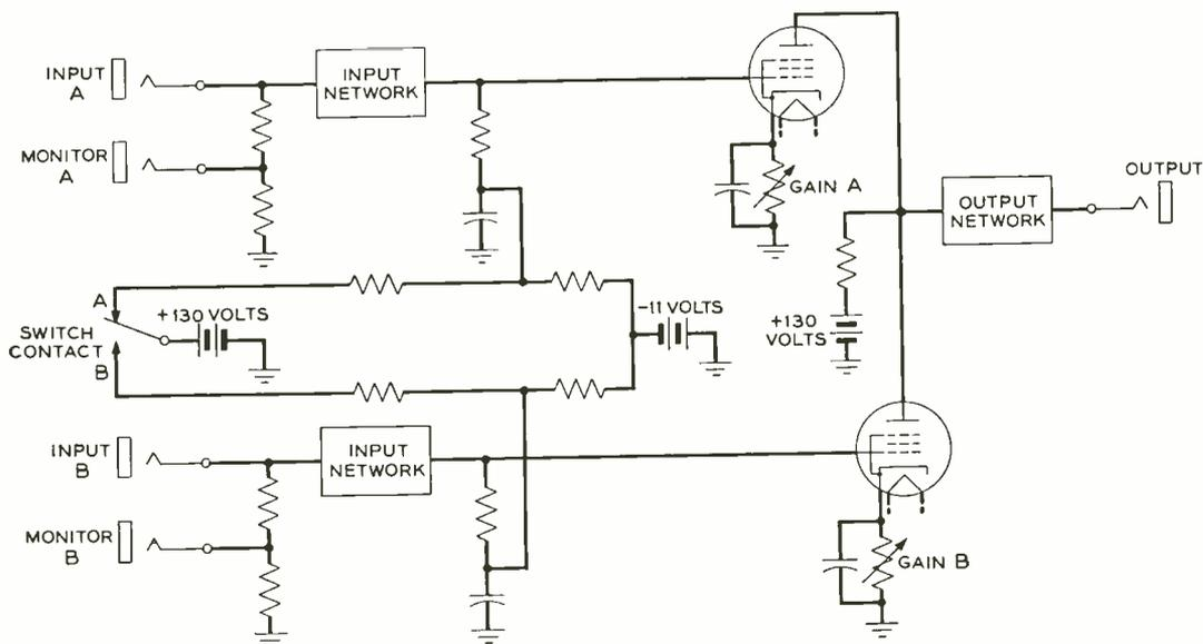
Fig. 1—Circuit of the switching amplifier.
