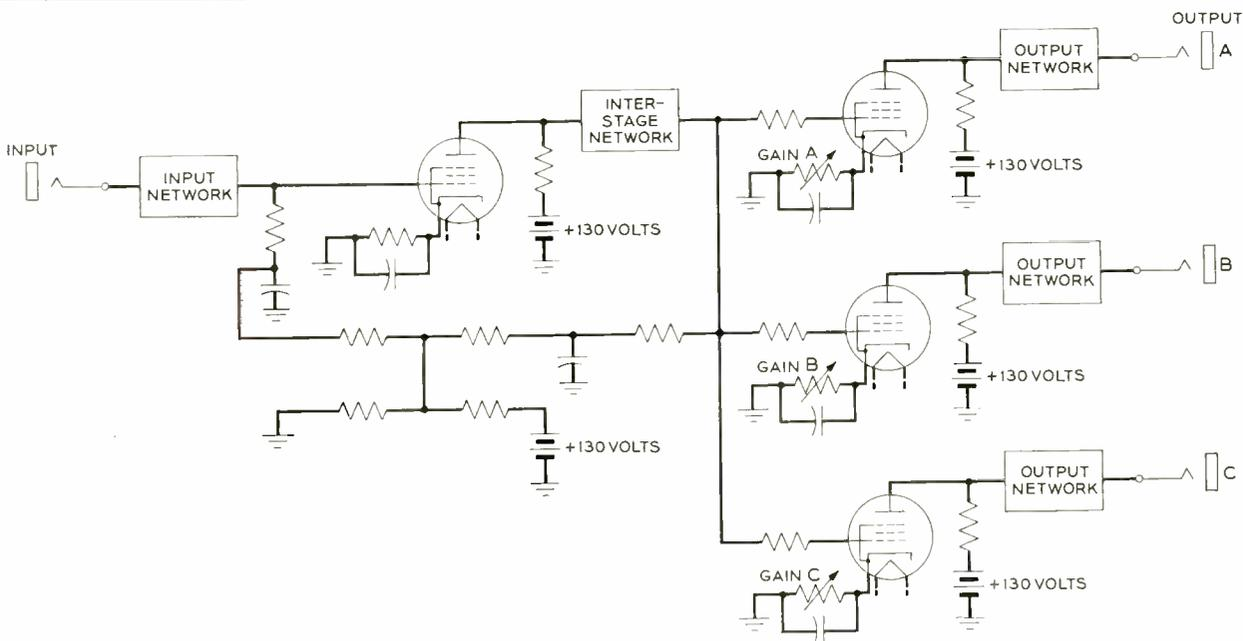
Fig. 2—Circuit of the distributing amplifier.
