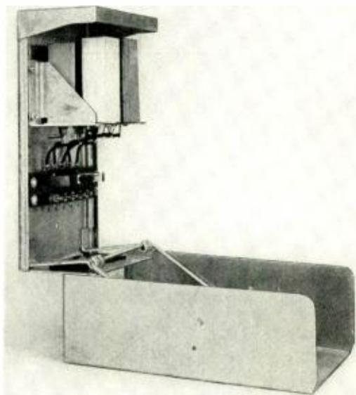
Fig. 2—The 108A protector in its mounting.
