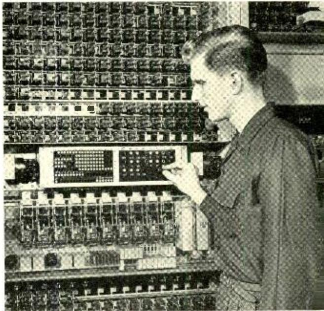
*A switching system is a physical structure of relays, tubes, wires, etc., combined with a wealth of stored information.*
