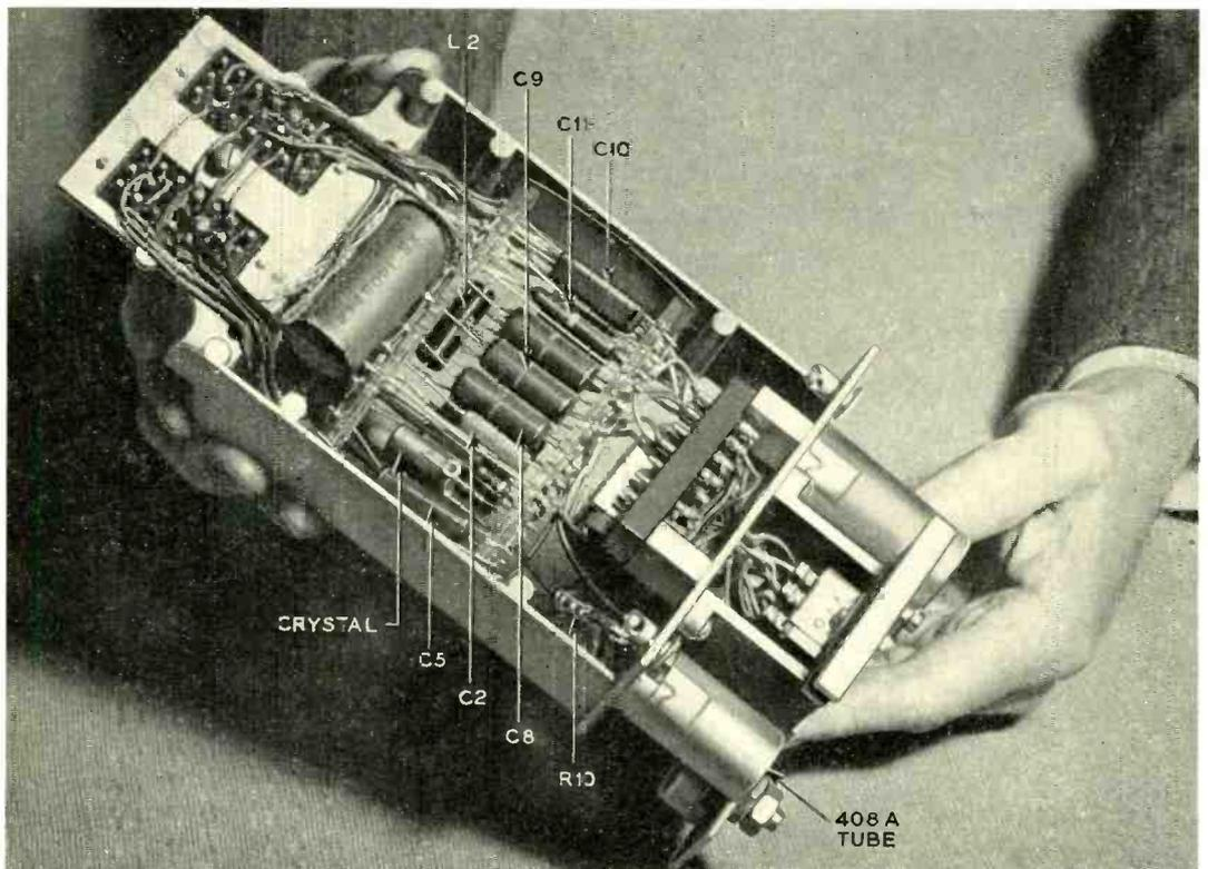
half-cycle change in frequency. Since the maximum possible change in capacitance due to the tolerance of  $c_3$  and  $c_5$  is approximately 5 mmf, a maximum change in frequency of 2.5 cycles is possible. Capacitor  $c_2$  is less critical than  $c_3$  and  $c_5$ ; it requires a 10 per cent change to produce a 0.3-cycle change in frequency.
