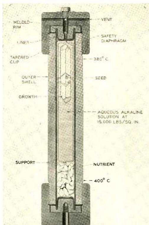
Fig. 4—Cross section of an autoclave used in successful crystal growing experiments.
