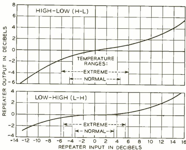
Fig. 2—Regulation characteristics for the high-low and low-high repeaters.
