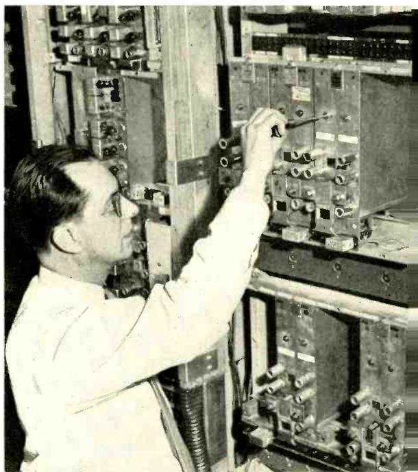
*Fig. 5—The author adjusts the repeater slope control in the laboratory test installation.*
