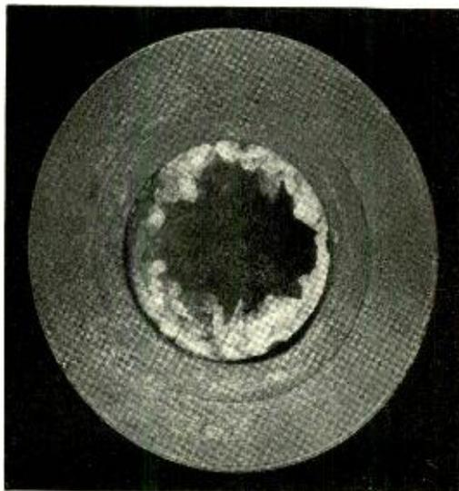
Fig. 3 — Section of an autoclave that leaked during a crystal growing run showing spurious quartz crystals adhering to inner walls.
