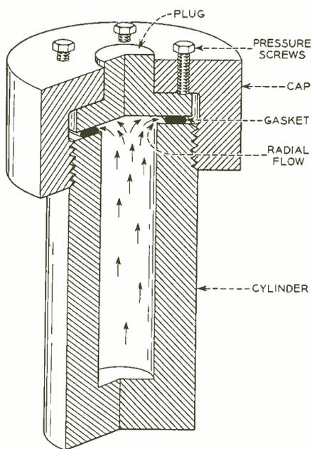
Fig. 2 — Cross section of an autoclave used in early attempts to grow quartz crystals.
