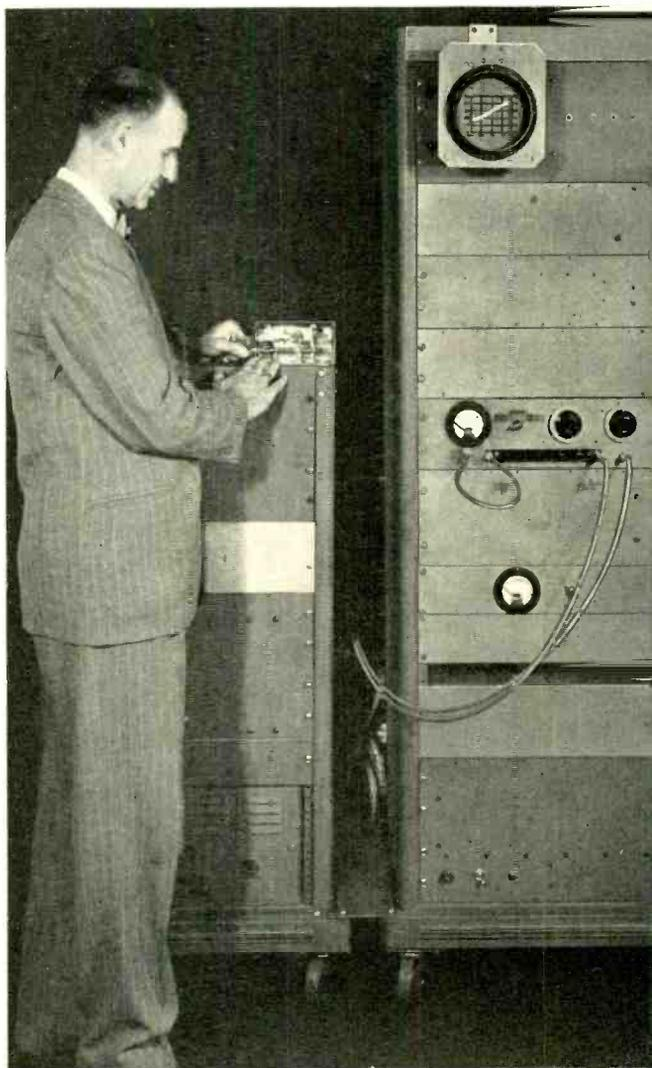
transmission systems. Envelope delay variations as small as one milli-microsecond can be measured over a range of several hundred milli-microseconds, and the operation is not affected by severe amplitude compression in any TD-2 transmission link. This apparatus is designed to measure the delay distortion characteristics in the 60- to 80-mc intermediate frequency band since that is common to all TD-2 channels while
