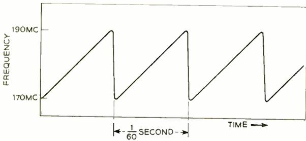
Fig. 4—Method of sweeping the 20-mc TD-2 intermediate frequency carrier band.
