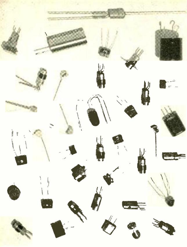
*Some of the nearly forty experimental types of transistors which have been developed at the Laboratories. In the illustration the transistors appear about half their actual size.*
