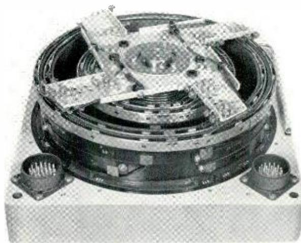
*Fig. 4—Drum type potentiometer with fourteen card brushes and drum assemblies.*
