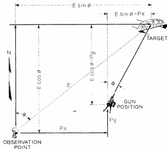
Fig. 9 — Trigonometric relationships between the observation point, gun position, and ground target.
