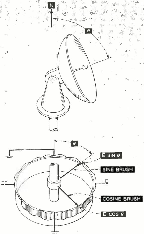
Fig. 10—Drawing illustrating the function of a potentiometer in relation to radar antenna.
