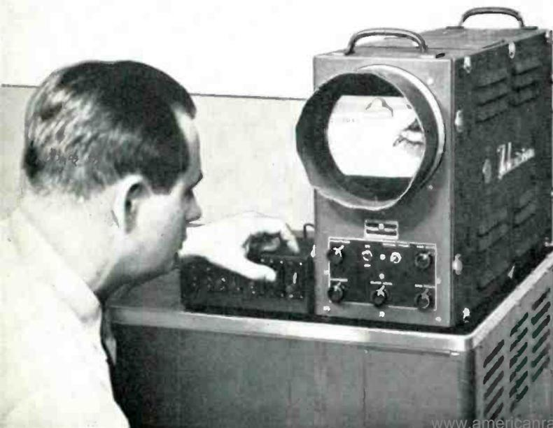
*A. P. Winnicky monitors scene picked up in another room by the television camera. By deflecting a key with his left hand, he can switch in a movie camera to make a permanent record of significant sequences.*
