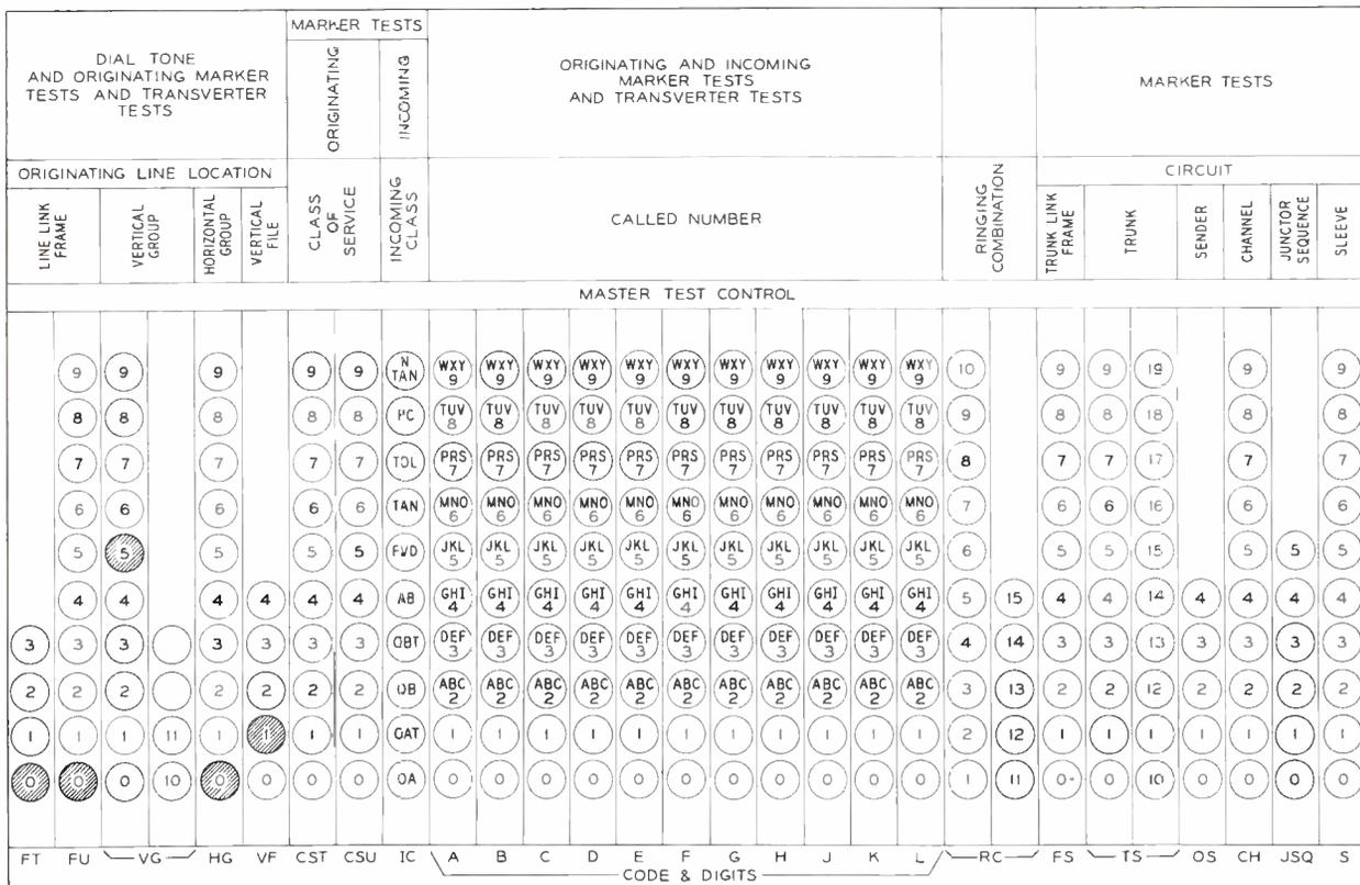
Fig. 4—Diagram of the master test frame keyboard. Shaded keys would be depressed if customer line appeared on line link frame 0, vertical group 5, horizontal group 0, and vertical file 1.
