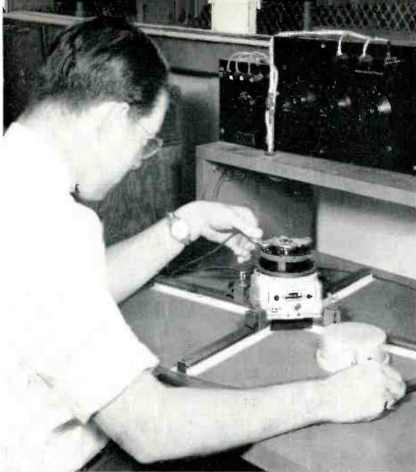
Fig. 5—R. G. Maines setting up potentiometer for calibrating. The potentiometer here is a small drum type with one card and drum assembly.
