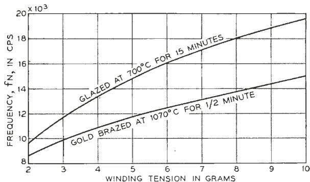
Fig. 4 — Natural frequency of vibration versus winding tension for gold brazed and glass glazed grids.
