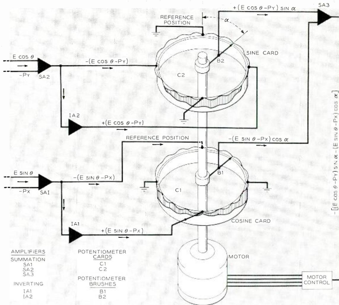
Fig. 11 — Potentiometers in an electrical circuit used to mark a shaft position and thus to aim a gun.
