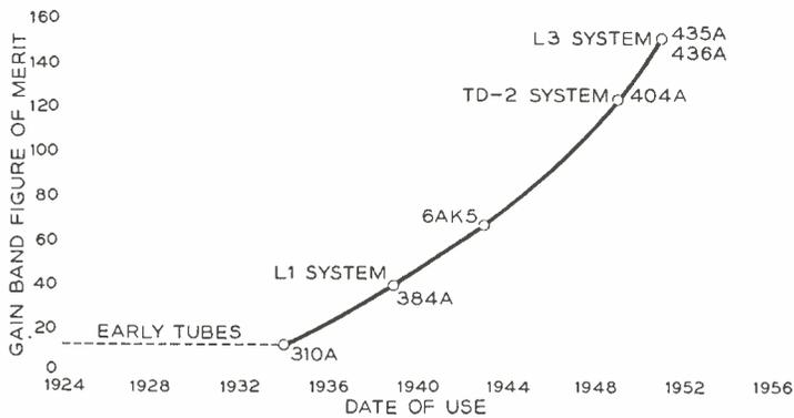
Fig. 1—Electron tube “gain-band figure of merit” versus date in which various tubes were used.
