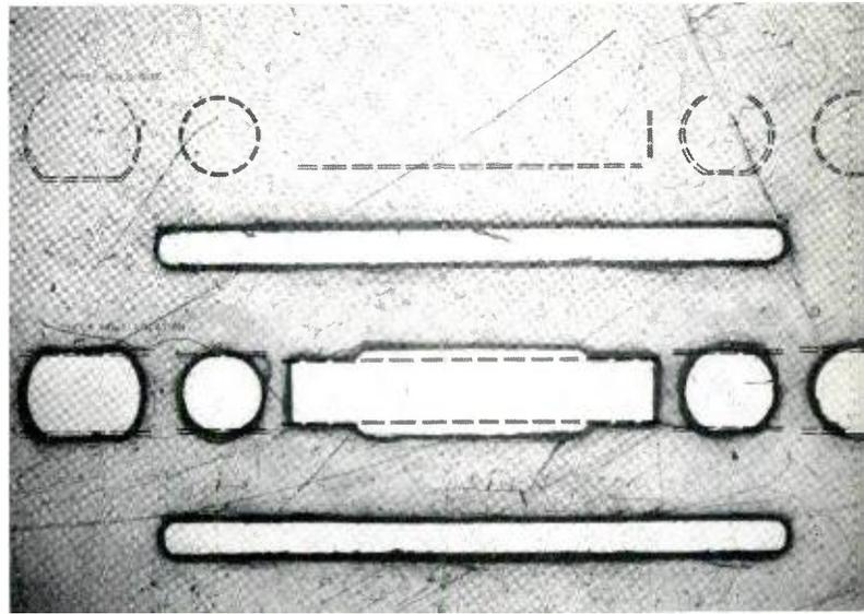
Fig. 6—Screen of optical projection apparatus showing a mica insulating disk in position.
