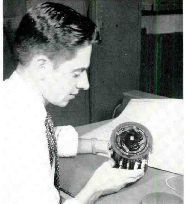
Fig. 6—F. L. Sulpy examining a molded potentiometer having two cards and four slip rings mounted in three concentric slots.
