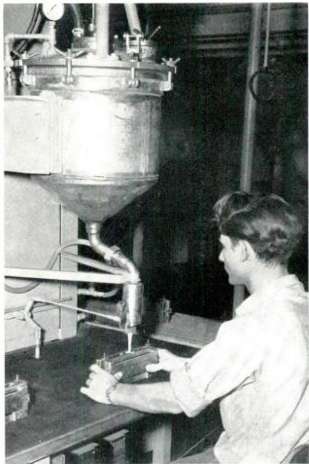
*Fig. 3 — After the solid sides of the mold have been clamped on, the casting compound is poured in this way. The operator is Donald F. Beck.*
