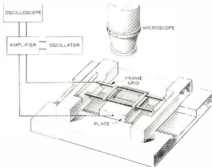
Fig. 5 — Schematic diagram of apparatus used to measure grid wire vibration frequencies.
