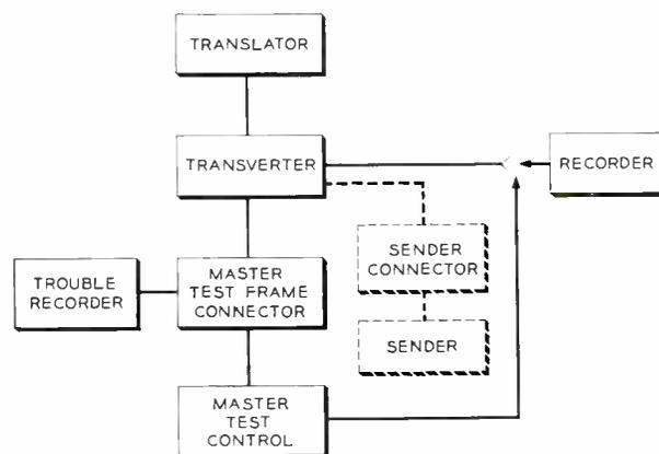
Fig. 3 — Block diagram illustrating the connections used on a transverter test. Broken lines represent circuits simulated by master test control circuit.
