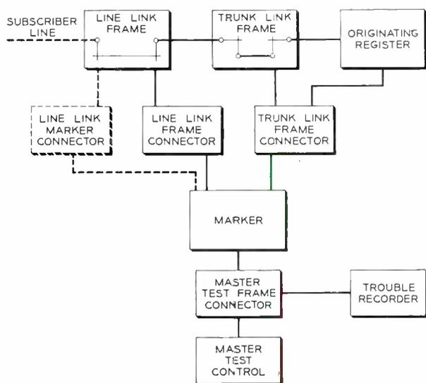
Fig. 1 — Block diagram illustrating the connections used on dial-tone marker tests. The broken lines represent circuits that are simulated by the master test control circuit.
