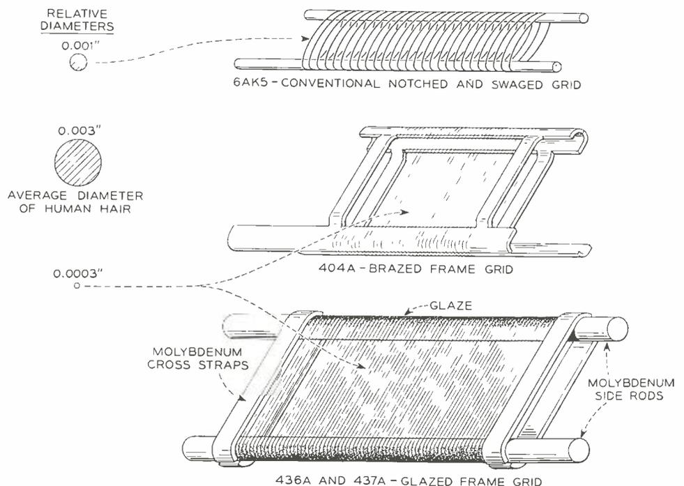
of this is that with the grid wires longer than before and closer to the cathode, greater precautions must be taken to prevent their sagging and shorting against the hot cathode.
