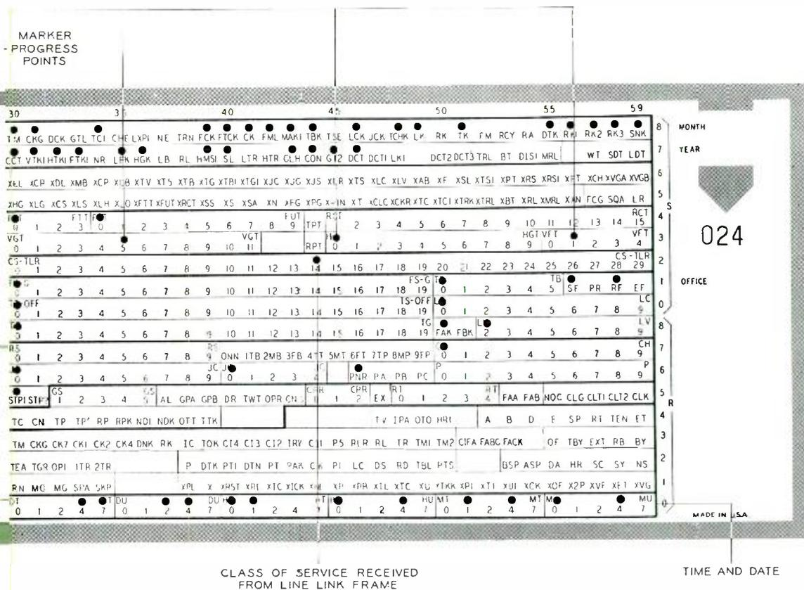
Fig. 5—Trouble recorder card produced as a result of a dial-tone marker test.
