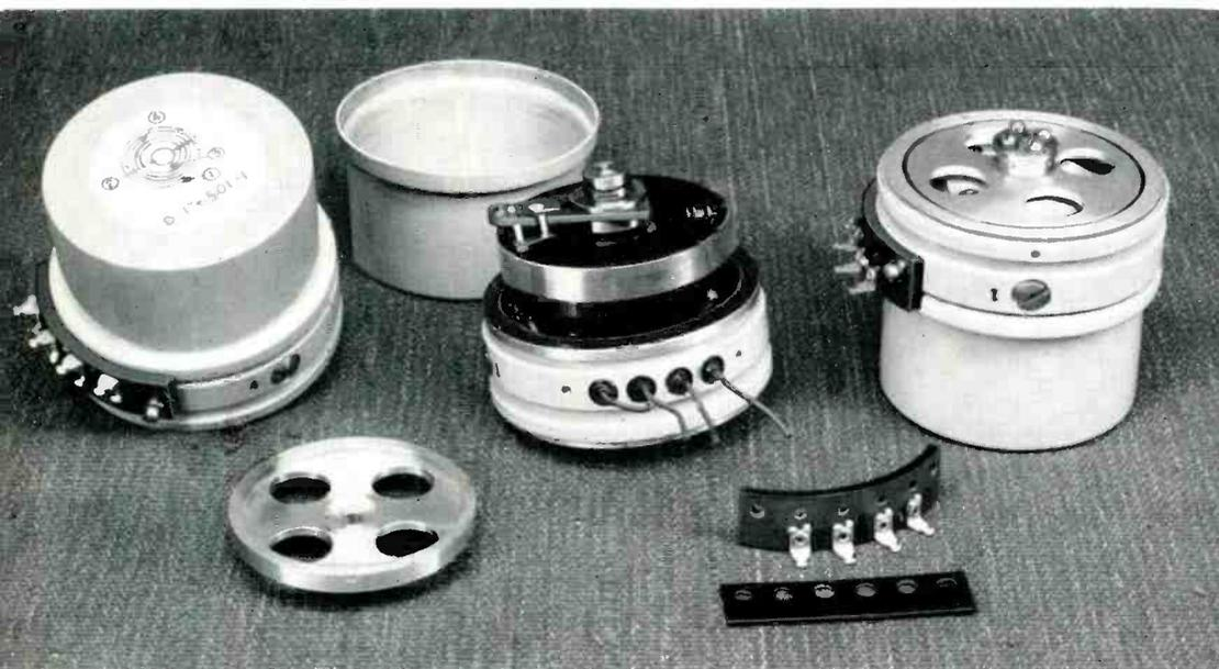
Fig. 7—A small potentiometer of the spiral type. A thirty-inch card is wound into a five and one-half turn spiral, two and one-half inches across.
