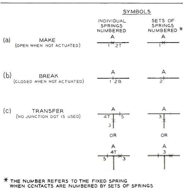
Fig. 3—Basic contact symbols used on detached contact schematics.
