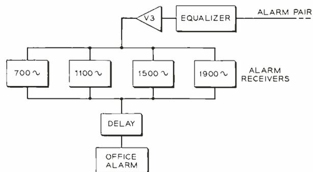
Fig. 4 — Block diagram illustrating a typical receiving station.
