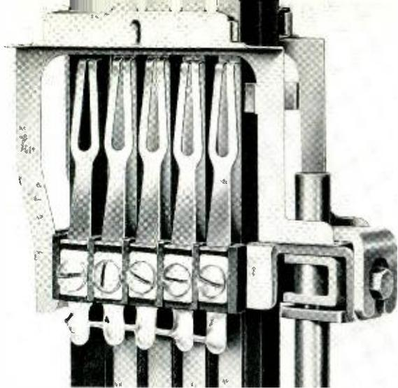
*Fig. 2 — Cleaning device attached to commutator brushes. This device eliminates much manual work and lost service time.*
