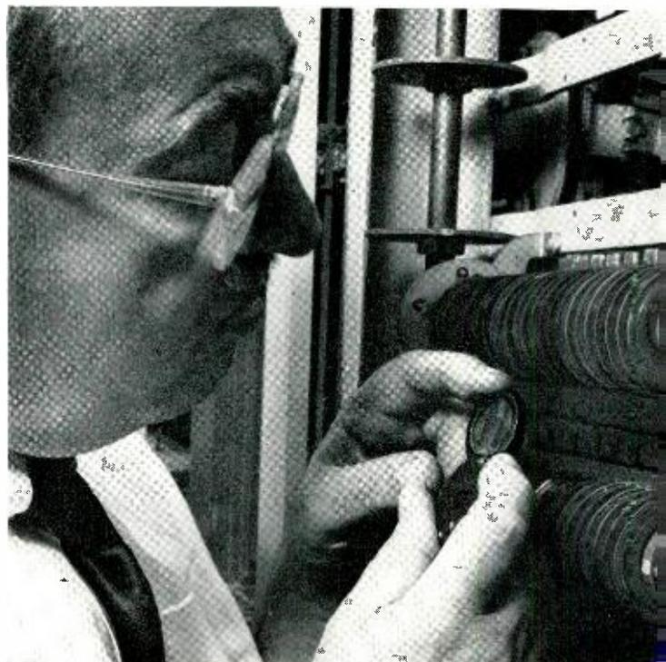
*Fig. 4 — W. W. Seibert examining silver-faced cams now incorporated in all panel system sequence switches.*
