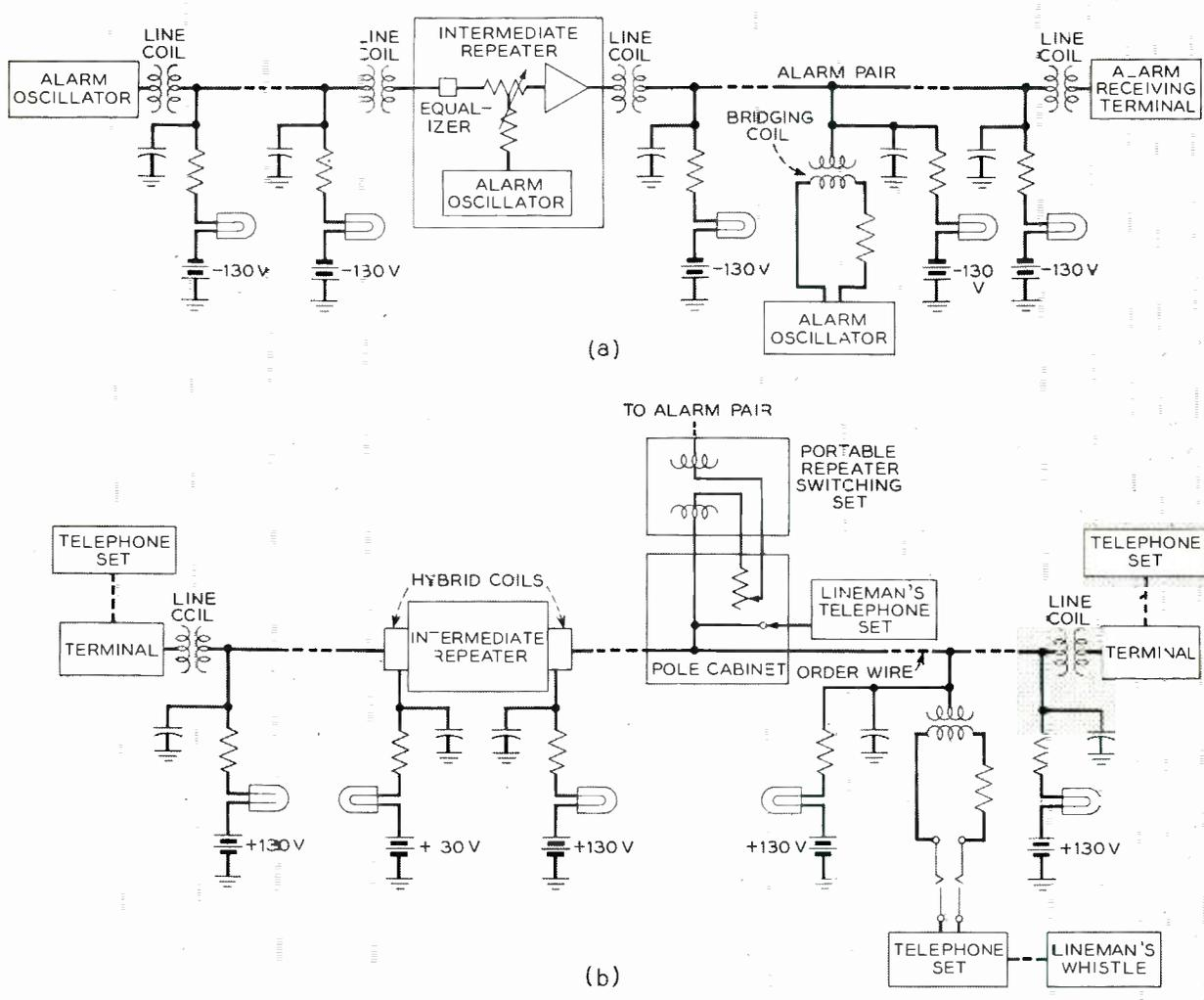
Fig. 1 — Block diagram, (a) alarm pair, (b) order wire pair.
