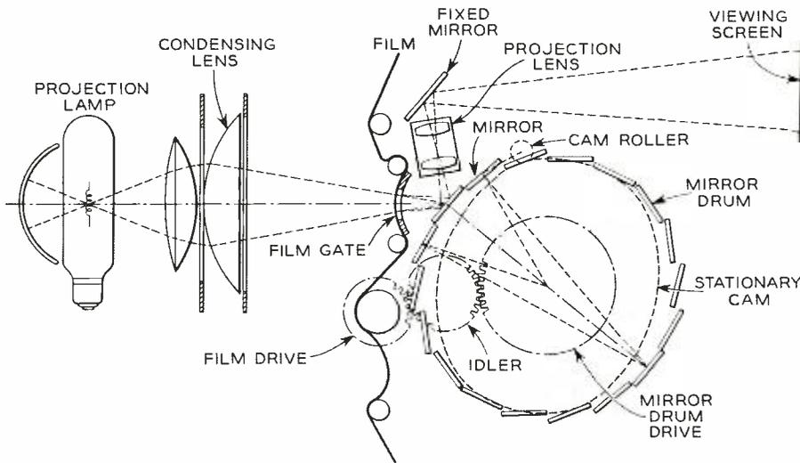
Fig. 2—The simple mirror-and-crank arrangement of Figure 1 has been replaced by several mirrors placed on a moving drum.
