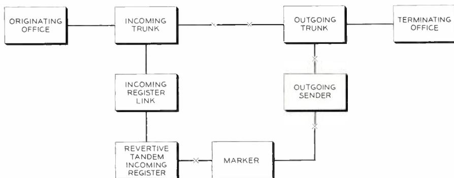
Fig. 2 — Block diagram illustrating the operation of the No. 5 crossbar tandem revertive-pulse incoming register.
