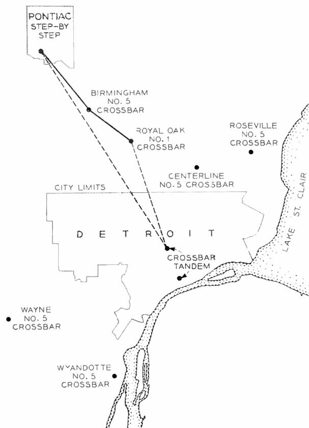
Fig. 1—Map illustrating use of the No. 5 crossbar tandem revertive-pulse incoming register in the Detroit, Michigan Area. Solid line shows the path of a call from Royal Oak to Pontiac if a No. 5 crossbar office is used and the dashed lines indicate the route that would be required if that office were not available.
