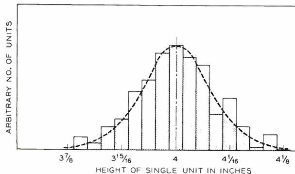
Fig. 1—Normal distribution of single units distributed about a four inch center.
