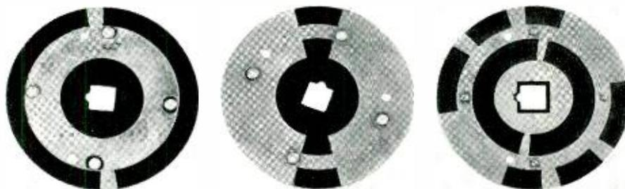
As shown in Figure 2, this device, which is easily attached to the commutator brush, employs two wiper pads. The pads are made of nylon pile fabric resembling velvet, which presses lightly against the contacting surfaces. The fabric may be either oil-impregnated or coated with a mild abrasive, depending upon the commutator molding material. When necessary, it is possible to replace the pad quickly and inexpensively. It is estimated that 1,500,000 of these devices will be employed.
