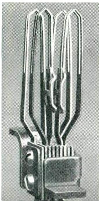
*Fig. 3 — Nest of eight sequence switch springs. The middle two springs in the front have been replaced.*
