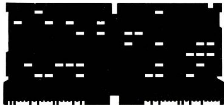
*Fig. 3—Shadowgraph end view of card stack with one card dropped, all channels blocked except those corresponding to enlarged holes.*
