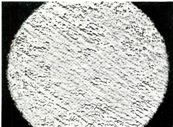
*Fig. 4 — Photomicrograph of compressed germanium, showing etch pits. Width of area shown about two-hundredth cm.*
