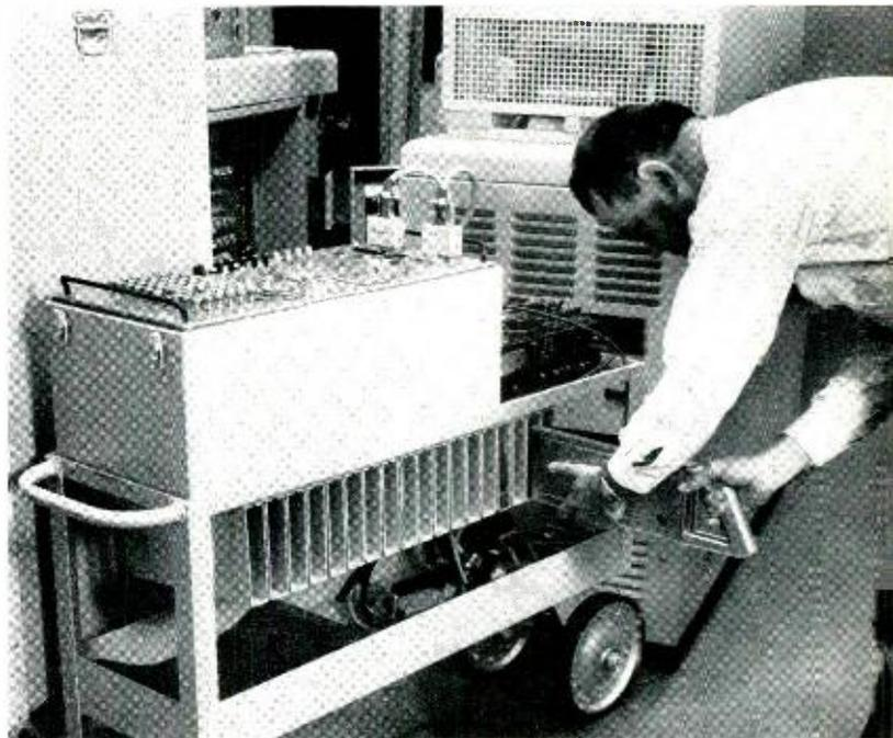
*Fig. 6—D. A. James using bulk removal tool to transfer cards in one bin of the translator to the "tea wagon" test set.*
