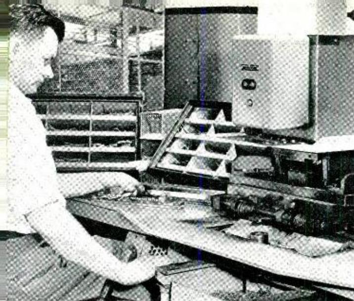
Fig. 3—Chester Grzyb makes Minaplas assemblies at Western Electric's Kearny Works. Ordinarily, two operators feed assemblies into the machine from alternate sides. The safety cover was removed to show details of the press.
