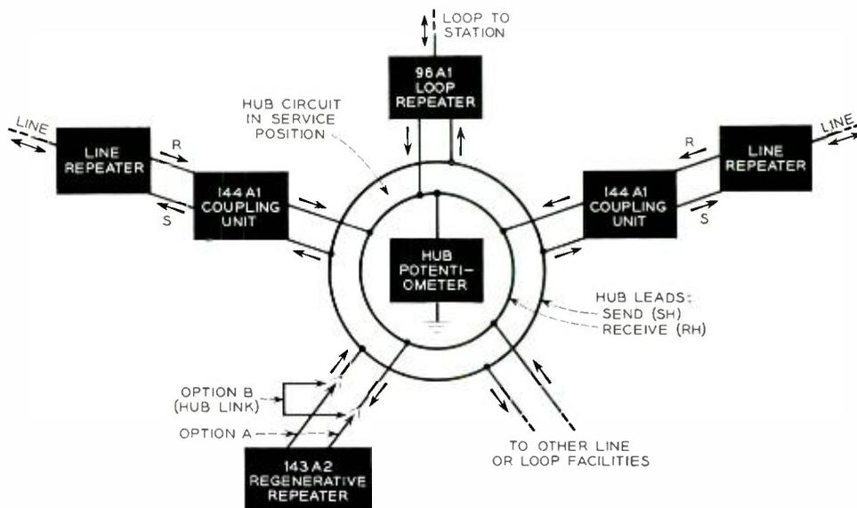
Fig. 4 A simple hub circuit of a station loop, two lines, and a regenerative repeater.
