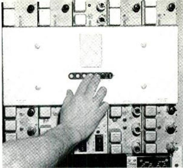
Fig. 3 — Two fingers are sufficient to operate the test keys and test the loop.
