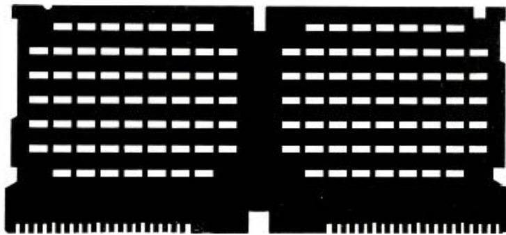
*Fig. 2—Shadowgraph end view of card stack, all cards in normal positions and all light-channels clear.*
