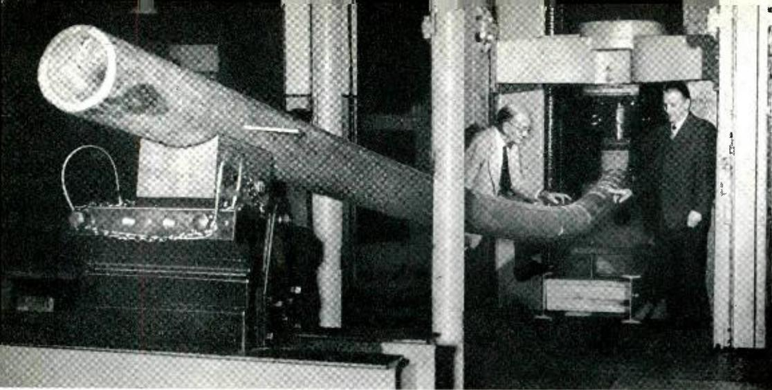
*Fig. 1 — Untreated western larch pole under test in the million-pound testing machine at the U. S. Government Forest Products Laboratory, Madison, Wisconsin. Pole is near ultimate load. Left to right: R. P. A. Johnson and L. J. Markwardt, Forest Products Laboratory.*
