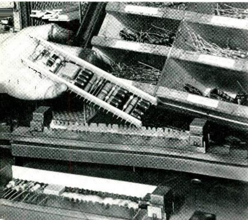
Figure 1 (left) shows fiber apparatus cards with riveted studs, commonly used to support apparatus and provide terminals for soldering. In contrast, the Minaplas counterpart has double the number of components, each providing its own soldering lugs. The cost of a Minaplas assembly is half that of its predecessor, partly because of material and volume reduction, but mainly because of its adaptability to machine assembly.
