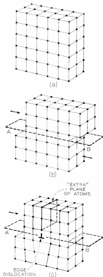
*Fig. 1 — Representation of crystal lattices illustrating formation of edge dislocation by partial slip of plane of atoms.*
