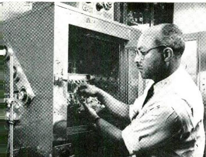
Fig. 2—Apparatus for volumetric measurement of absorbed oxygen. W. L. Hawkins adjusts some samples being measured as he checks the level of the gas in the burettes.
