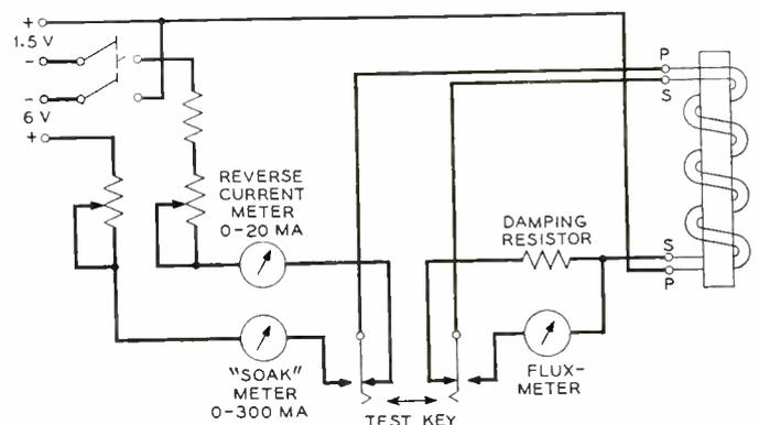
*Fig. 1 — Circuit of the test set. The test key is operated to the left, to normal, and then to the right for the indication on the fluxmeter.*
