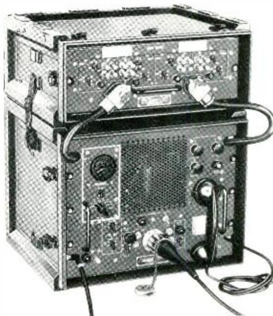
*Fig. 1 — Four-channel modem unit mounted above its associated amplifier-power supply.*
