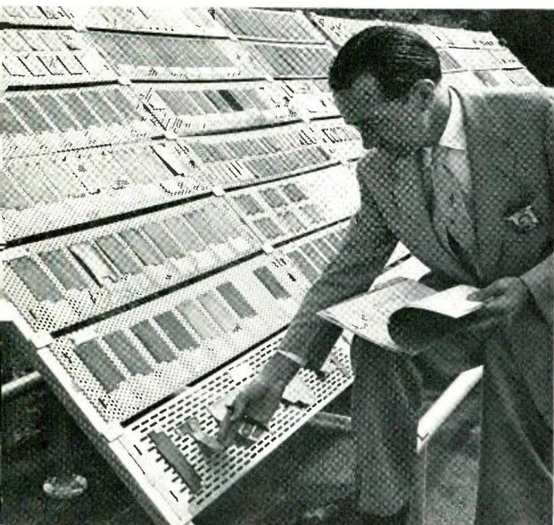
*Fig. 1—V. T. Wallder at an outdoor exposure plot examines part of the original sample of black polyethylene that has been exposed since 1941.*
