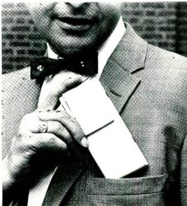
*Small transistorized receiver responds to individual customer's radio signal, informing him that he has a telephone call. Service is still experimental.*
