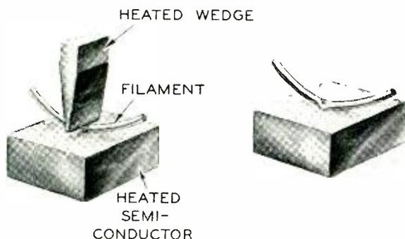
*The thermo-compression bonding technique: 5,000 to 10,000 psi pressure on wedge at temperature of 200-300°C produces mechanically strong bond.*
