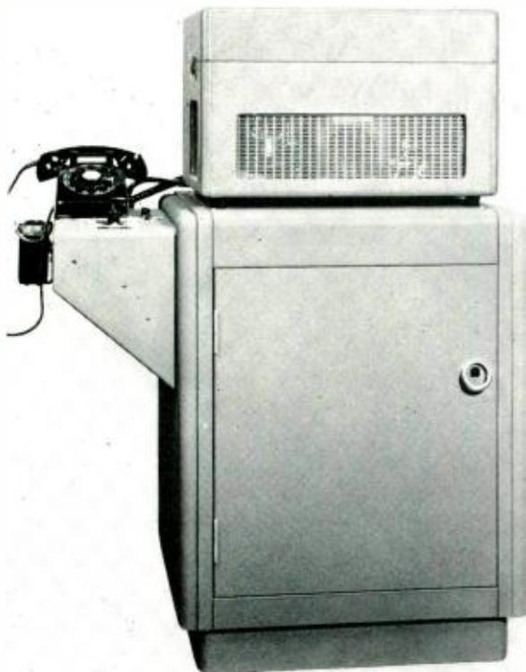
*Fig. 3—Later version of the Recorded Carrier System equipment with modified control panel.*
