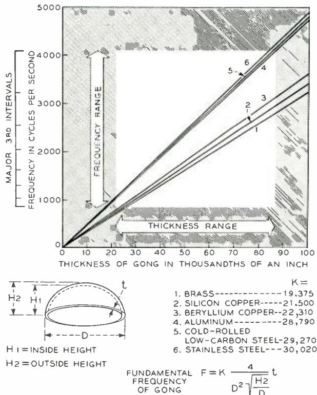
Fig. 2—Graphs of six possible metals for distinctive gongs, relating thickness to fundamental frequency according to the design formula.
