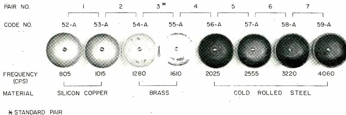
Fig. 3—The eight distinctive gongs grouped into seven ringer pairs. Brass gongs are in 500 set ringer.
