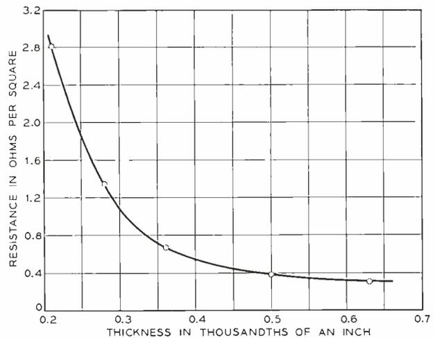
Fig. 4—Resistance versus thickness of film for 30 per cent by volume of silver pigment.
