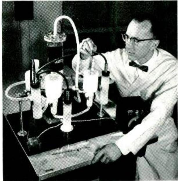
A highly effective system for removing surface contamination from semiconductor components has been adapted from electron-tube techniques by Miles V. Sullivan of the Laboratories. This is a continuous water-washing system that completely removes all water-soluble materials which remain after etching, and that monitors the effectiveness of the washing procedure.
