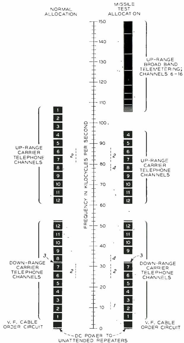
Fig. 1 — Frequency allocations for various channels in the Air Force cable. 1. Telemetering channel 12 for down-range transmission. 2. Program band for either up- or down-range transmission. 3. Synchronizing frequency, 32 kc. 4. Channel 8 down range transmits range timing pulses with the normal 80-kc carrier shifted to 72 kc. Up-range channel is used for checking purposes.
