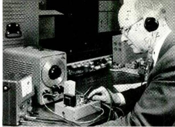
Fig. 5 — W. R. Young of the Laboratories with special aircraft-type detector used in the simulation tests of air-ground communication system.
