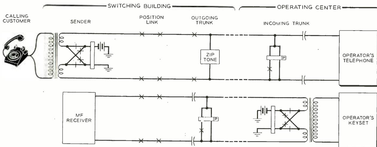
Fig. 2—Signaling paths used for C.A.M.A. operation in a position remote from the switching equipment.
