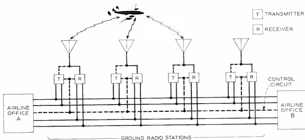
Fig. 1 — Air-ground communication circuit using telephone lines to connect radio equipment located at stations along an airway.
