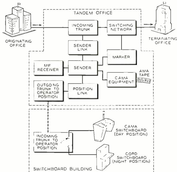
Fig. 1—Equipment arrangement for remote C.A.M.A. operator positions.
