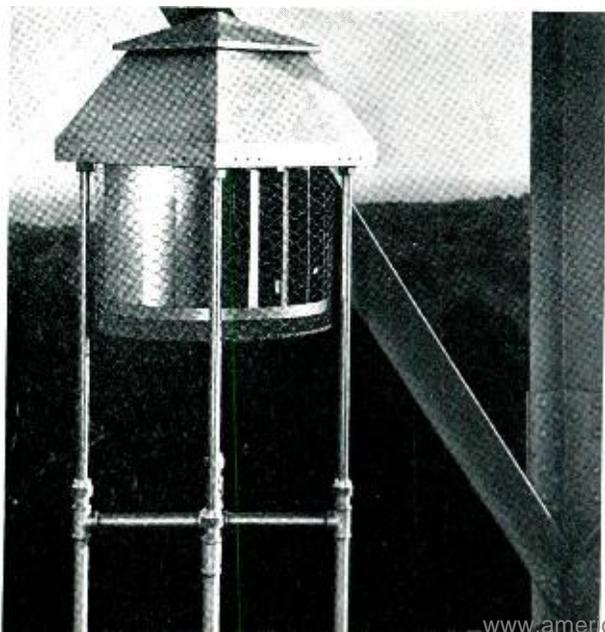
The model windmill has an effective cross section of about one square foot and, with an average wind speed of 11 miles per hour, produces an average power of one watt. Since the power in the wind varies as the cube of the velocity, the output into the battery is considerable at high wind speeds. At the Chester Outside Plant Laboratory, where the new windmill is now operating experimentally, the average wind speed is about 11 miles per hour.
