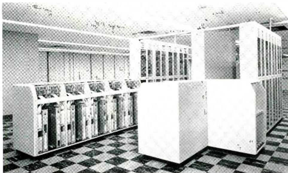
*Fig. 1—The assembler-computer replaces assemblers and computers in older installations of automatic message accounting equipment.*
