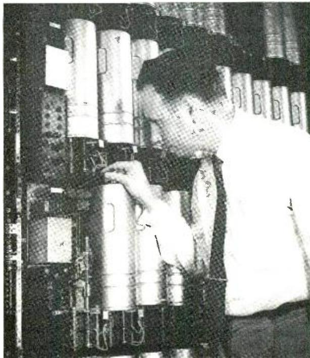
Fig. 4—*I. M. Fine adjusts relay contact spacing in connector for line-insulation test circuit.*
