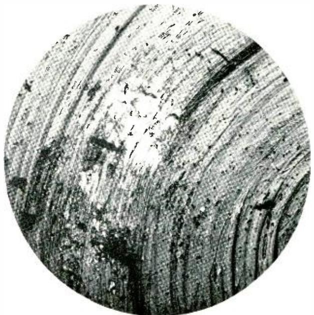
Fig. 2—Photomicrograph by F. G. Foster showing black-dyed oxide ripped and abraded from aluminum surface (magnification 100 diameters).
