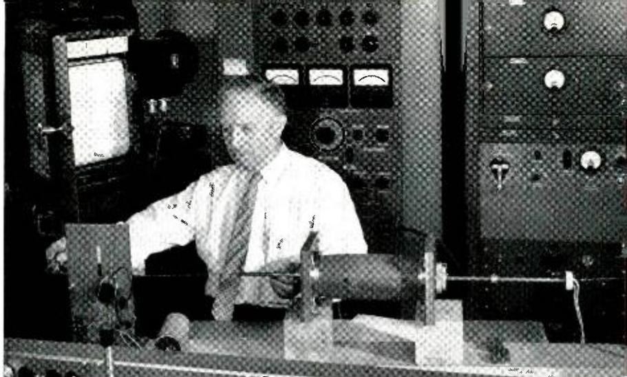
**The traveling-wave tube, now finding many uses in the Bell System, has an important element located outside the glass envelope. Though mechanically simple, this exterior structure — the beam-focusing magnet — must be precisely designed and its field accurately aligned with the tube axis to insure satisfactory operating efficiency and long life in microwave amplifiers.**
