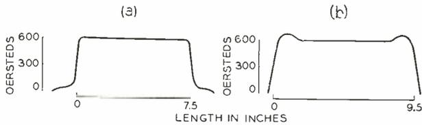
Fig. 2—Beam-focusing magnet developed for power TWT in TH system (a), and (b) magnet structure for TWT in a military application. Air-gap curves for respective magnets are shown below.
