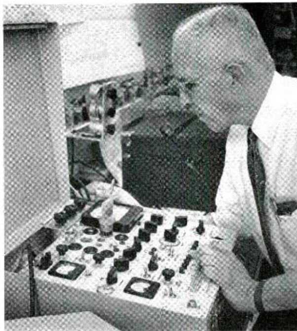
**Many key parts of various Bell System communications networks depend on the reliable operation of a wide variety of electron tubes. To help prevent failures and any resulting interruption in service, these tubes are tested from time to time and weak units are replaced. Portable, general-purpose tube testers are often used for performing a variety of these tests.**
