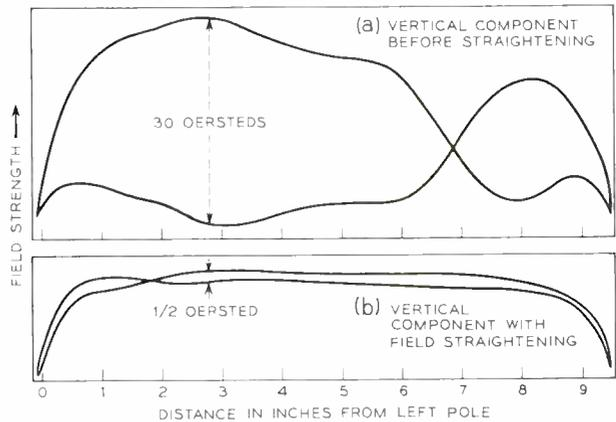
Fig. 5—*Transverse-field patterns of (top) field before straightening, and (bottom) field after installation of field-straightener in the air-gap.*
