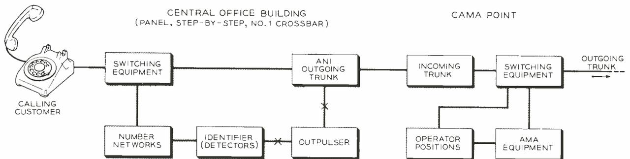
Fig. 2—Diagram of ANI equipment in central office and connecting equipment at CAMA point.
