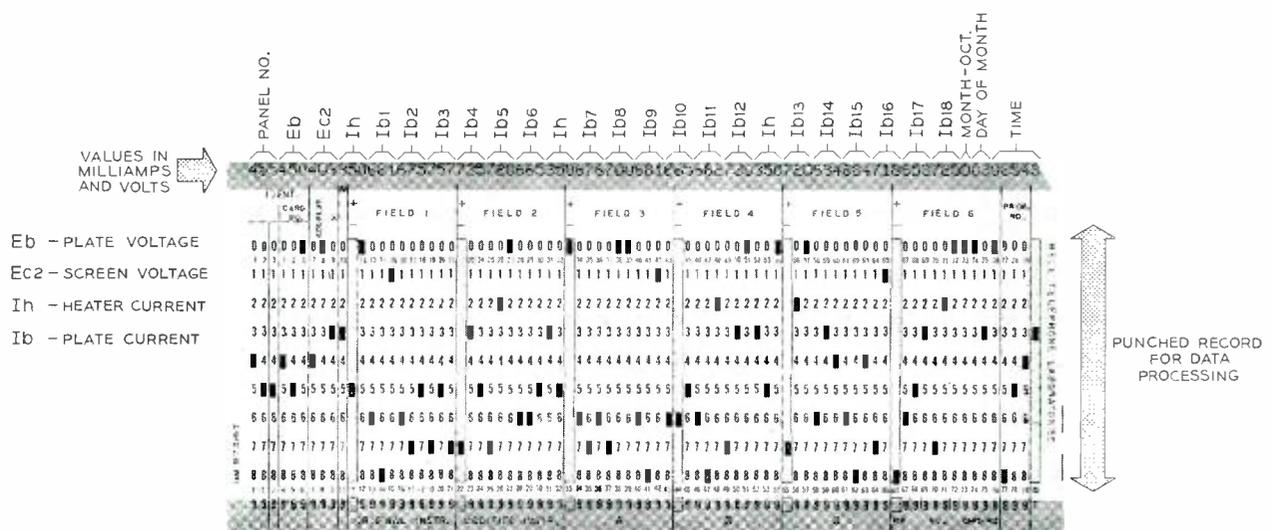
Fig. 2—Business machine card showing printed and punched data and designations of columns.
