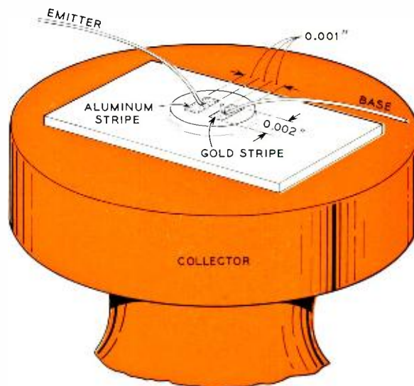
Details of structure seen in cover photograph: germanium crystal has raised area or "mesa", on which are evaporated two tiny metal stripes. Wires from headers are bonded to these stripes to form the transistor's base and emitter connections.
