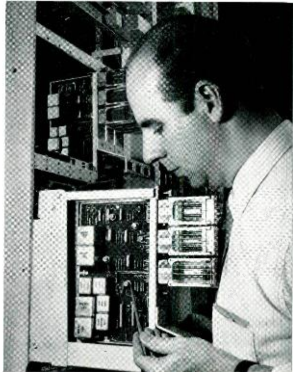
E. M. Hoffman of Special Developments Department inspecting a single-frequency signaling unit. Transistors allow small size and low power drain.
