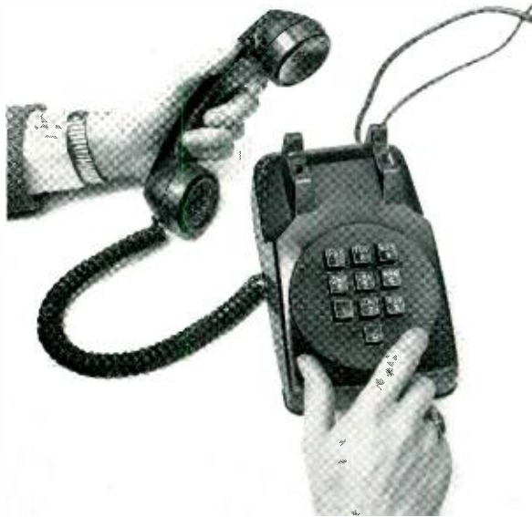
Experimental electronic telephone instrument: this trial model contains transistor circuits for both speech transmission and tone ringing, and uses pushbuttons instead of the usual dial. Pushbuttons send multifrequency tones in place of the usual direct-current pulses to the central office.
