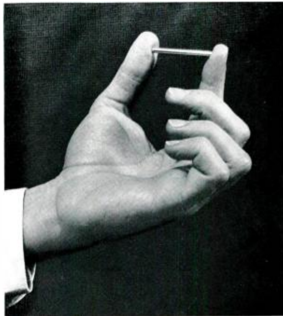
Despite its extremely small size, this amplifier built for research study contains a broadband transistor and fourteen other circuit elements.
