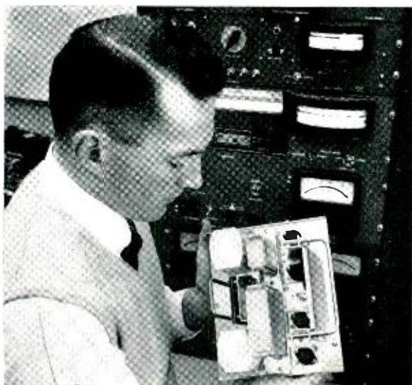
C. W. Green holding a transistorized power supply developed for a military system. The four transistors can be seen along the right side of the unit.
