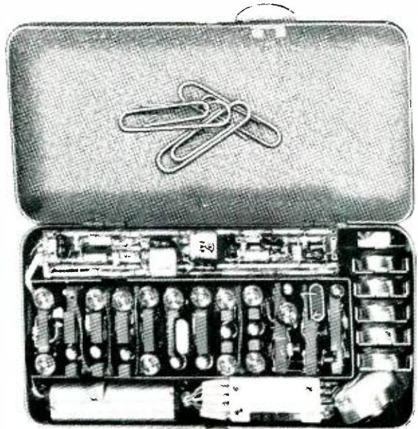
Another example of miniaturization: radio signaling receiver includes seventeen transistors and has high performance with long battery life.
