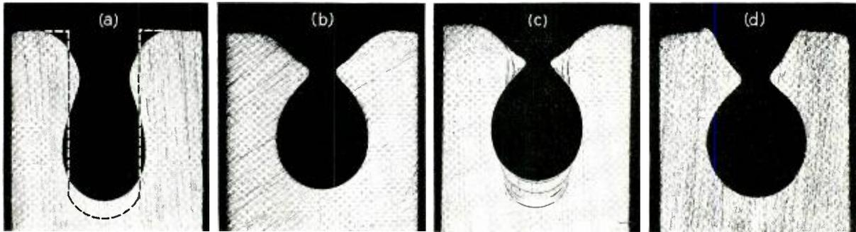
*This series of photomicrographs (about 45 diameters) shows effect of sputtering on cathode structure. A cathode with cylindrical hollow (a)*
