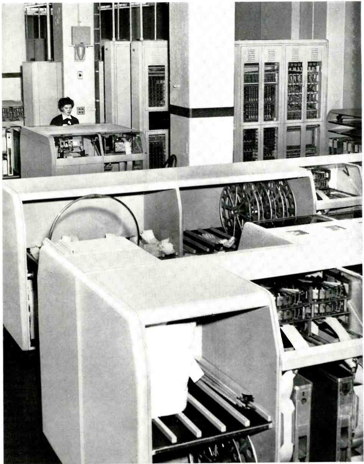
*Automatic message accounting center similar to the one installed at Philadelphia in 1948. Guard in left foreground locates splicing table now partially replaced by portable splicing dolly.*
