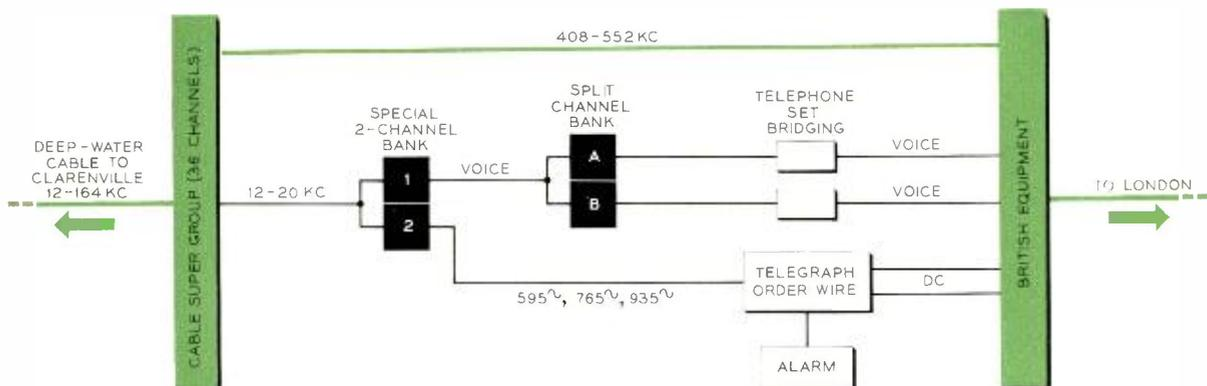
Block diagram of terminal equipment at Oban, Scotland. This equipment is the actual connect-
