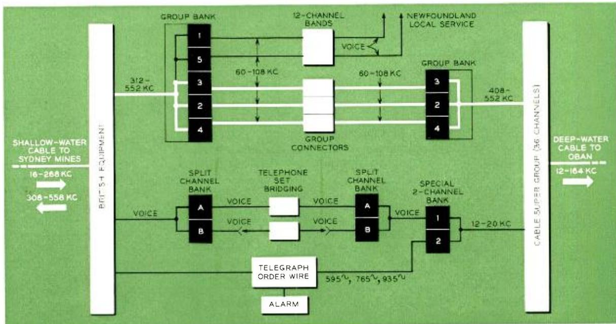
Block diagram of cable terminal equipment at Clarenville, Newfoundland; this arrangement con-
