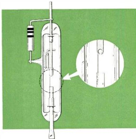
*"Production" model of talking-path diode, left, and a portion of tube cut away to show the cathode construction. Tube is about 1½ inches long. Resistor and deposit on inside of tube ("getter flash") provide small photoelectric priming current to initiate rapid breakdown in main gap.*
