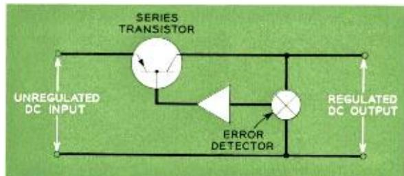
*Circuit diagram of basic series-transistor regulator. Detector and amplifier details are omitted.*
