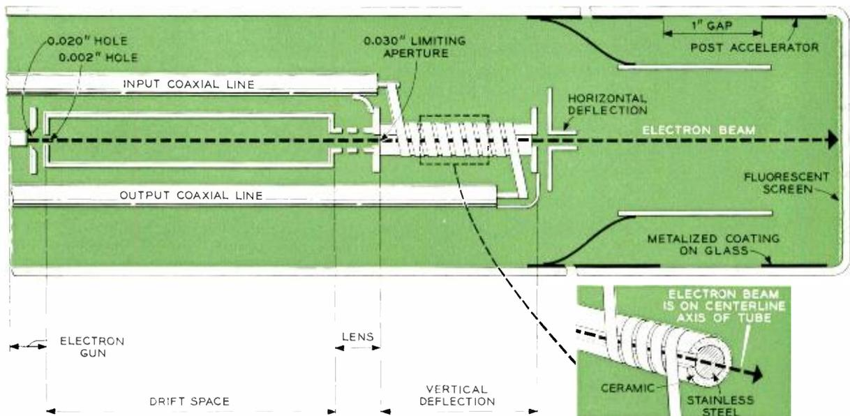
An important aspect of the new broad-band tube is the "multiple" vertical deflecting plates which limit the time the electron spends in a single
