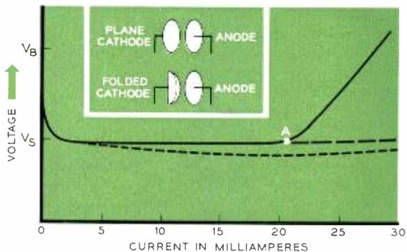
Current-voltage characteristic of plane-cathode tube in high-current state, current plotted linearly. Inset shows plane cathode, top left, and single hollow cathode made by folding plane type.
