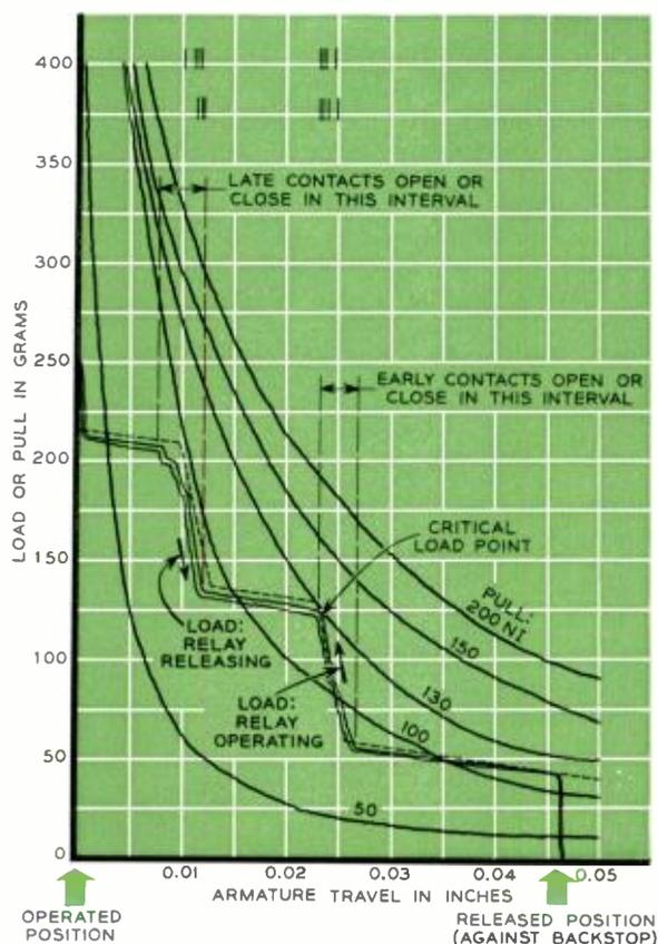
Typical load and pull curves for the “two-in-one” unit. Irregular curves relate load in grams on the armature vs its travel in inches, in both the operate and release directions for this spring relay.
