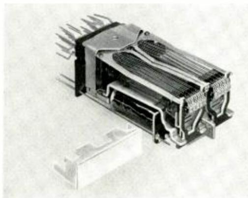
“Two-in-one” wire-spring relay with lyre-shaped cards and formed armature; contact cover at left.
