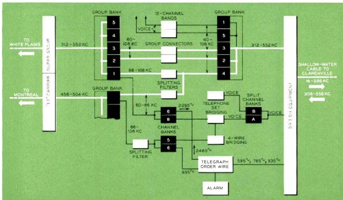
Block diagram of terminal equipment at Sydney Mines, Nova Scotia; this connects the microwave
