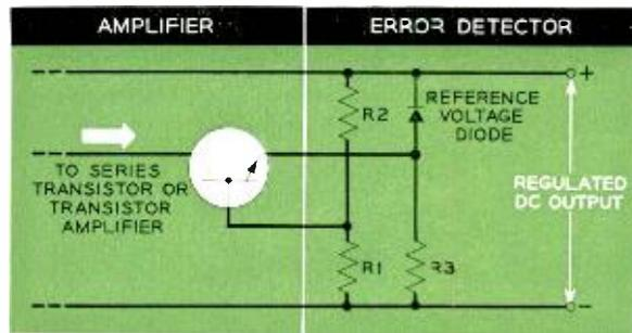
*Circuit arrangement of a typical common-emitter error detector. Circuit works in series regulator.*
