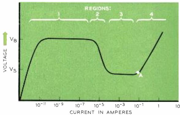
"Breakdown characteristic" of a typical, elementary cold-cathode gas diode. Current is plotted logarithmically.  $V_B$  is the point on the voltage scale at which breakdown occurs.  $V_S$  is the stable operating voltage in the high-current state.
