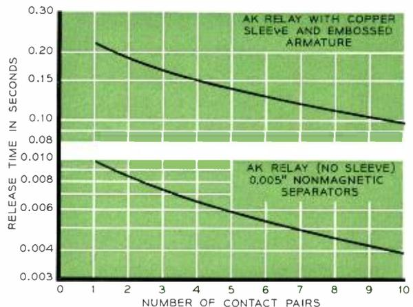
Typical release-time curves for basic and slow-release types. The AK relay (no sleeve) is represented by the lower curve and the AK relay (with copper sleeve) is indicated by the upper curve.
