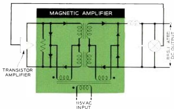
*Transistor magnetic-amplifier regulator used to supply power to Leprechaun transistor computer.*
