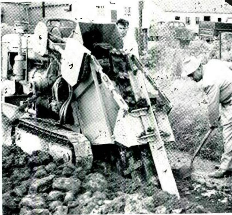
*A crawler-mounted trencher being demonstrated by the manufacturer. Different types of trenching machines are continuously studied as part of the program designed to discover the best-performing equipment for burying cables.*
