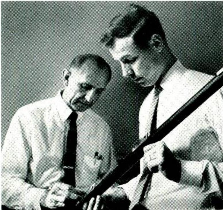
*John B. DeCoste, left, and Richard A. Connolly examine small strip of plastic similar to those to be buried in Roswell tract. Samples are attached to polyethylene rod for burial at 18- and six-inch depths.*
