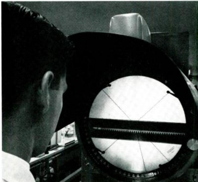
*Western Electric technician inspects helix of a traveling wave tube in an optical "comparator."*
