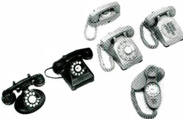
*This group picture shows recent trends in handset design. Two earlier designs, in black, are shown at left. Group at right consists of 500-type set with dial, experimental unit with push buttons, Princess Set, top, and new experimental Dial-In-Handset. The Dial-In-Handset is the first radical departure in handset design.*
