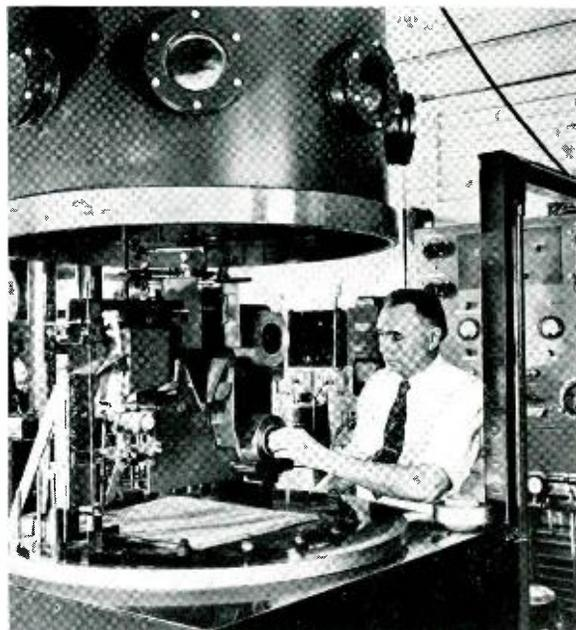
*Operating under a vacuum ( $1 \times 10^{-4}$  millimeter of mercury) this metallizer puts down a zinc coating on each side of the material, to become the fourth and fifth layers of the supported capacitor.*
