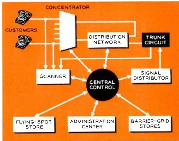
*No major device in ESS can carry out its functions by itself. Each needs the help of central control, which communicates directly with all major units, issuing commands and receiving responses.*
