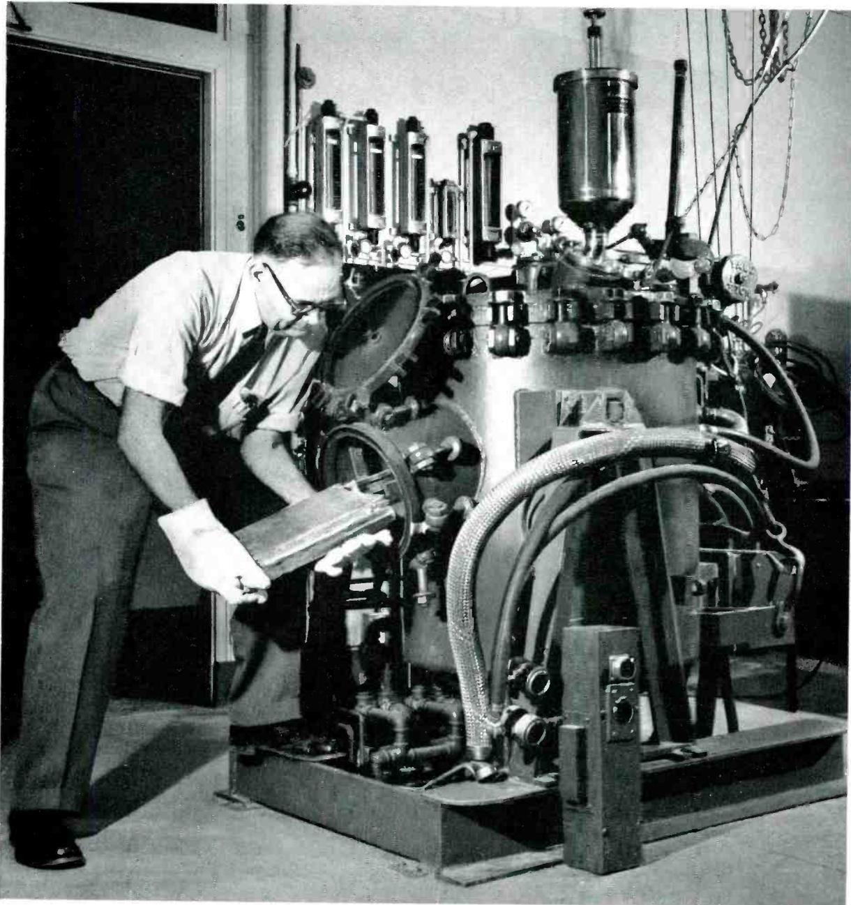
*P. H. Schmitt removes an ingot of high-purity nickel from the controlled-atmosphere melting furnace.*
