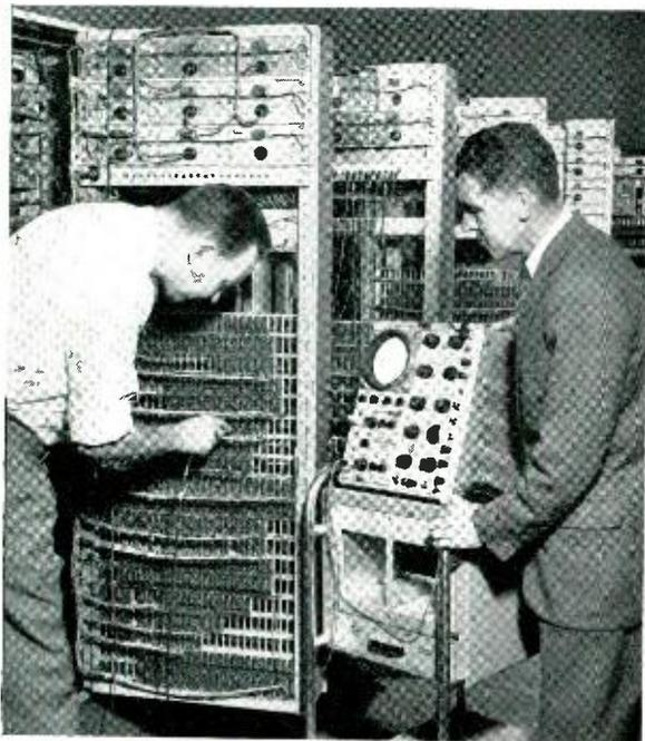
*G. W. Maymon, left, and the author test terminals on the wiring side of a central-control cabinet.*
