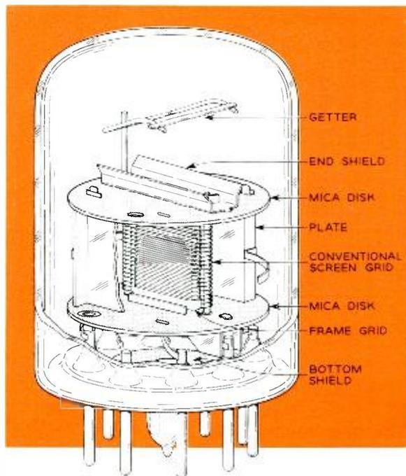
*A cutaway view of the WE 448A, showing the frame-grid construction and the other tube elements.*
