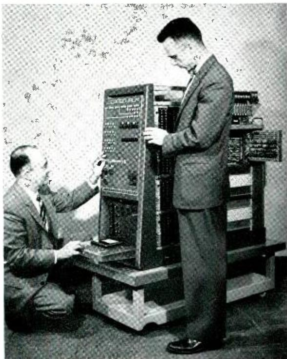
*The author, right, and J. A. Githens check the control panel of Leprechaun. A leaf of one of the books, with circuit patching cords installed, is swung out behind Mr. Baird. Memory is on top.*
