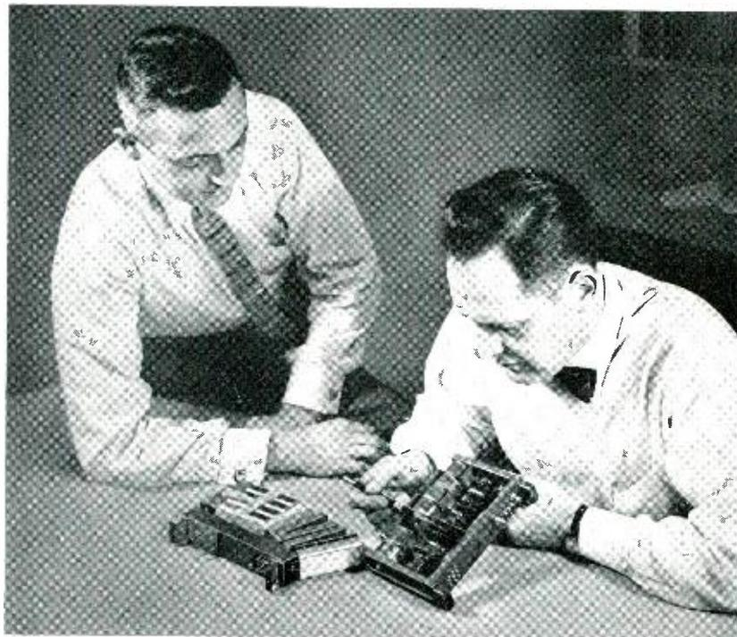
plug and all the pins are molded into the chassis, effectively transforming it into an elaborately shaped connector, capable of housing the entire network. All this is done at a very nominal cost, representing a substantial cost saving compared with that of the stacked assembly. The chassis is shown in the photograph below.
