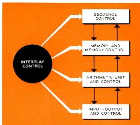
Block diagram showing the major elements of the Leprechaun computer and their relationship to each other. Interplay control is essentially the master control unit of entire computing system.
