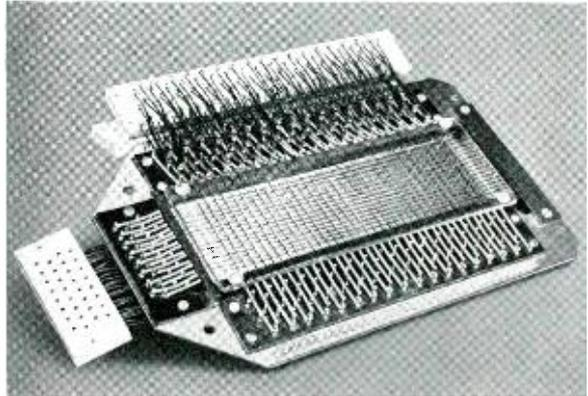
*One plane of the Leprechaun memory system. Magnetic cores are at junctions of wires crisscrossing in center. Eighteen such planes, one for each digit and operated by transistor circuits, make up the entire memory system of the computer.*
