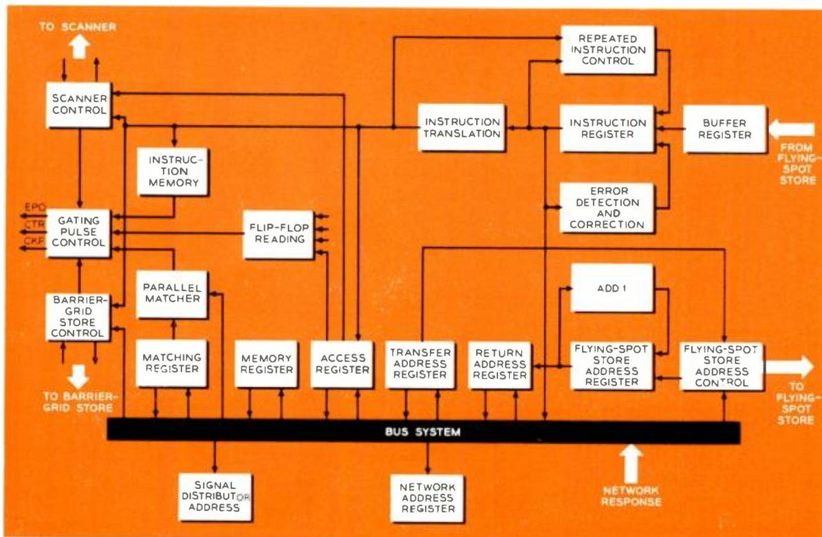
Internal circuitry of the central control for the Electronic Switching System. A bus arrangement
