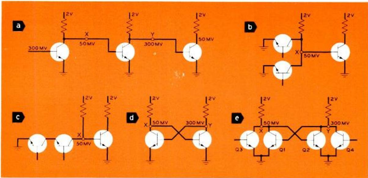
Circuit diagrams show how the two voltage levels for "zero" and "one" are achieved (a), and shows
