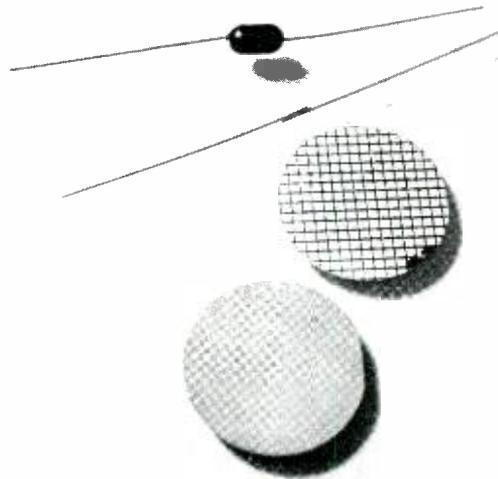
*To make the 100A varistor, from bottom to top, a slice of silicon is diffused, stamped, and gold-plated; slice is etched; resulting wafers soldered between steel leads; and the unit encapsulated.*
