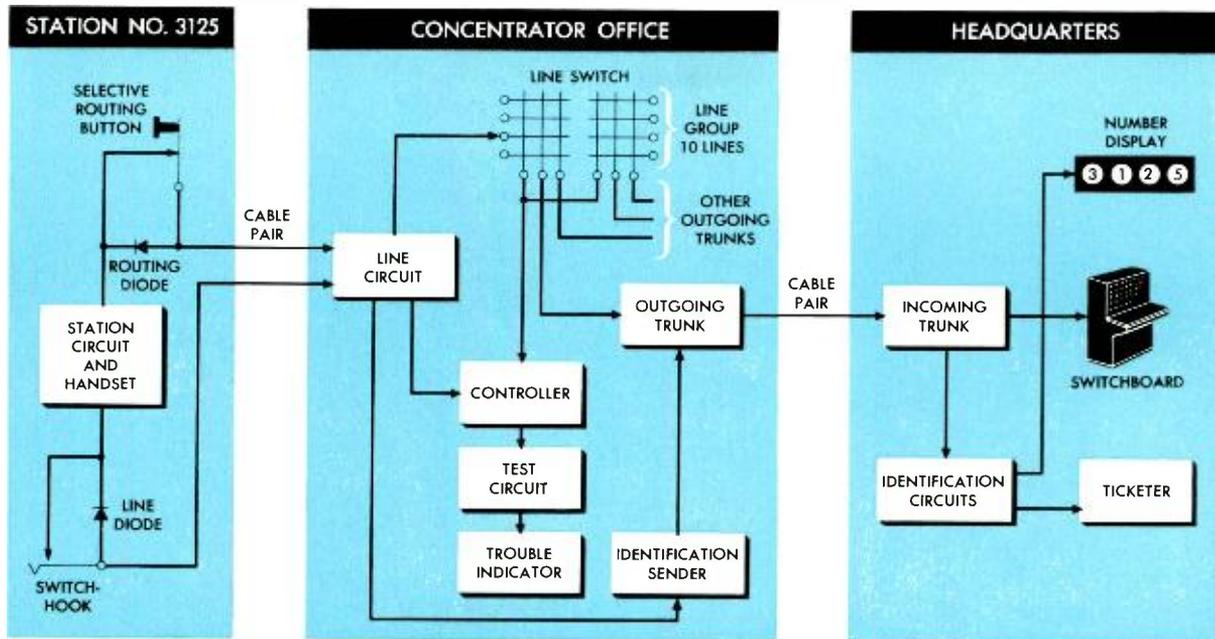
Diagram of the concentrator-type emergency reporting system. The concentrators are located
