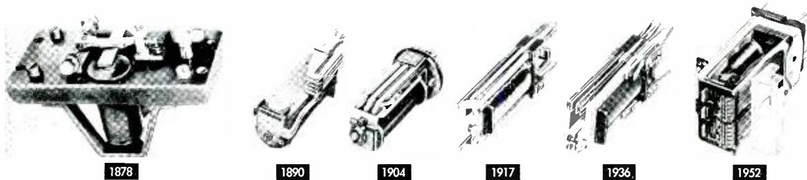
Some steps along the road to modern electro-mechanical relays. At left is telegraph key modified for telephone circuits. Device labeled 1890 depicts first step-by-step telephone switching relay.
