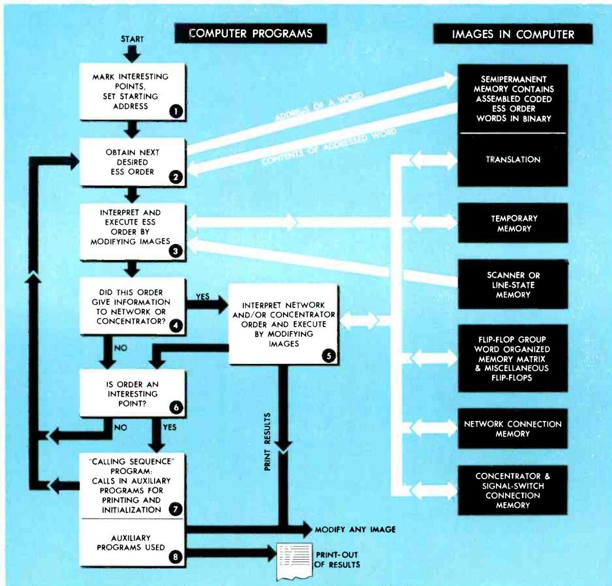
This block diagram shows broadly the progress of a simulation run. All of the information in the images is written into the memory section of the computer and remains there, unchanged, until modified or read out by the computer program. The program portion of the simulation run is executed by the arithmetical and control units of the computer working on the various images.
