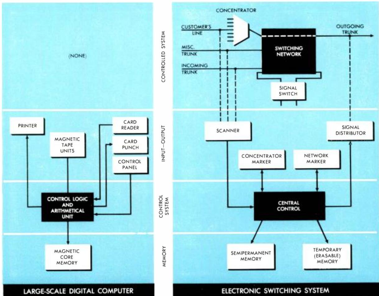
This diagram compares the important elements of an ESS with those of a digital computer. Incom-
