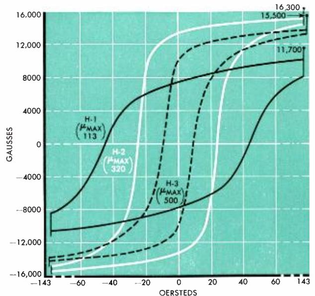
different hardness values. Hysteresis loops on right show magnetic properties of same cores.
