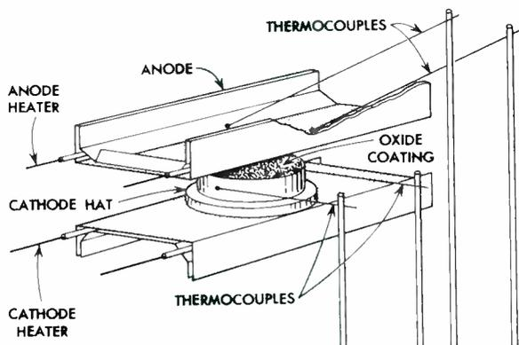
Diagram of the planar diode used in the cathode studies. Thermocouples control tube temperatures.
