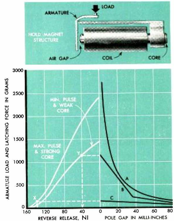
*Design objectives: right, hold-magnet load range and its magnetic-pull characteristics, and, left, range of magnetic-latching forces for the same magnet core. Above, the hold-magnet structure.*
