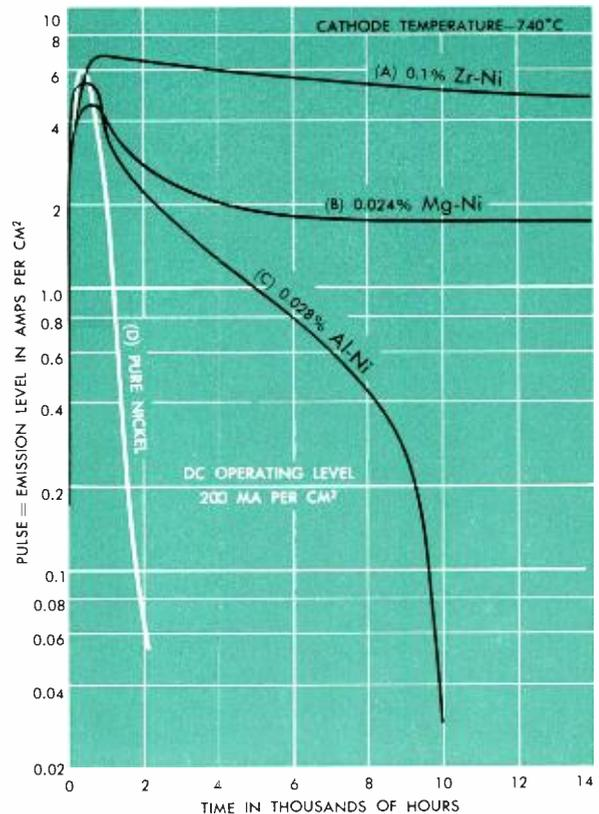
Curves showing emission and life characteristics of three significant cathode alloys and pure nickel.
