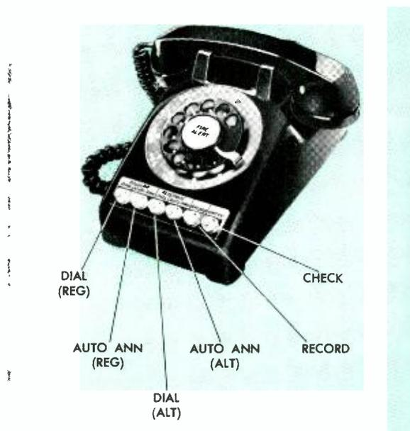
*By dialing a digit on this special telephone, a fire dispatcher can alert one or several groups of volunteer firefighters. A recorder built into this new system repeats the alert over the line.*
