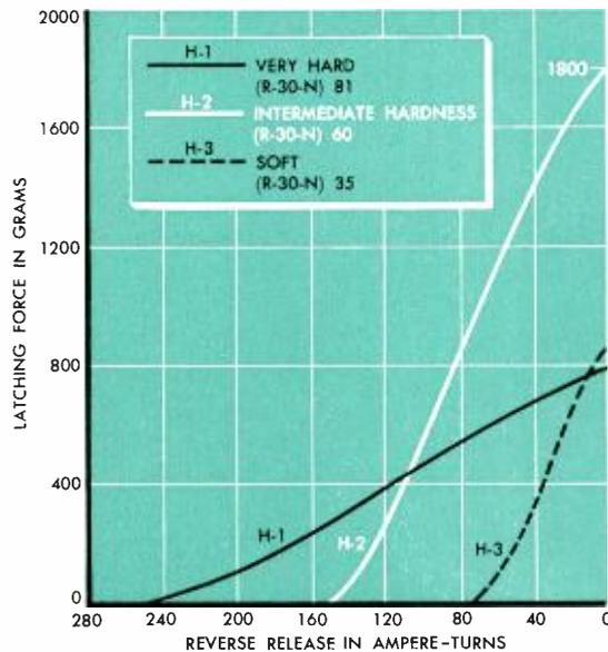
Curves at left show latching force vs. reverse-release ampere turns for cores of three widely
