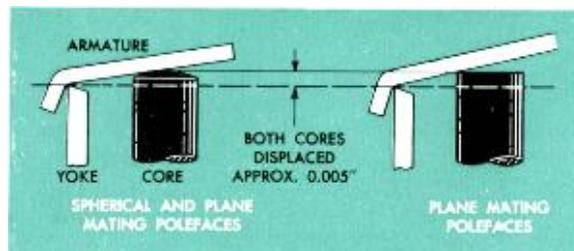
*The importance of poleface shape showing effect of misalignment on closed polegap reluctance.*
