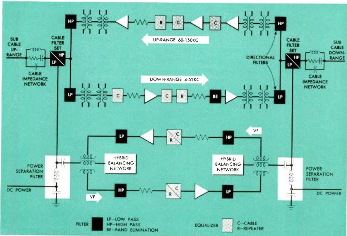
Special devices at an unattended repeater on Air Force cable serve to separate power current from
