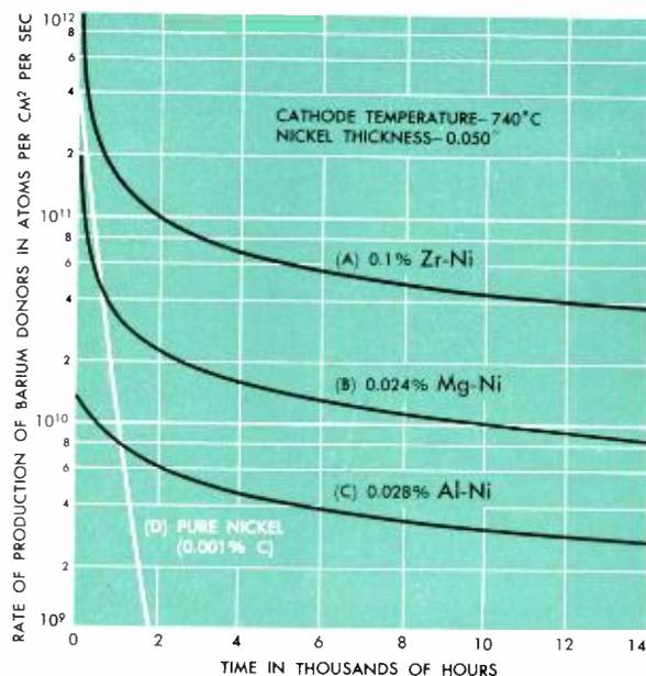
Donor-production rates vs. time for the three alloys and nickel shown in emission curves. Curves were plotted from diffusion data in table above. Alloys are same as in curves on page 454.
