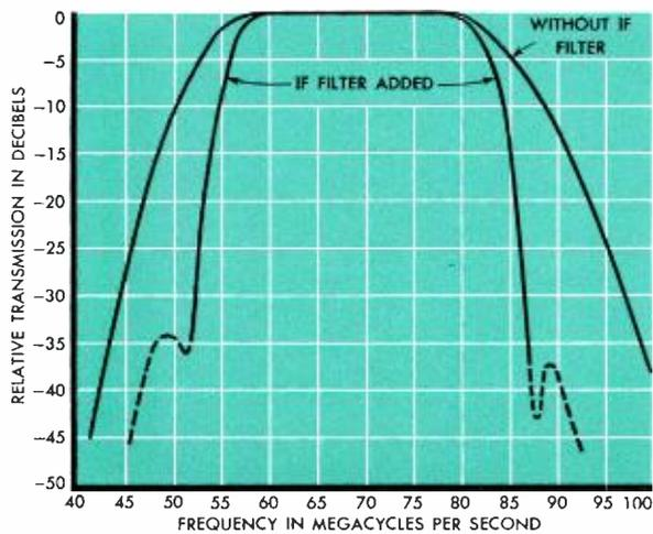
*Radio receiver gain-frequency characteristics showing loss obtained by placing an additional IF filter ahead of the 70 mc amplifier in each receiver.*
