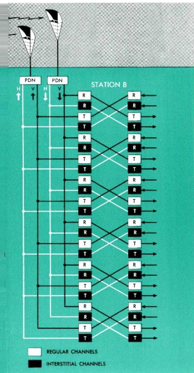
is made possible by the practical method of cross-polarization and the use of horn-reflector antenna.
