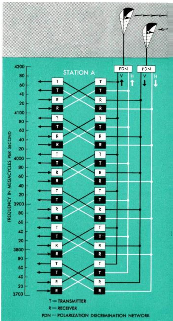
TD-2 system with interstitial channels. The use of entire broadband channel between 37 and 42 mc
