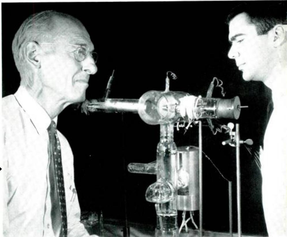
*L. H. Germer, left, and A. U. MacRae are shown with the apparatus used in a new technique for studying the adsorption of monolayers of gas on the surface of a crystal.*
