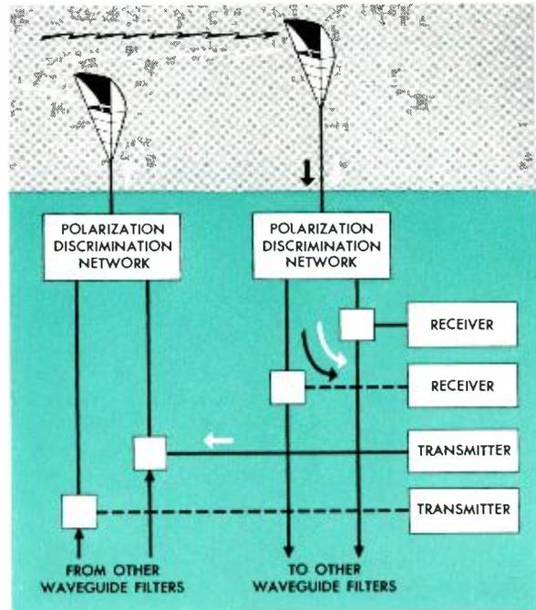
*The effect of mutual coupling between the transmitting and the receiving antennas on the same tower. Extra IF filter helps reduce coupling loss due to interference between the two antennas.*
