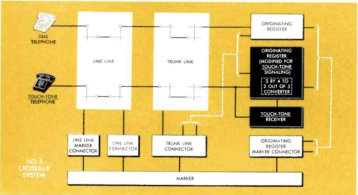
experimental TOUCH-TONE system used the two-out-of-five multifrequency signaling. Laboratories engineers, however, found that a three-by-four multifrequency system would be even better than the two-out-of-five.
