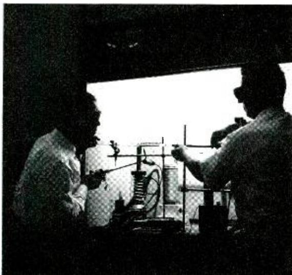
*E. S. Greiner, left, and J. A. Gutowski seal the quartz tube in which silicon ribbons are grown.*
