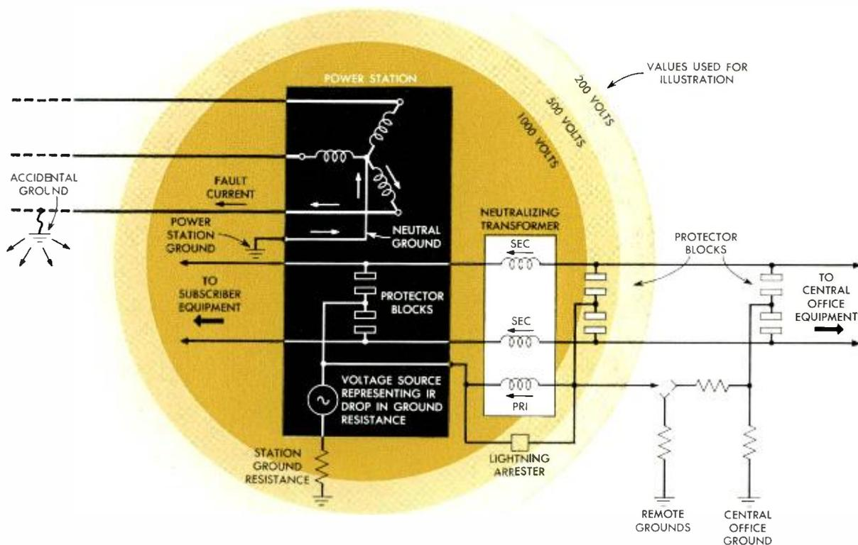
Arrangement of protector blocks and neutralizing transformer on the lines serving a power station.
