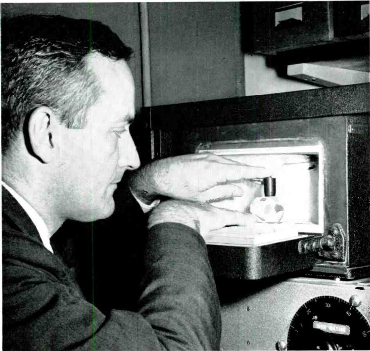
*J. C. King places quartz crystal in furnace for electrolysis treatment. Wafers cut from quartz are*
