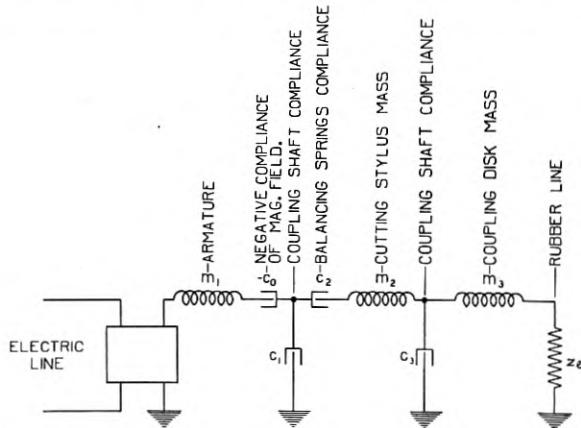
Fig. 12—Equivalent electric circuit of the electromagnetic recorder
