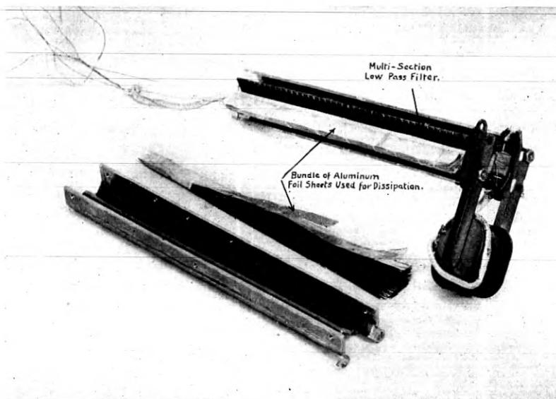
Fig. 13—Electromagnetic recorder using lumped loaded termination
