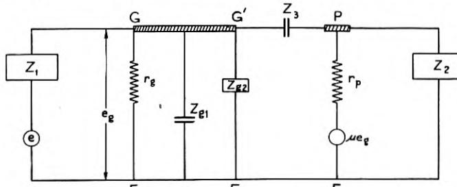
Fig. 5—Equivalent network
