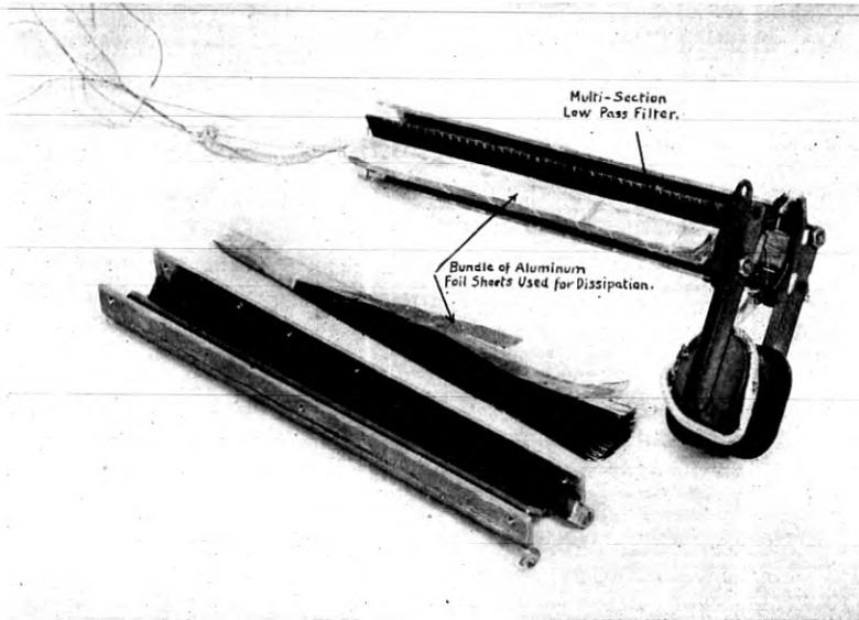
Fig. 13—Electromagnetic recorder using lumped loaded termination
