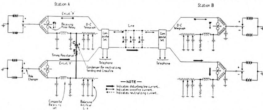
Fig. 4—Method of neutralizing sending-end crossfire between two telegraph circuits
