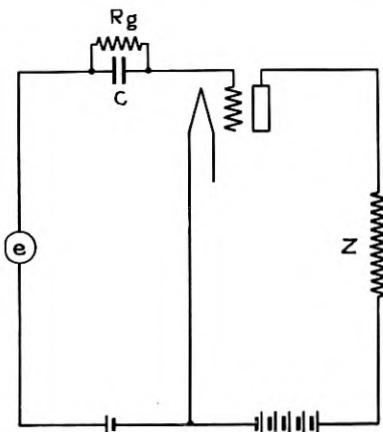
Fig. 3—Grid-leak detector
