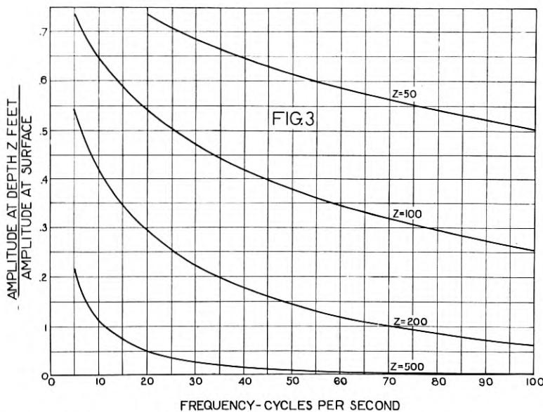
$z$  below the surface of an infinite plane conductor are given by the formulas:<sup>3</sup>
