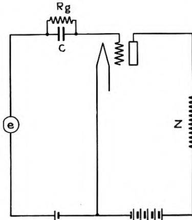
Fig. 3—Grid-leak detector
