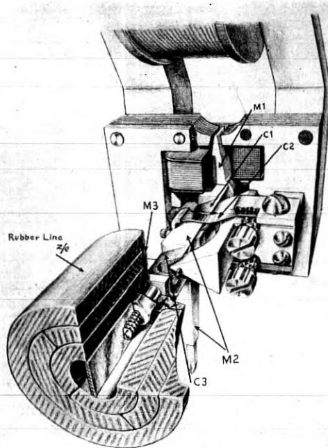
Fig. 11—Detailed drawing of the mechanical filter of an electromagnetic recorder.
