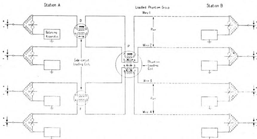
Fig. 6—Effect of loading coils on crossfire
