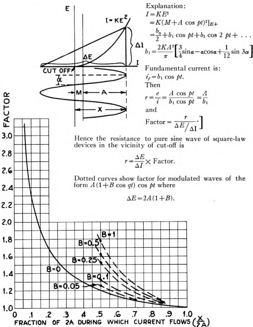
Fig. 7—Correction factor for resistance of non-linear device
