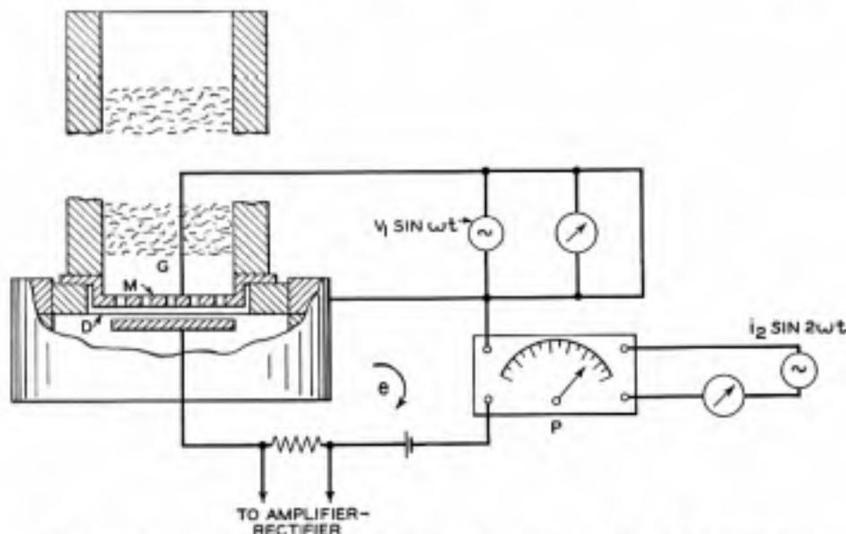
Fig. 8—Electrostatic method—auxiliary third electrode driving diaphragm.
