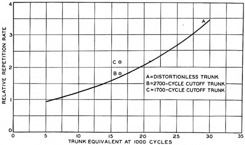
Fig. 1—Relation between repetition rate and trunk equivalent.
