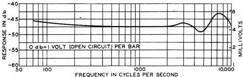
Fig. 9—Pressure calibration of the 387-type carbon microphone.
