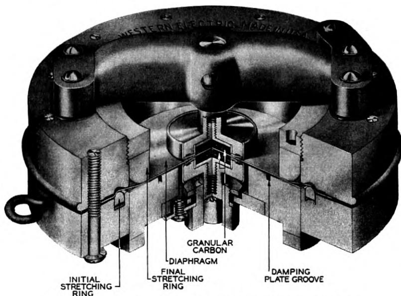
Fig. 8—Cross-sectional view of the 387-type carbon microphone.
