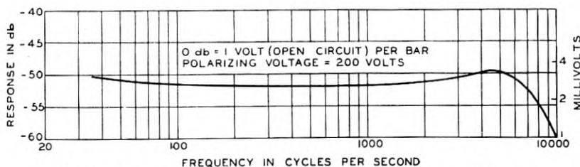
Fig. 4—Pressure calibration of the 394 type condenser microphone.
