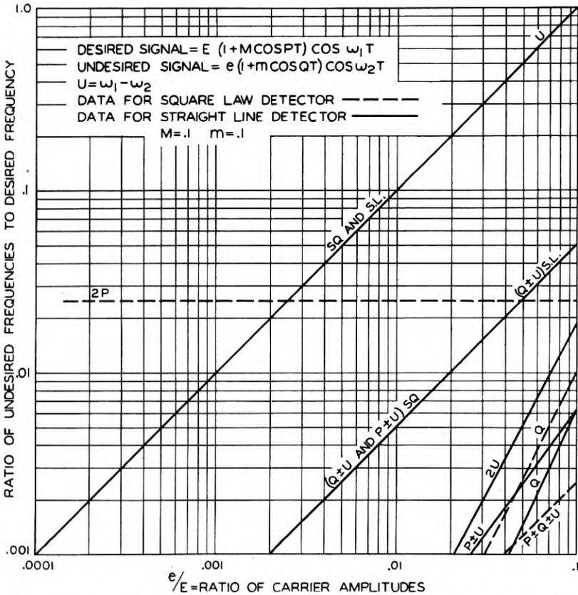
Fig. 1—Relative amplitudes of undesired frequencies as a function of the ratio of the amplitudes of the desired and the interfering carriers. Modulation of both stations small and equal.
