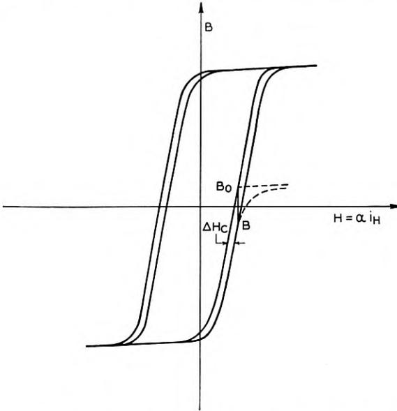
Fig. 10—A diagram to illustrate the widening of a loop due to inductance.
