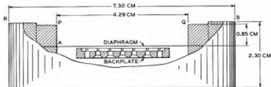
Fig. 1A—Contour dimensions of No. 394-type condenser transmitter.
