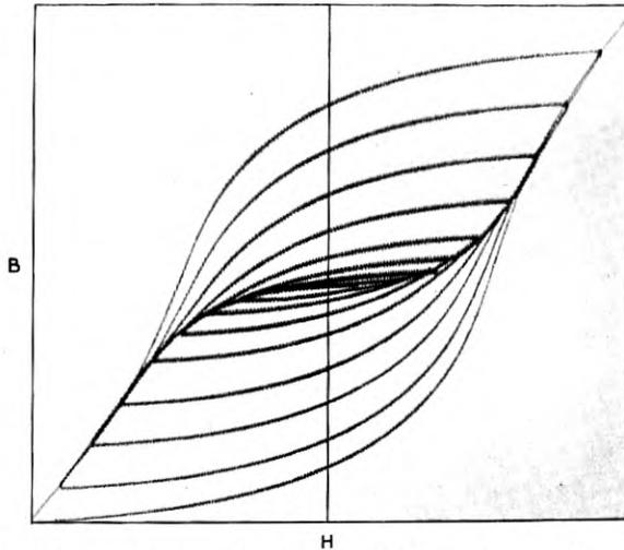
Fig. 6—Hysteresis loops of hard iron, with increasing maximum fields.
