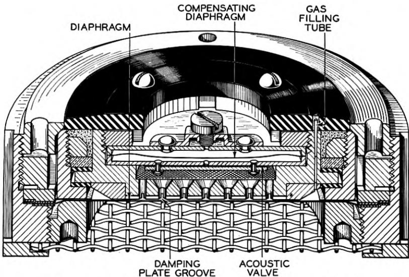
Fig. 2—Cross-sectional view of the 394-type condenser microphone.
