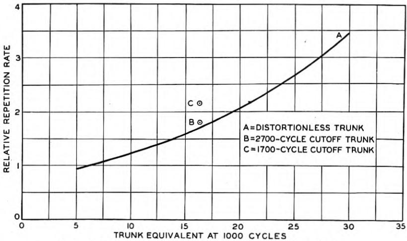
Fig. 1—Relation between repetition rate and trunk equivalent.
