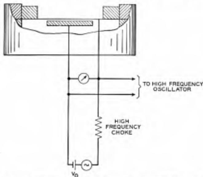
Fig. 7—Electrostatic method—Back electrode serving as driving electrode.
