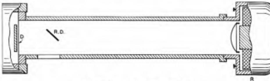
Fig. 4—Resonating tube method.
