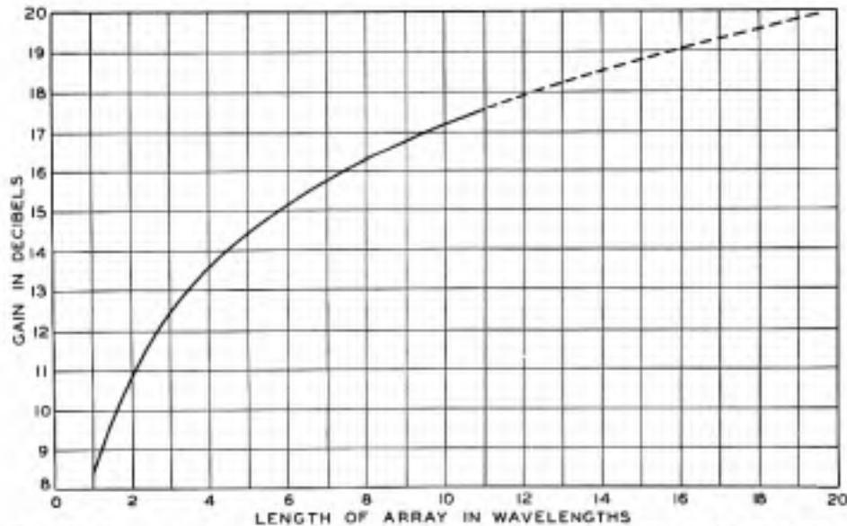
Fig. 10—Approximate gains to be expected from arrays of couplets for spacings of approximately  $\lambda/4$  and  $\lambda/2$ .
