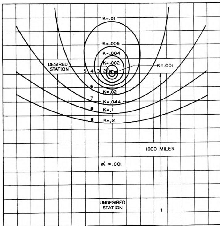
Fig. 5—Curves along which the ratio of the carrier amplitudes received from two stations has a constant value  $K$ , as indicated. Attenuation small.
