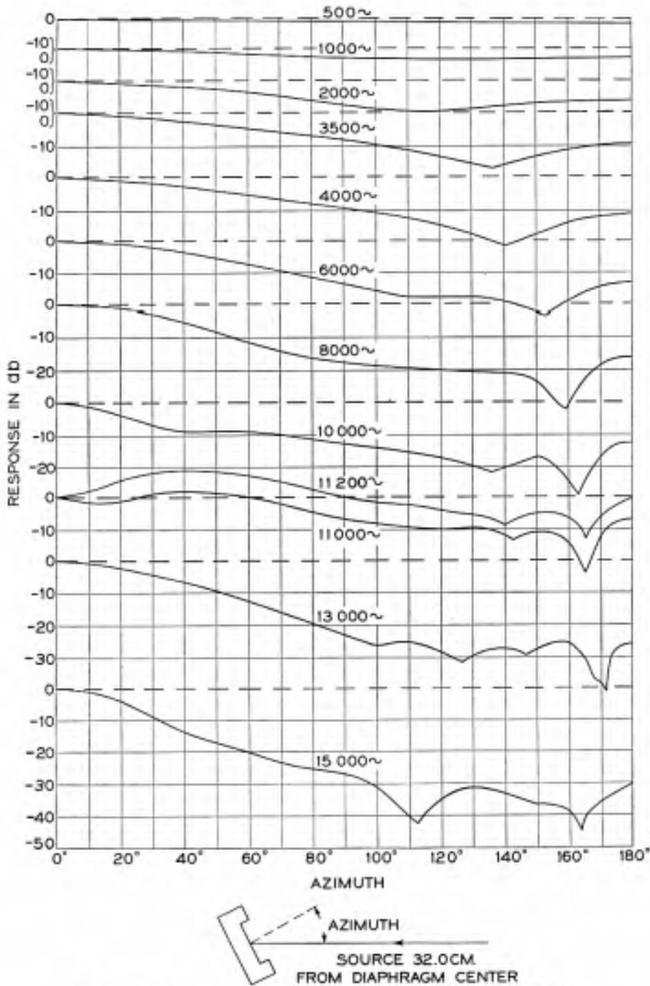
Fig. 11—Azimuth response of No. 394-type condenser transmitter.
