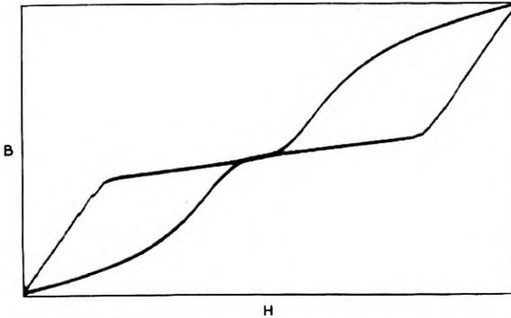
Fig. 7—Hysteresis loop of permivar, showing the “wasped” loop.
