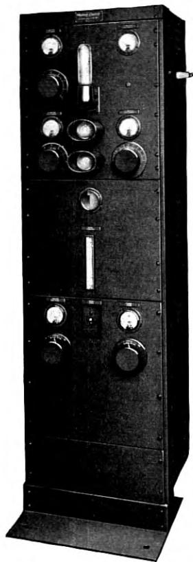
Fig. 3—Front view of crystal controlled oscillator-amplifier unit.
