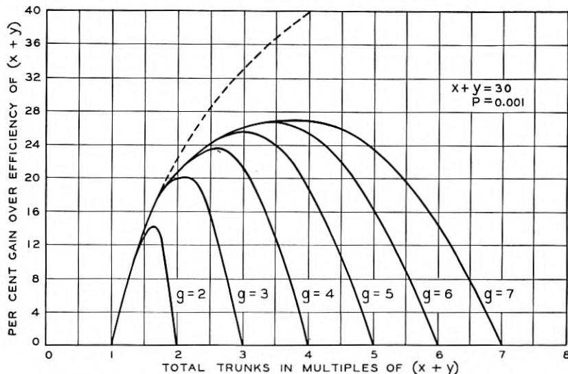
Fig. 14—Graded multiple efficiency.  $x + y = 30$ .  $P = 0.001$ .
