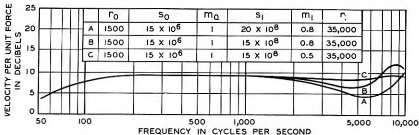
Fig. 7—Theoretical response curves of moving coil microphone.
