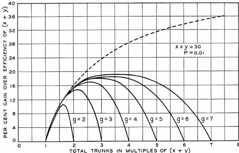
Fig. 10—Graded multiple efficiency.  $x + y = 30$ .  $P = 0.01$ .
