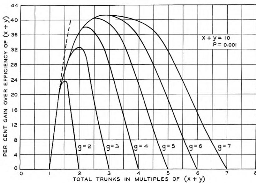
Fig. 12—Graded multiple efficiency.  $x + y = 10$ .  $P = 0.001$ .
