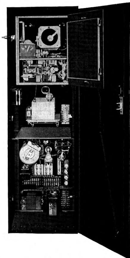
Fig. 4—Rear view showing interior of oscillator-amplifier unit.
