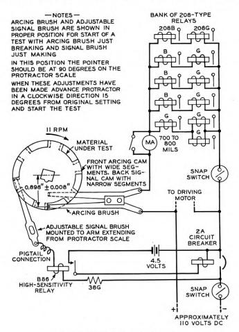
Fig. 8-Circuit for arc resistance test.
