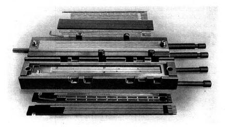
Fig. 1—Panel system commutator (flash type mold).
