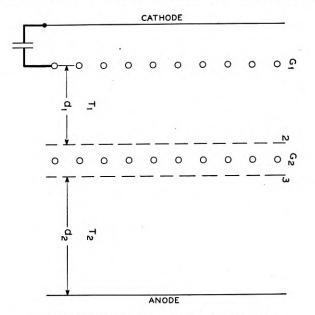
Fig. 3-Schematic of a space charge grid tube.
