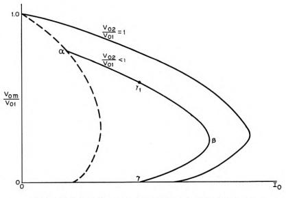
Fig. 2—Variations of the magnitude of the potential minimum as function of injected current.
