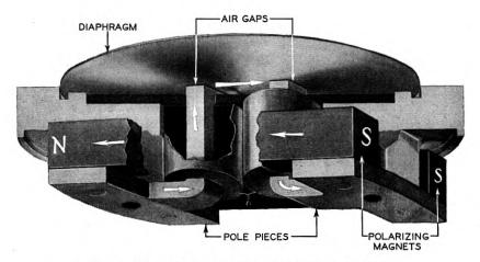
Fig. 6-Magnetic circuit of the new telephone receiver.
