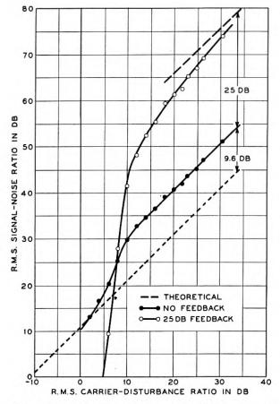
Fig. 15—Output signal-to-noise ratio vs. carrier-disturbance ratio with and without feedback. Modulation  $\pm$  124.5 kilocycles for 25-decibel feedback and  $\pm$  7 kilocycles for no feedback.
