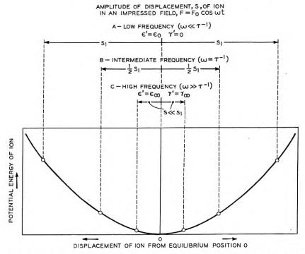
Fig. 3-The mechanism of anomalous dispersion illustrated by a simple model.
