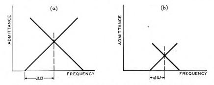
Fig. 2—Idealized conversion-system characteristics for (a) limiter system, (b) feedback system.
