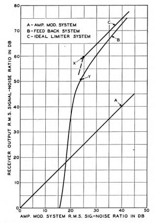
Fig. 16—Theoretical comparison of signal-to-noise ratios obtained at 25-decibel feedback (curve *B*) with amplitude-modulated system (curve *A*) and ideal limiter system with deviation ratio = 31.1 (curve *C*). Point X = threshold of noise improvement for limiter system. Point Y = point where "crackling" first became evident in the presence of  $\pm$  124.5-kilocycle modulation.
