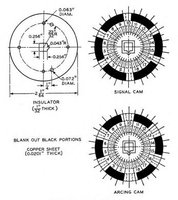
Fig. 7-Arc resistance test cam.
