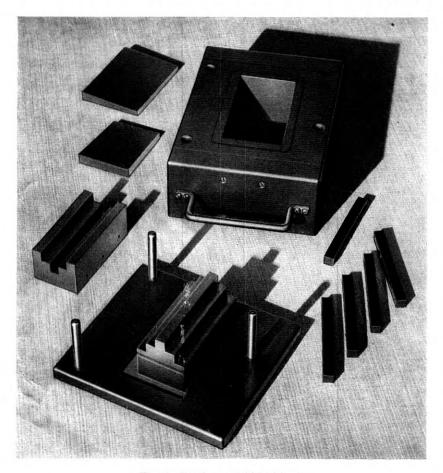
Fig. 5-Specimen mold and bars.
