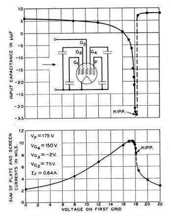
Fig. 11—Measured input capacitance of experimental vacuum tube no. 59 (grid signal = 0.05 volts r.m.s. at 50 kc.).
