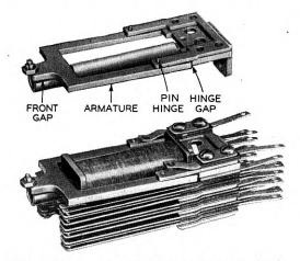
Fig. 4-U-type relay, showing the magnetic circuit
