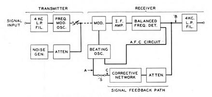
Fig. 4-Schematic of experimental feedback system.
