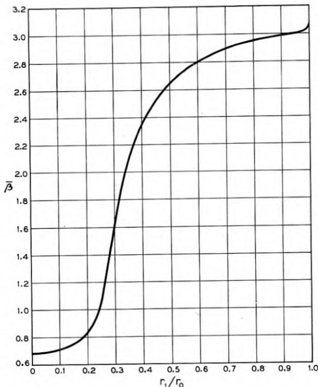
Fig. 1 — Propagation constant of a circular guide containing an unmagnetized coaxial, dielectric rod ( $\epsilon/\epsilon_0 = 10$ ).  $r_1$  is the radius of the rod and  $r_0$  the radius of the guide.  $r_0 = 0.4\lambda_0$ , where  $\lambda_0$  is the free space wavelength.
