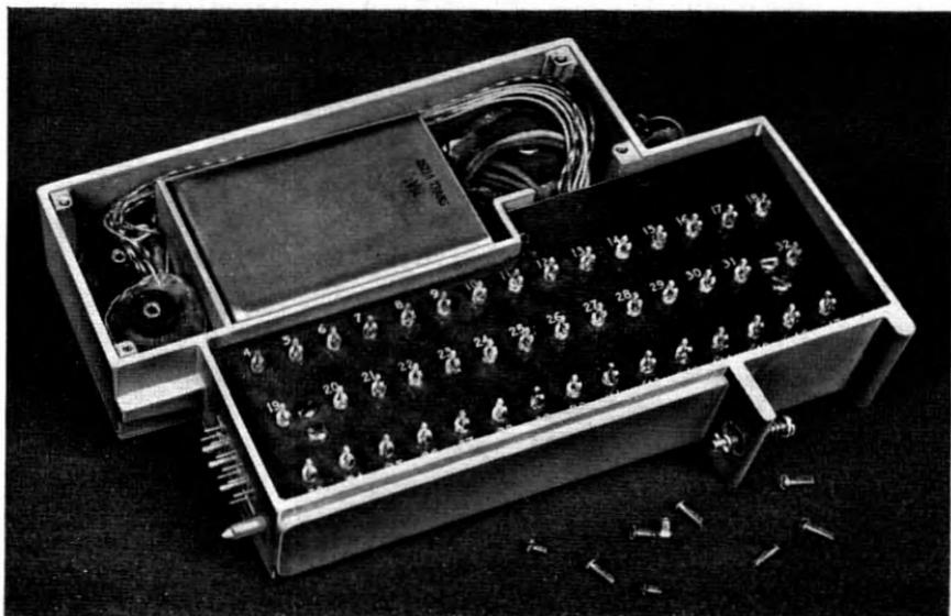
Fig. 20 — Assembly and wiring of E2 repeater.
