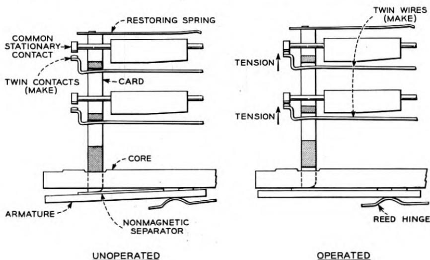
Fig. 5 — Principal of contact operation.
