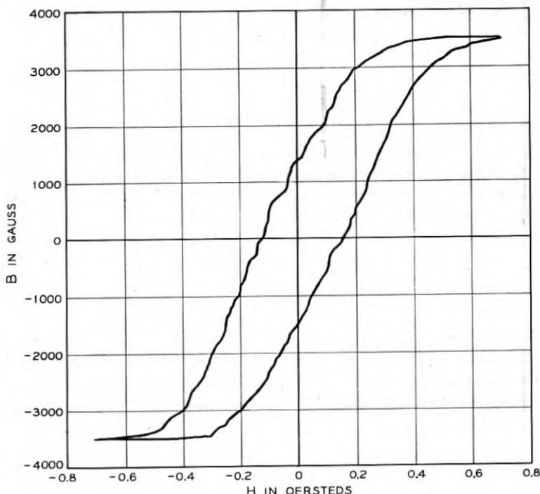
Fig. 2 — Hysteresis loop taken on sample before heat treatment in a magnetic field.
