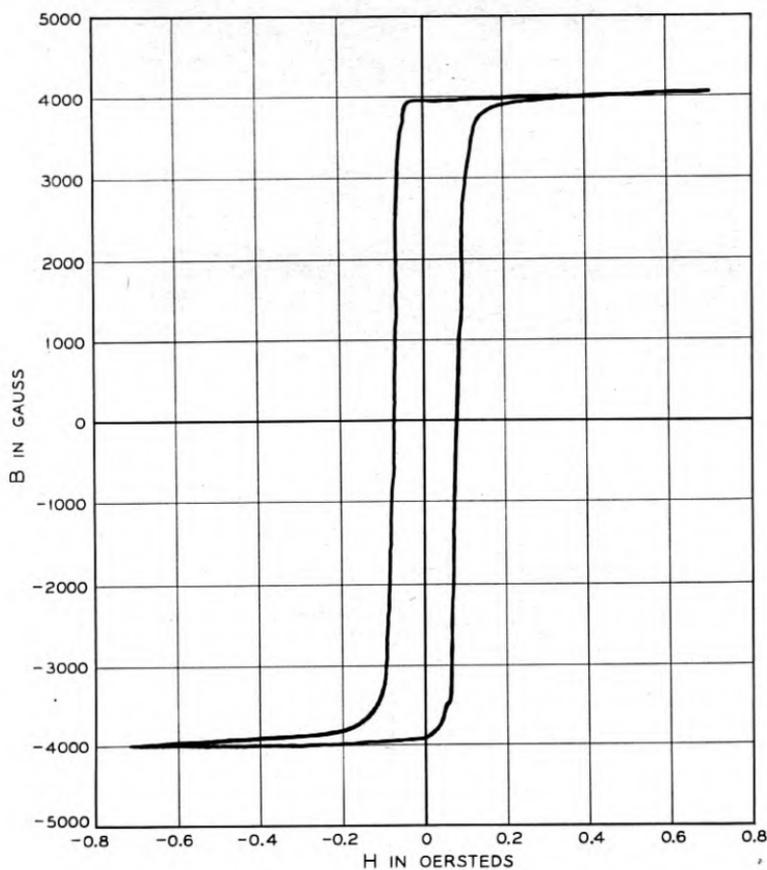
Fig. 3 — Hysteresis loop taken on same sample as loop in Fig. 2 after annealing for one hour at 580°C in a magnetic field of approximately 20 oersteds.
