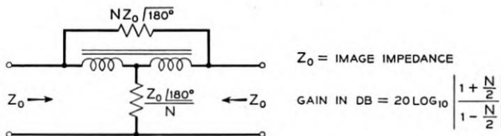
Fig. 12 — Schematic of the bridged T repeater.
