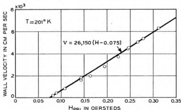
Fig. 7 — Typical plot of actual data for domain wall velocity as a function of applied field.
