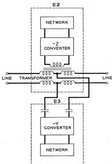
Fig. 10 — The bridged T repeater E23.
