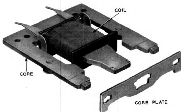
Fig. 7 — Core legs are held in alignment by the core plate, which is forced on the ends after the coil is assembled.
