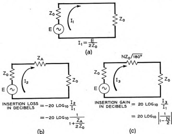
Fig. 13 — Insertion gain of the E2 repeater.
