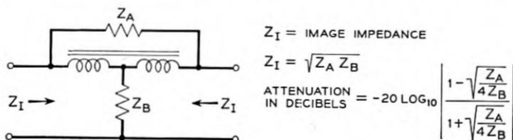
Fig. 11 — Schematic of the bridged T network.
