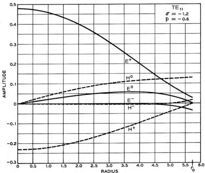
Fig. 9 — Amplitude of the field components in filled cylindrical guide, longitudinally magnetized, as a function of radius, for the  $TE_{11}$ -limit and  $TM_{11}$ -limit modes at several values of  $\sigma$ .  $r_0 = 5.75$ .  $|p| = 0.6$ , except for Figs. 9(f) and (p) which are the isotropic cases,  $\sigma = p = 0$ . The fields are normalized to a constant power flow per (free space wavelength)<sup>2</sup>. (a), top, (b), bottom.
