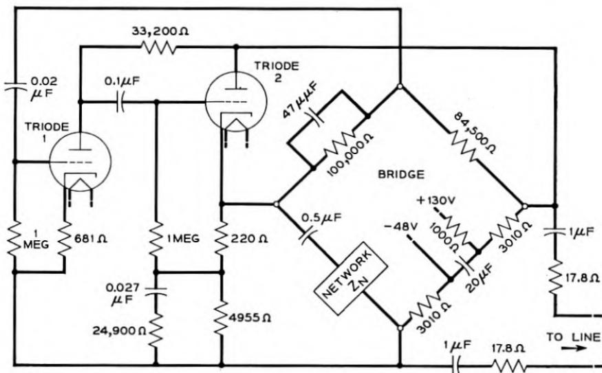
Fig. 17 — Schematic circuit of E3 repeater.
