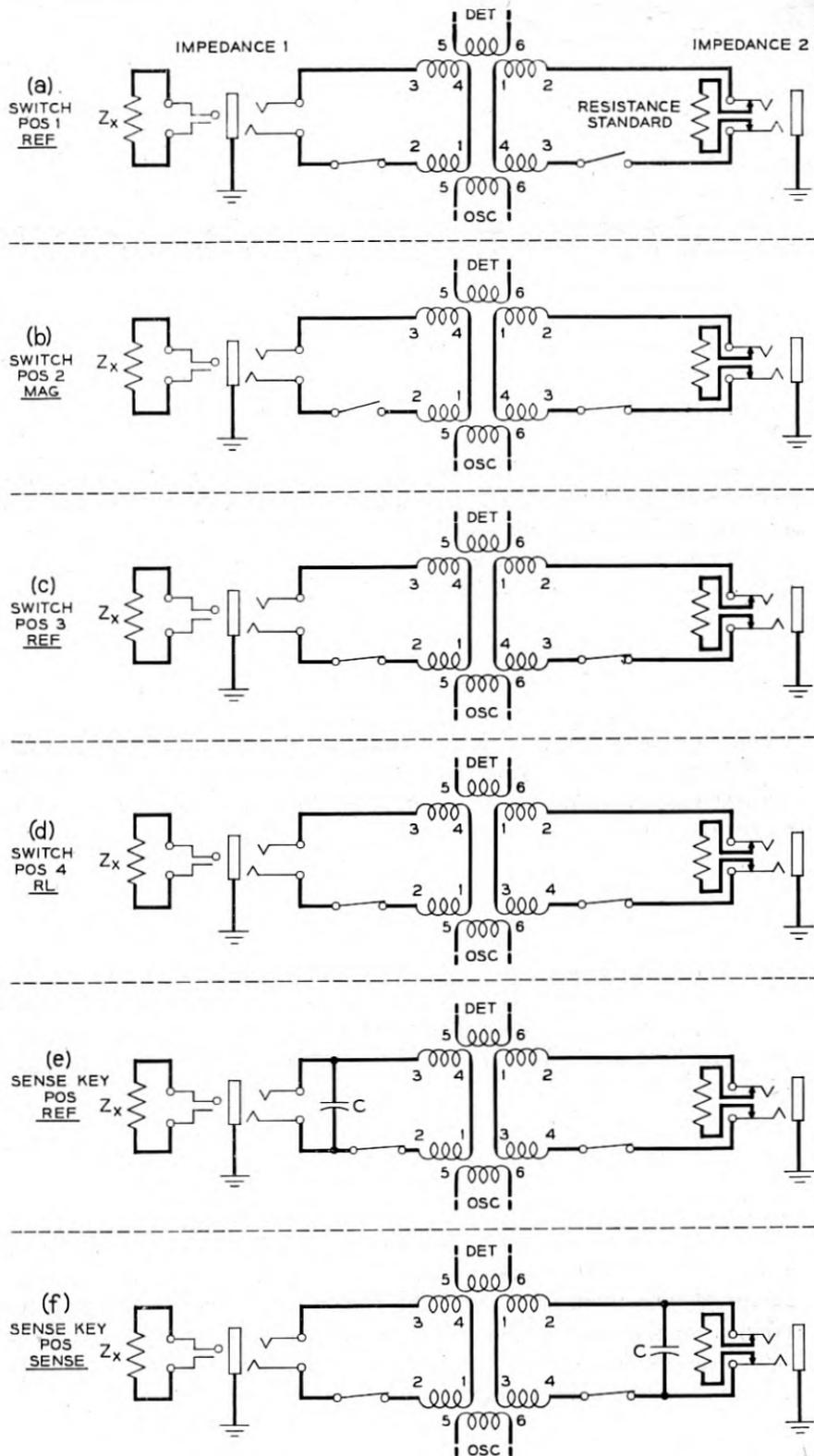
Fig. 27 — Sequence of impedance measurements.
