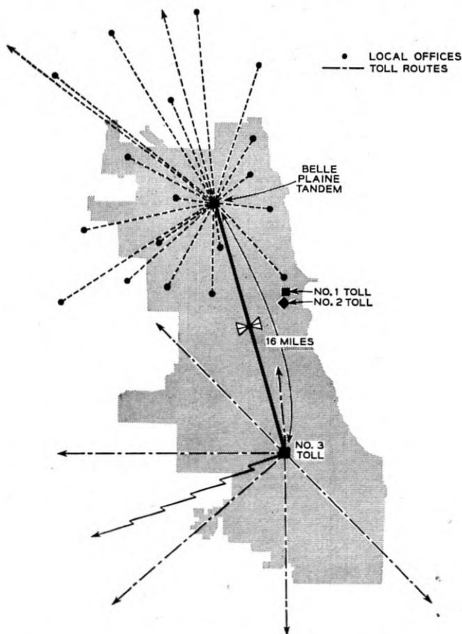
Fig. 4 — Typical E23 repeater application; Chicago toll tandem trunks.
