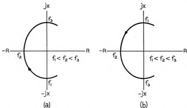
Fig. 6 — The two types of negative impedance: (a) Open Circuit Stable and (b) Short Circuit Stable.
