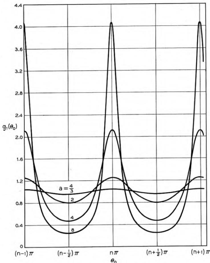
Fig. 6 — Rotation gain,  $g_1(\theta_0)$ , versus electrical thickness,  $\theta_0$ , for small magnetization.
