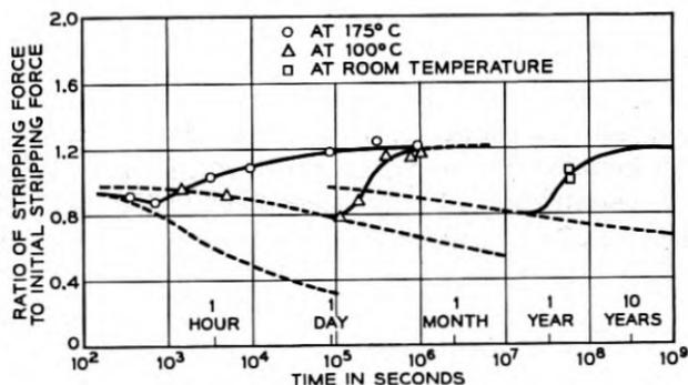
Fig. 5 — Ratio of measured stripping force to initial stripping force as a function of time and temperature for tinned copper wire on nickel silver terminals.
