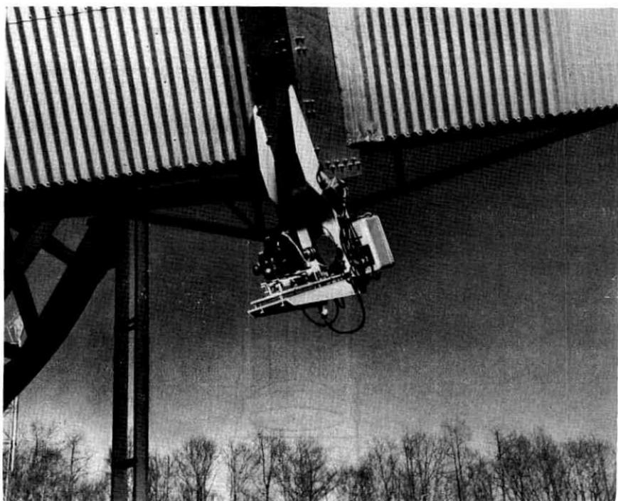
Fig. 4 — Camera mounted on horn receiver.
