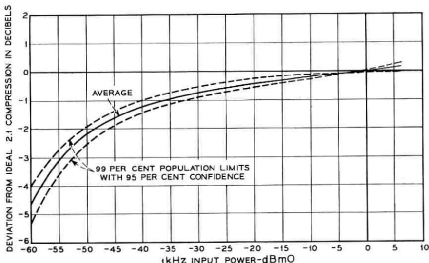
Fig. 8 — N3 channel compressor tracking characteristic.
