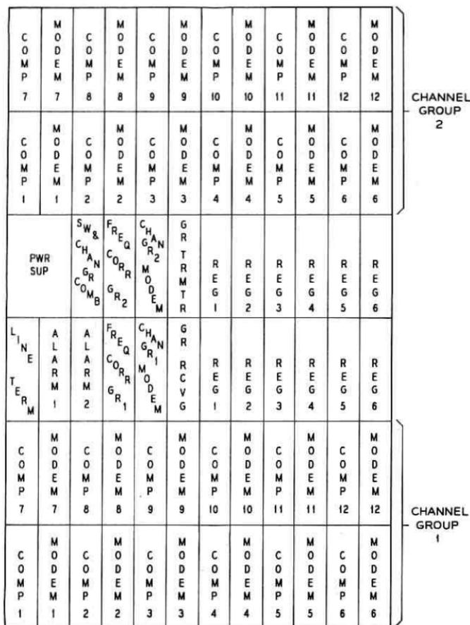
Fig. 1 — N3 carrier terminal — location of plug-in units.
