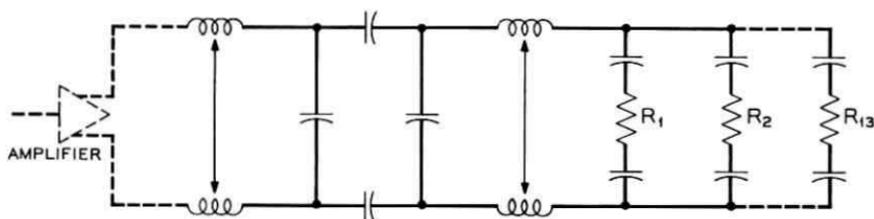
Fig. 29—Primary distribution circuit.
