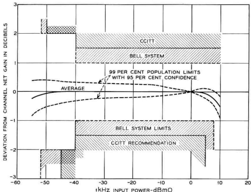
Fig. 7—N3 channel compandor tracking characteristic.
