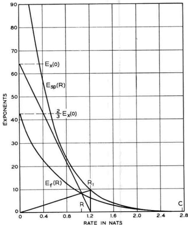
Fig. 1 — Construction for  $E_f(R)$  on AGC,  $S/N = 256$ .
