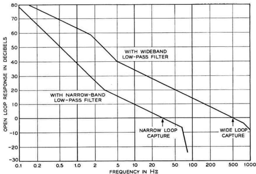
Fig. 15 — Open loop response of correction circuit.
