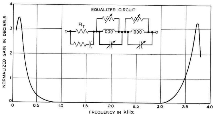
Fig. 7—Frequency characteristic of demodulator amplifier including channel equalizer.
