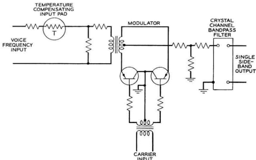
Fig. 3 — Channel modulator circuit.
