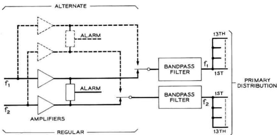
Fig. 25 — Amplification and distribution.
