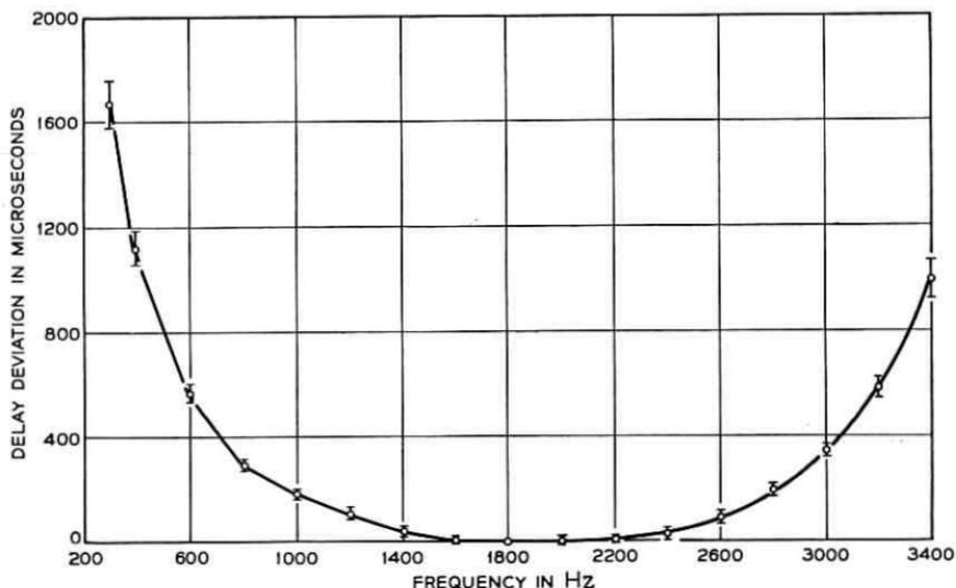
Fig. 9 — N3 channel delay distortion characteristic.
