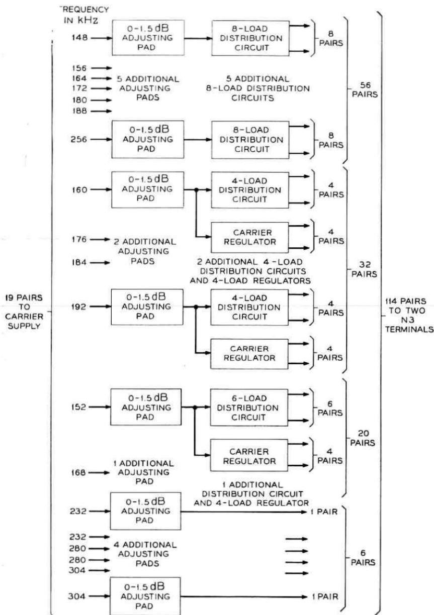
Fig. 30 — Secondary carrier distribution circuit.
