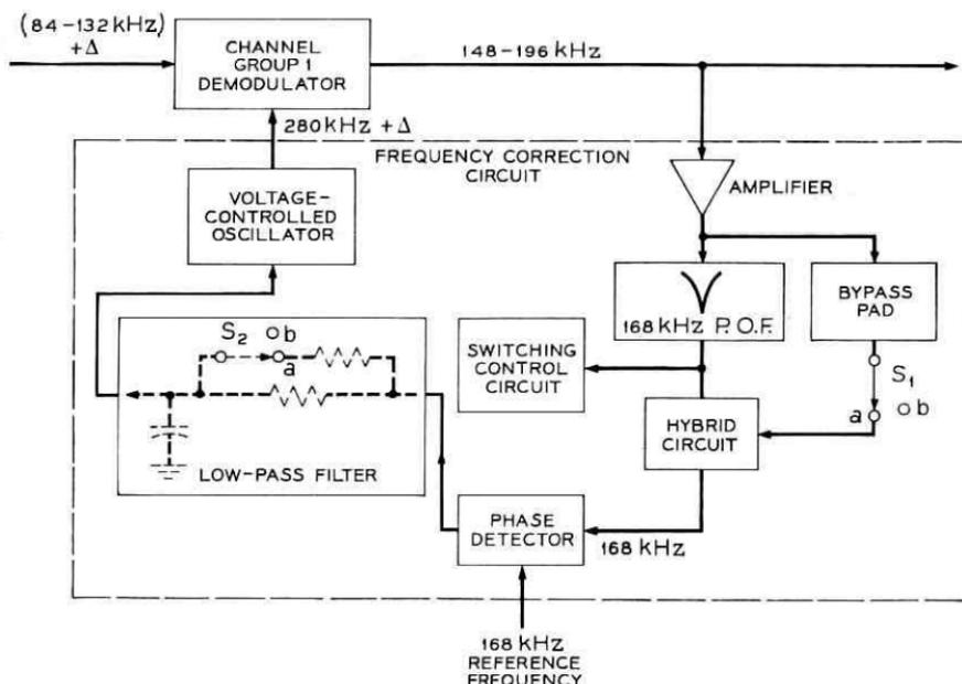
Fig. 14 — Block diagram of frequency correction circuit.
