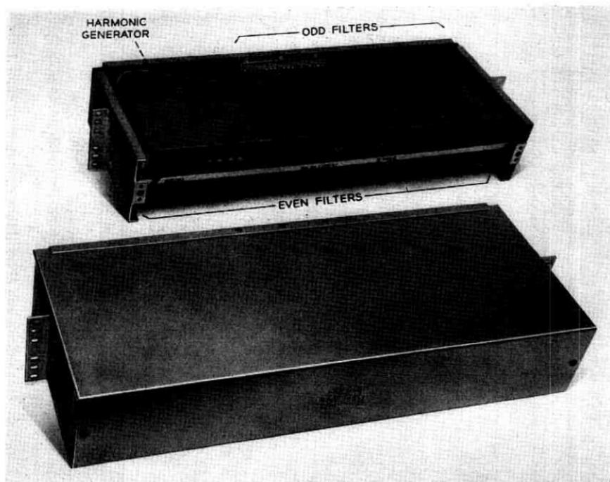
Fig. 22—Harmonic generator and carrier filter panel shown with and without protective cover.
