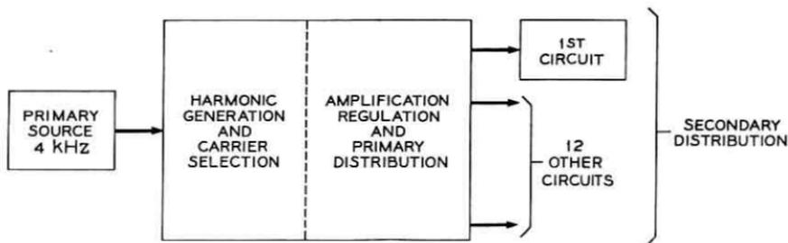
Fig. 19 — Carrier-supply — general plan.
