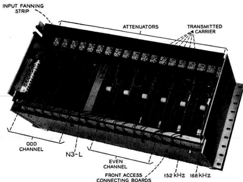
Fig. 25—Secondary carrier distribution panel (rear view).
