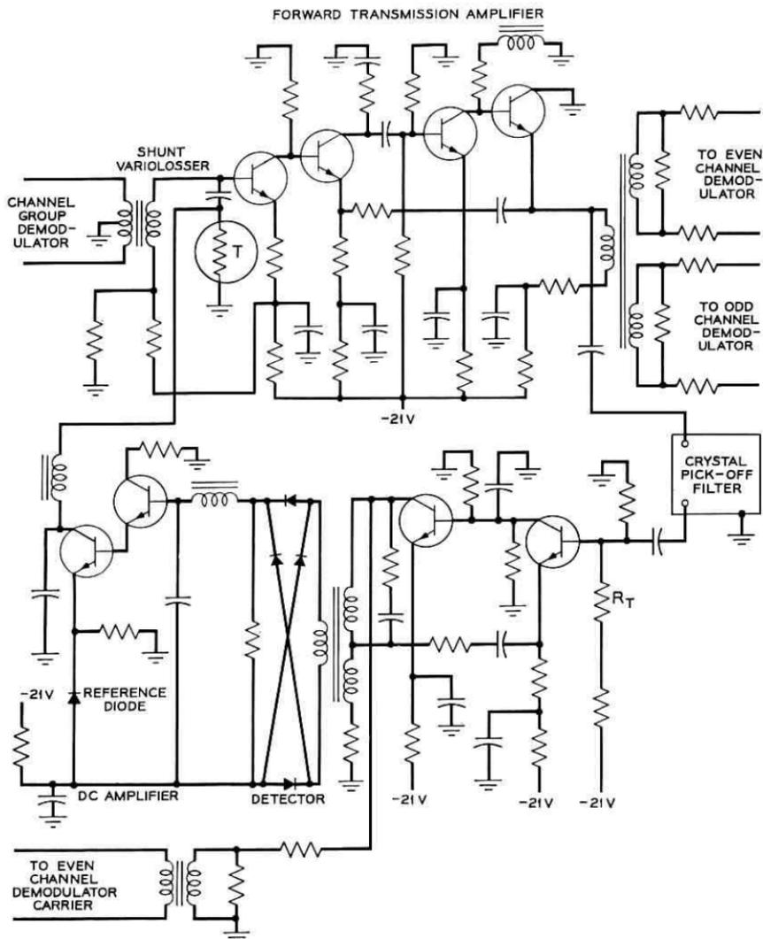
Fig. 8 — Double-channel regulator.
