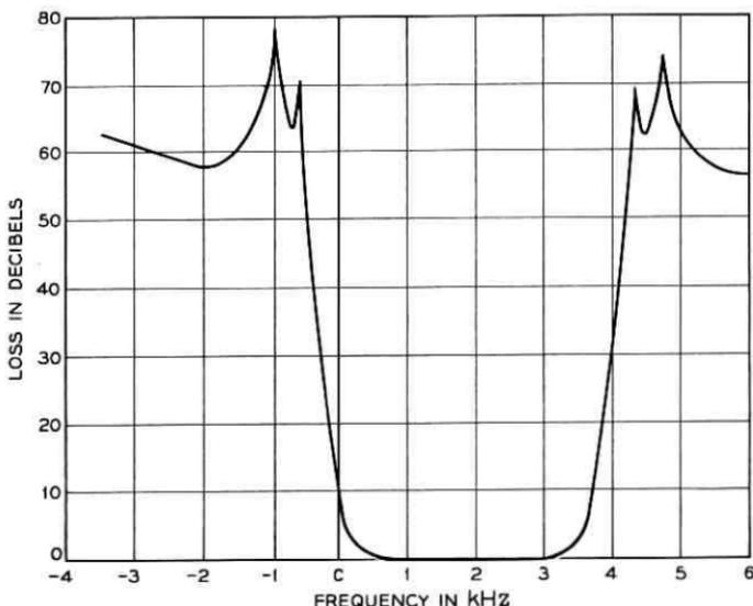
Fig. 4 — Measured insertion loss N3 channel band filter.
