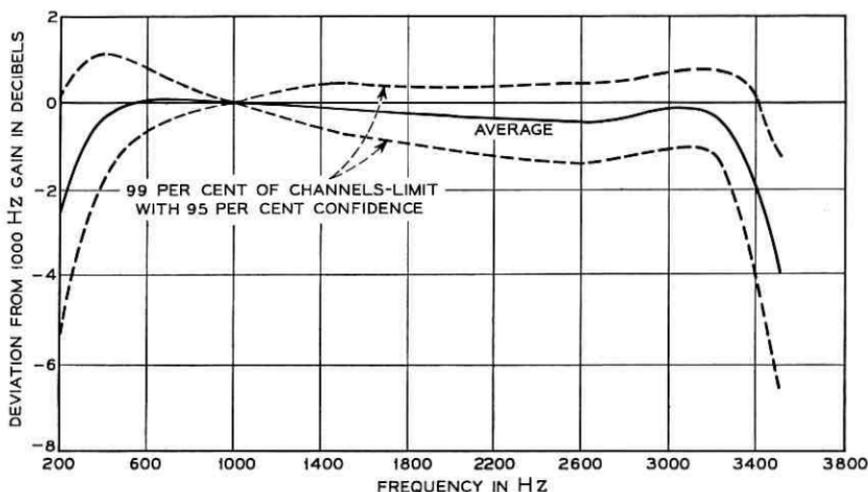
Fig. 5 — N3 channel VF gain-frequency characteristic.
