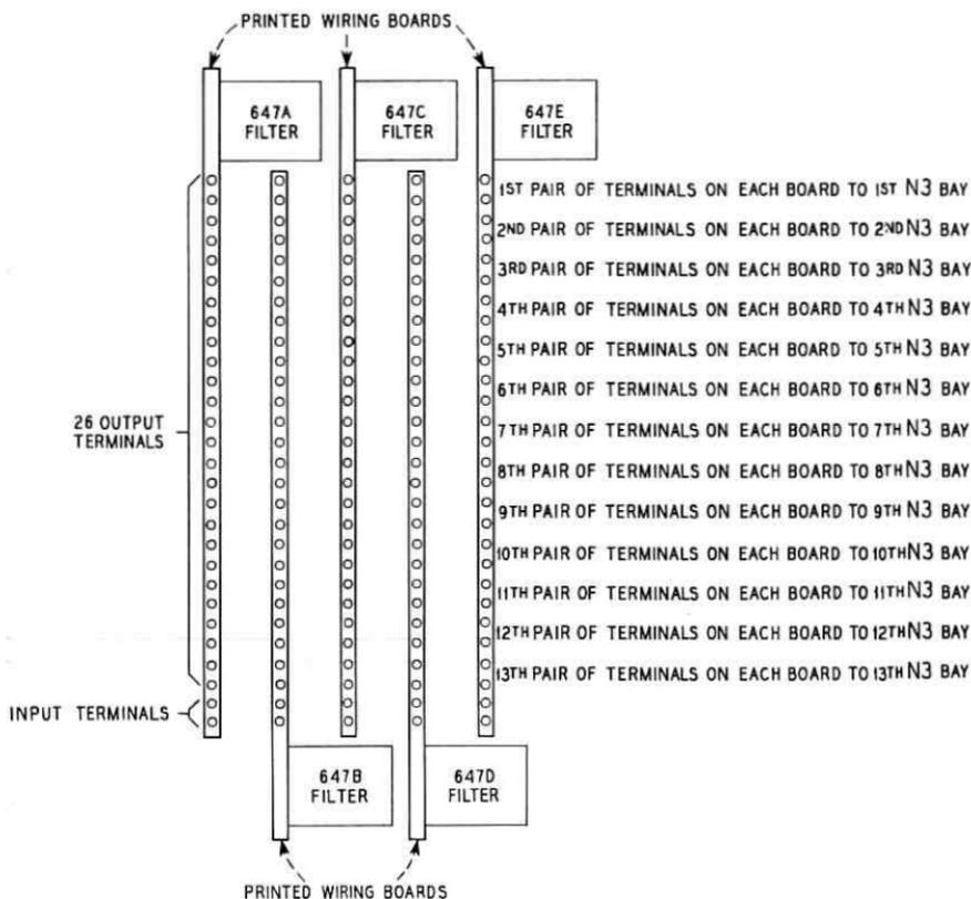
Fig. 27—Section of primary distribution panel showing mechanical interweaving of smoothing filters and terminal assignment.
