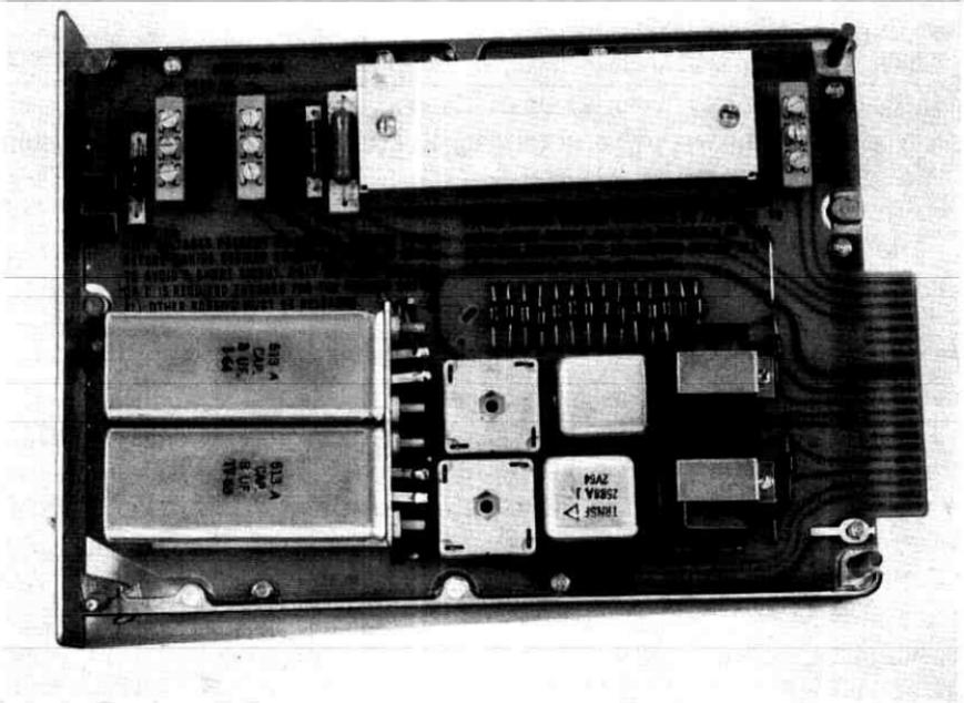
Fig. 17 — Line terminating unit.
