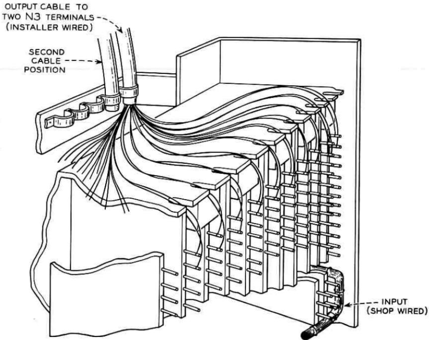
Fig. 28 — Input and output cable connections — primary distribution panel.
