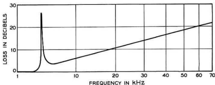
Fig. 6 — Low-pass filter.
