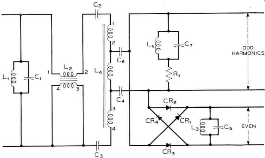
Fig. 23 — Harmonic generator circuit.
