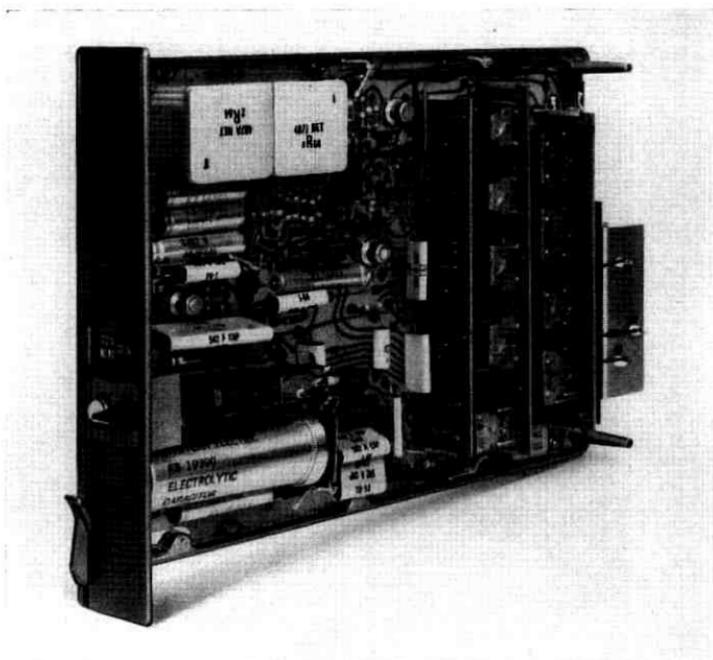
Fig. 14—Alarm and restoral unit.
