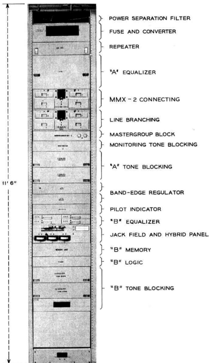
Fig. 45 — Receiving bay equipment arrangement.
