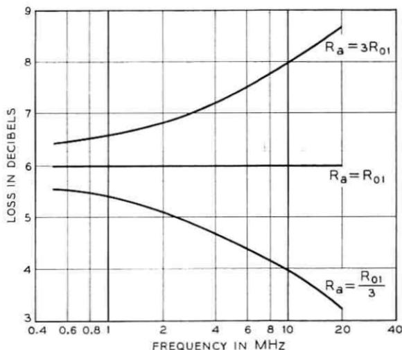
Fig. 25 — Insertion loss characteristic of preregulator network.
