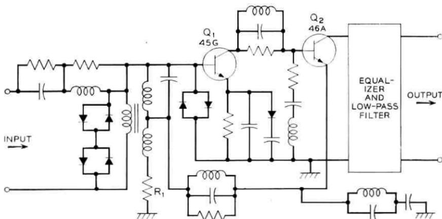
Fig. 6 — Schematic diagram of preamplifier (less bias circuitry).
