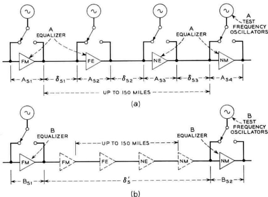
Fig. 7—(a) A equalization; (b) B equalization.
