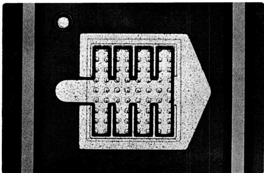
Fig. 3 — The 46E transistor.
