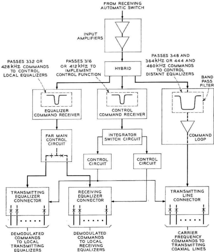
Fig. 5—Loop-back circuit for unattended main station.
