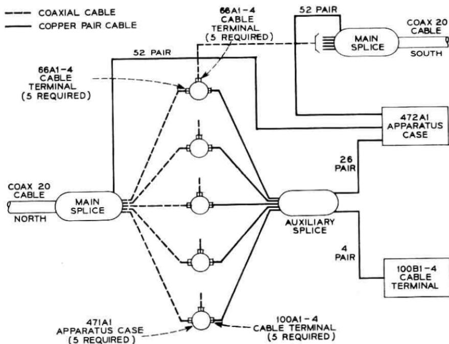
Fig. 13 — L-4 basic station schematic.
