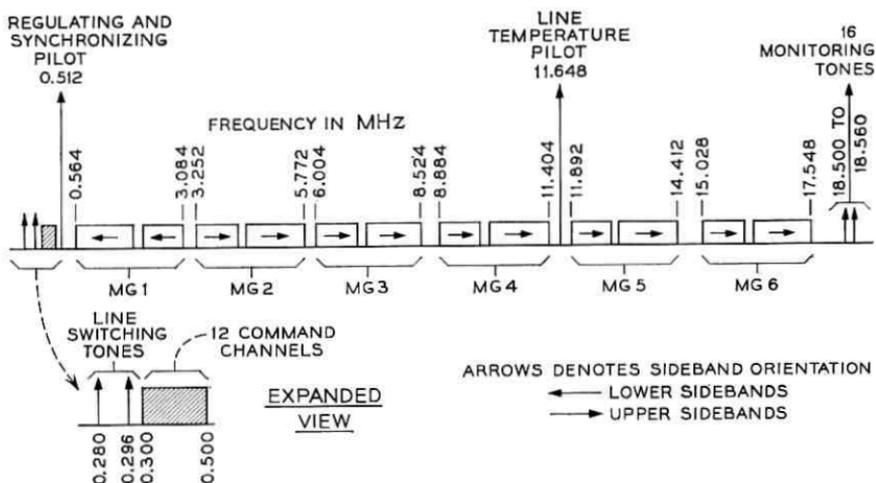
Fig. 1 — L-4 frequency allocations.
