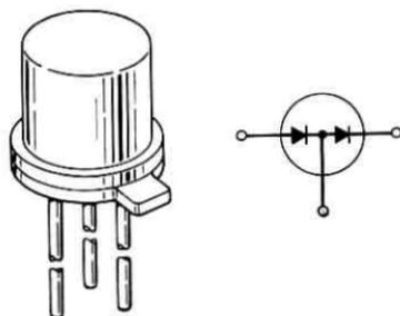
Fig. 6—The device outline for the 459A diode. All dimensions are in inches.
