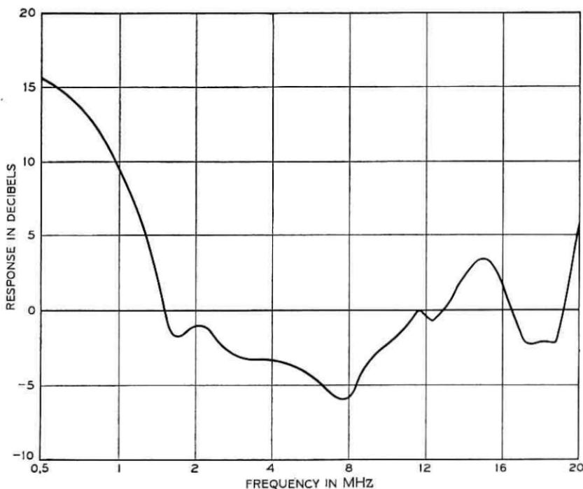
Fig. 50 — Response of L-4 main section before equalizer adjustment.
