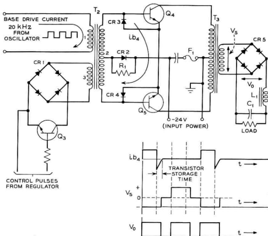
Fig. 3—Power converter simplified schematic.
