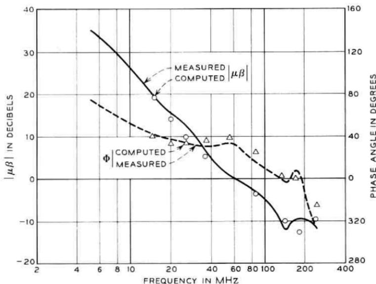
Fig. 7—Typical measured and computed  $\mu\beta$  or loop characteristic of preamplifier.
