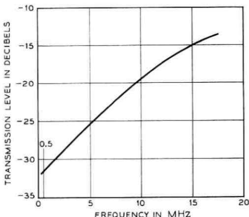
Fig. 5 — Transmission level at repeater output.
