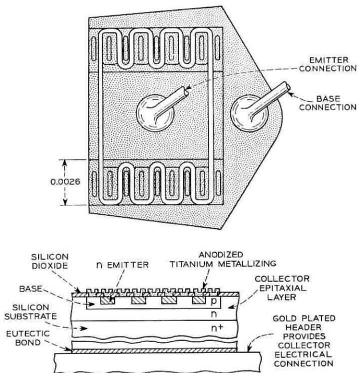
Fig. 1—The 45D transistor.
