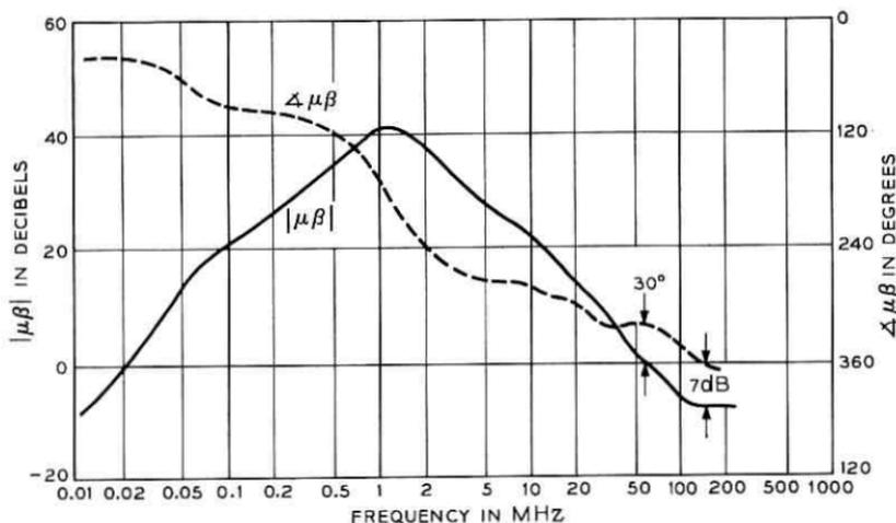
Fig. 28 — Typical  $\mu\beta$ , or loop characteristic, of regulating amplifier.
