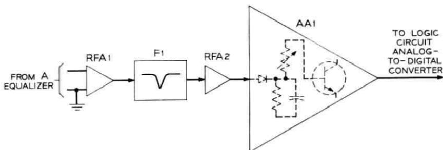
Fig. 19—Block diagram of the command receiver. The amplifier AA1 includes the envelope detector and amplitude control.
