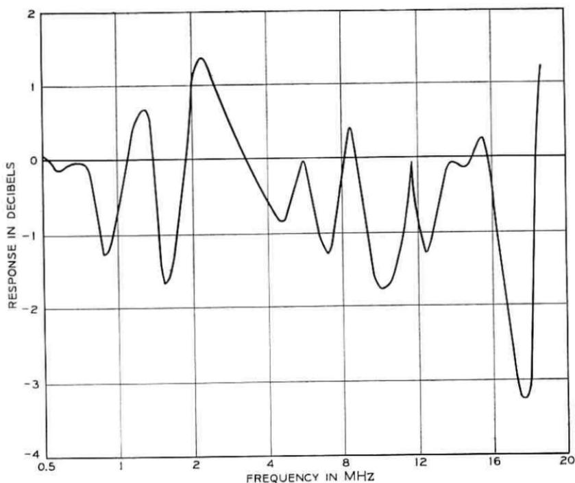
Fig. 51 — Response of L-4 main section after the adjustment of the A equalizers.
