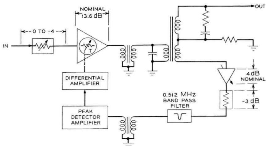
Fig. 36 — Block diagram of the band-edge regulator.
