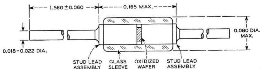
Fig. 7—Mounting and wiring arrangement.
