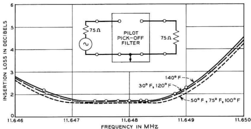
Fig. 33 — Inband temperature performance of pilot pick-off filter.
