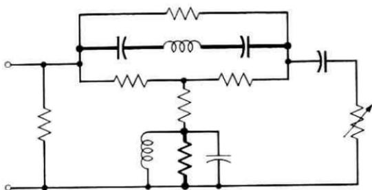
Fig. 32 — High frequency B equalizer Bode network.
