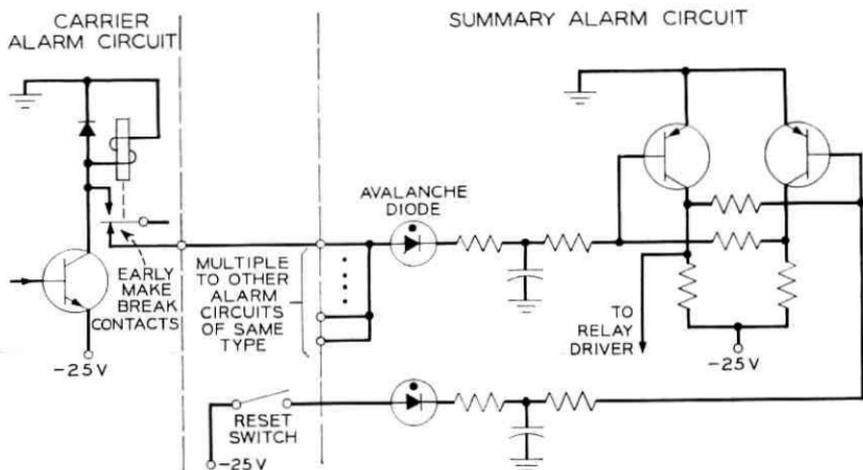
Fig. 9—Typical alarm circuit.
