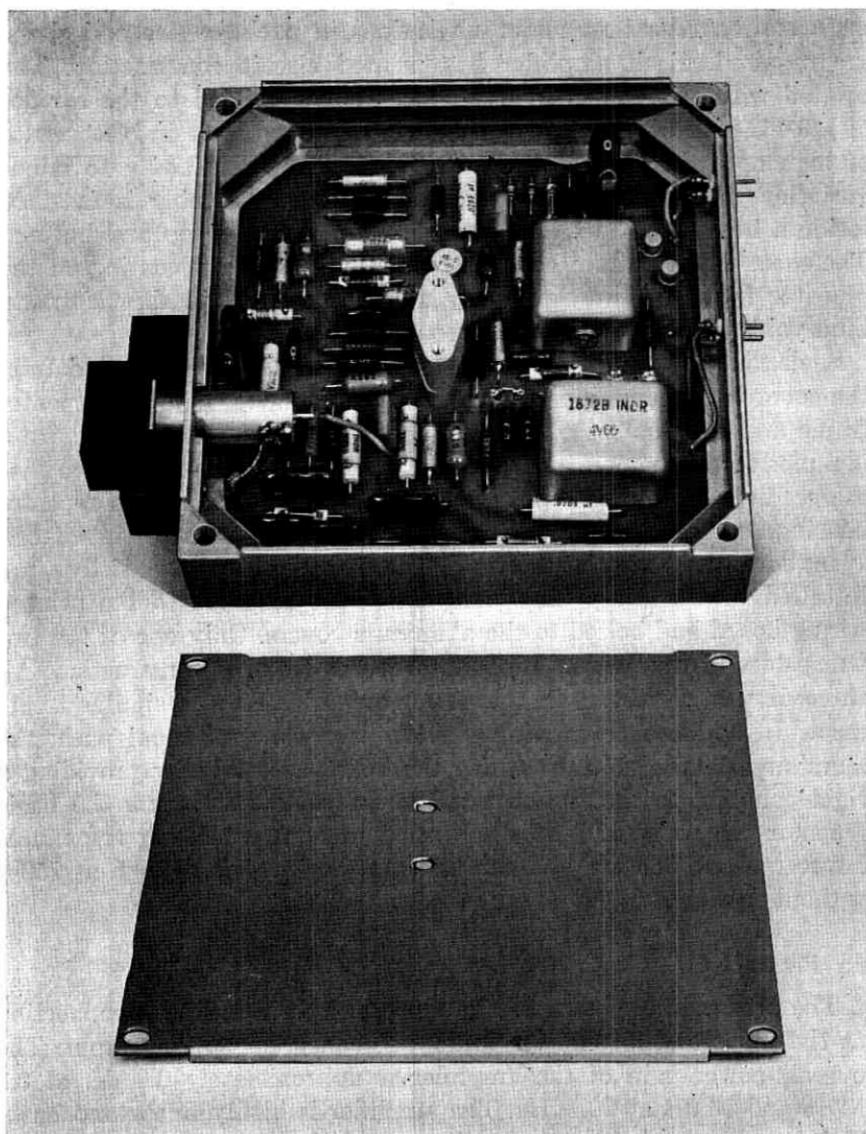
Fig. 4 — Top view of preamplifier with cover removed.
