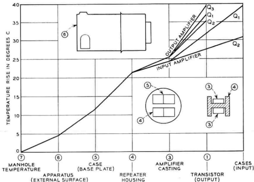
Fig. 5—Temperature gradients for basic repeater installed in a manhole.
