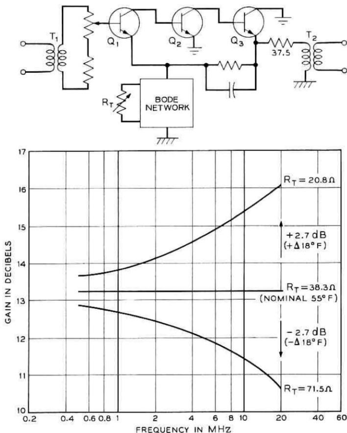
Fig. 30—Performance characteristics of postregulator for a typical cable temperature swing.
