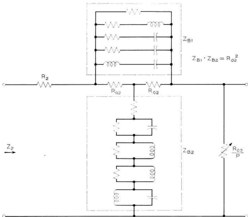
Fig. 29 — Schematic diagram of postregulator network.
