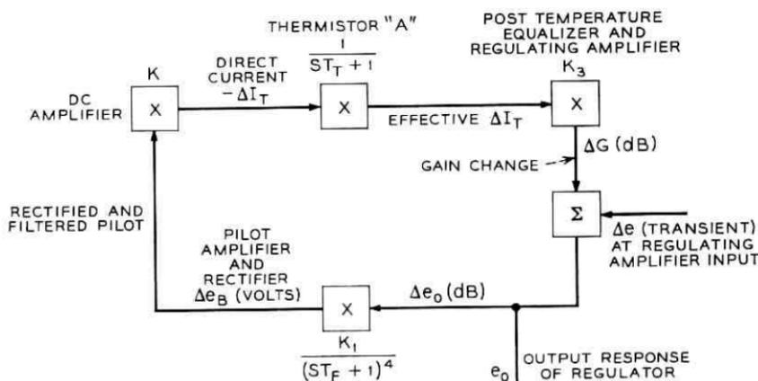
Fig. 35 — Mathematical model of the pilot-controlled postregulator.
