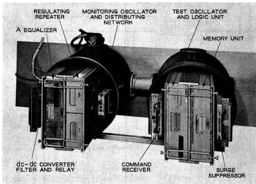
Fig. 24 — Equalizing repeater apparatus case. The left cabinet houses the transmission circuits; the right cabinet houses the remote control circuits.
