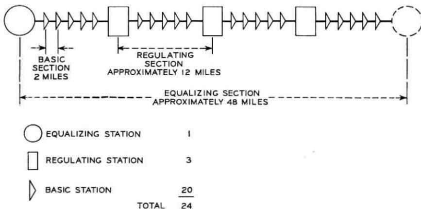
Fig. 12—Equalizing section schematic.
