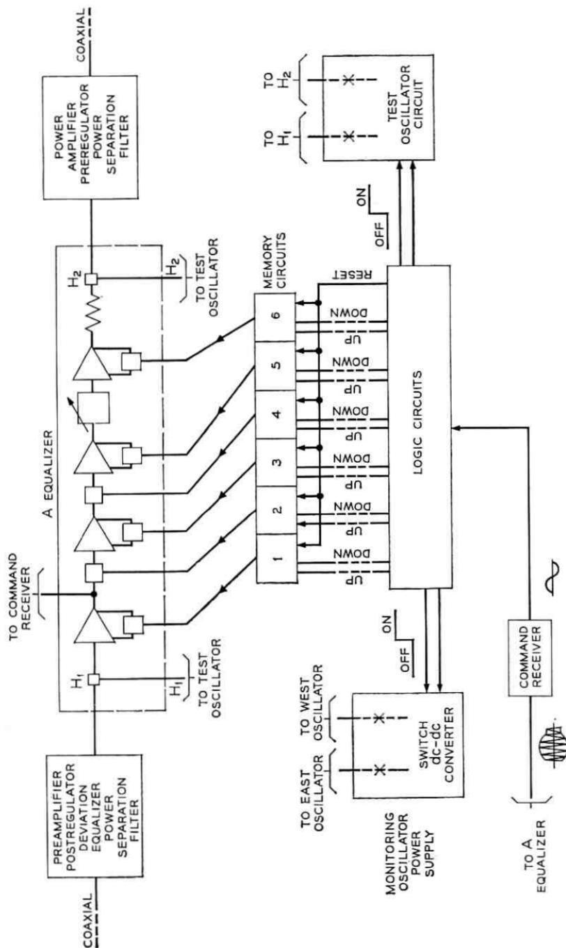
Fig. 1 — Functional block diagram of the equalizing repeater.
