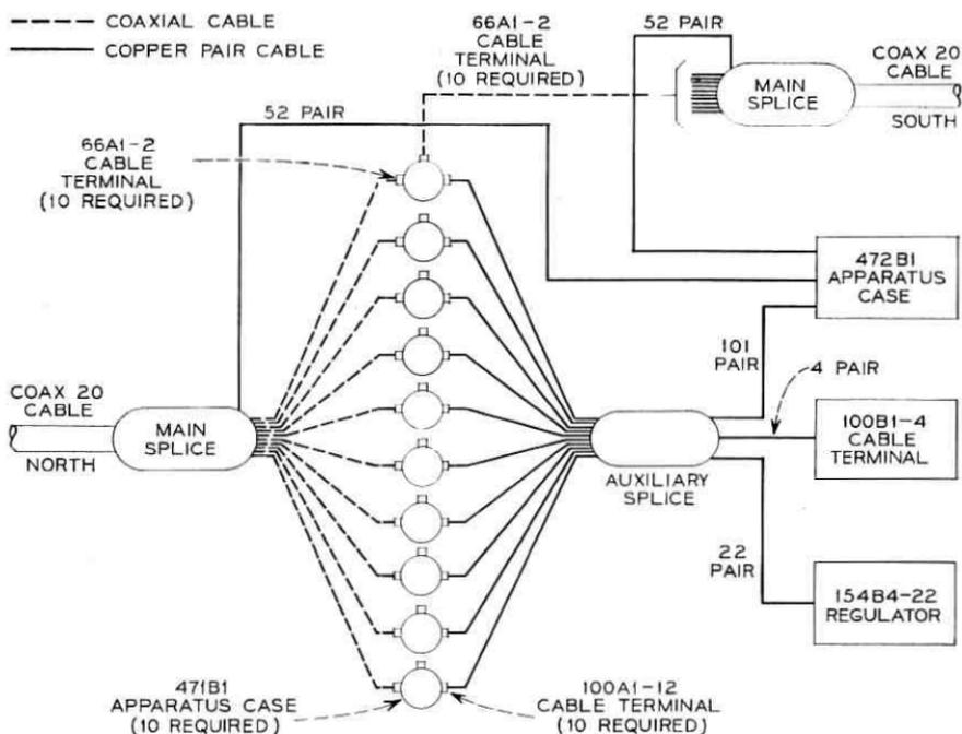
Fig. 14 — L-4 regulating station schematic.
