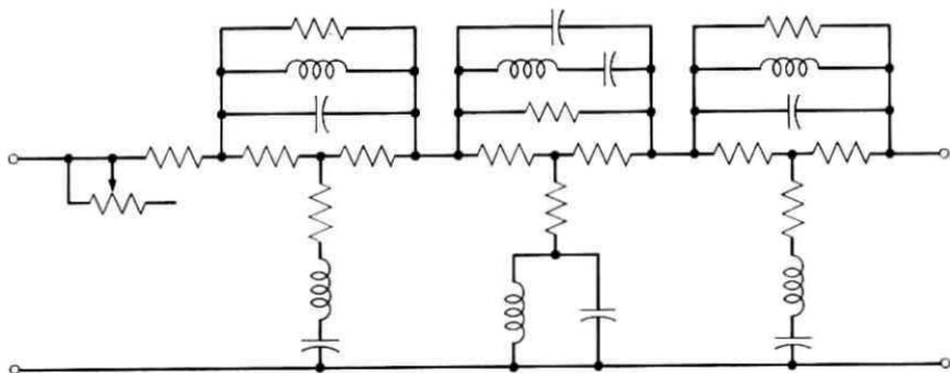
Fig. 18 — Configuration of the A trim equalizer.
