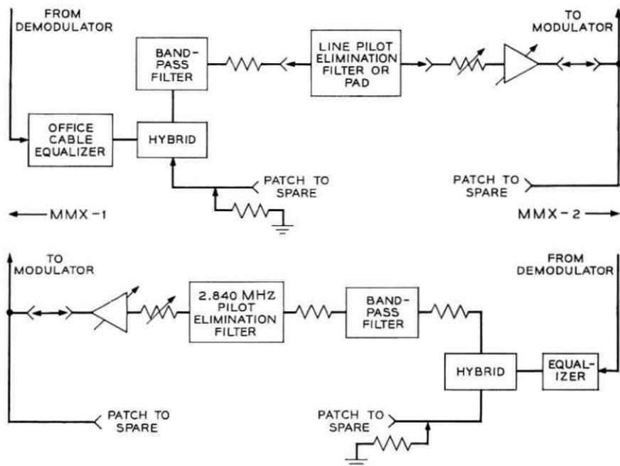
Fig. 20 — Mastergroup connector, MMX-1 to MMX-2 (two-way).
