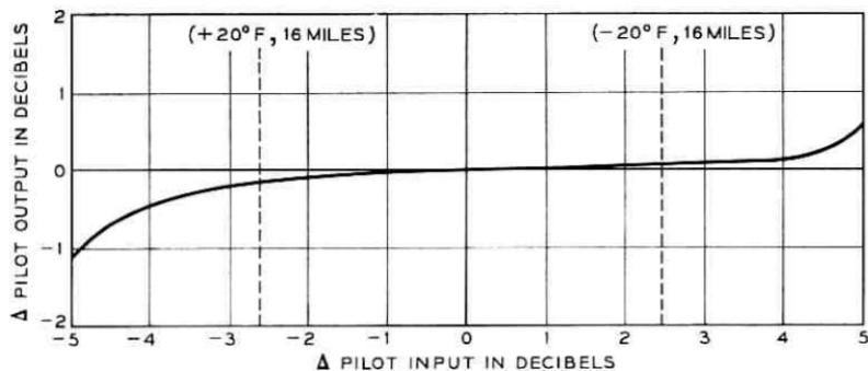
Fig. 37 — Regulating performance of pilot-controlled postregulator.
