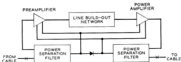
Fig. 1—Simplified block diagram of basic repeater.
