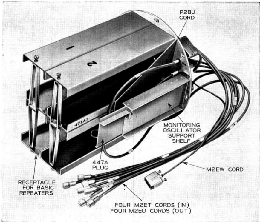
Fig. 19 — Chassis for basic repeaters.
