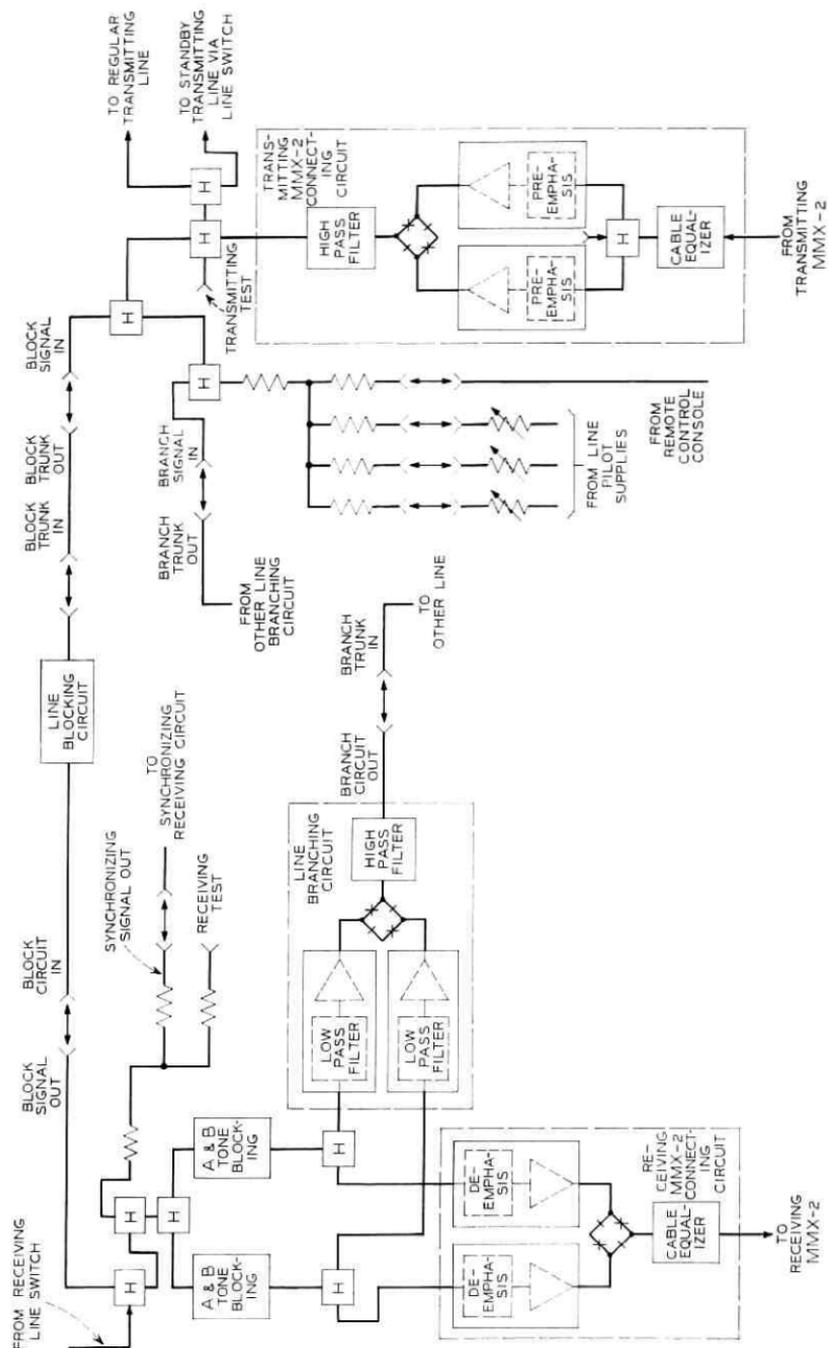
Fig. 16 — Line connecting circuits.
