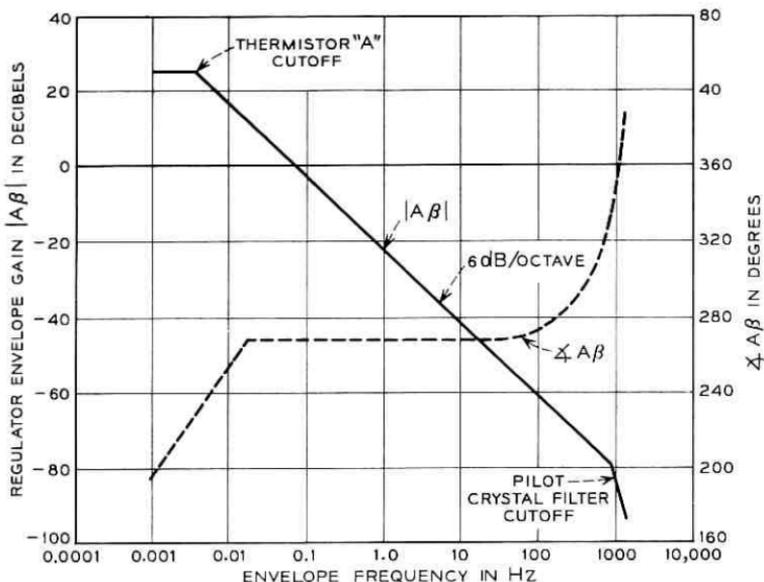
Fig. 36 — Measured postregulator envelope feedback characteristic.
