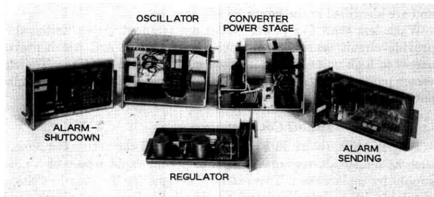
Fig. 8 — Converter plug-in packages.
