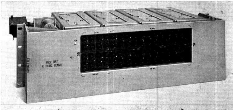
Fig. 41 — Fuse panel and converter assembly.
