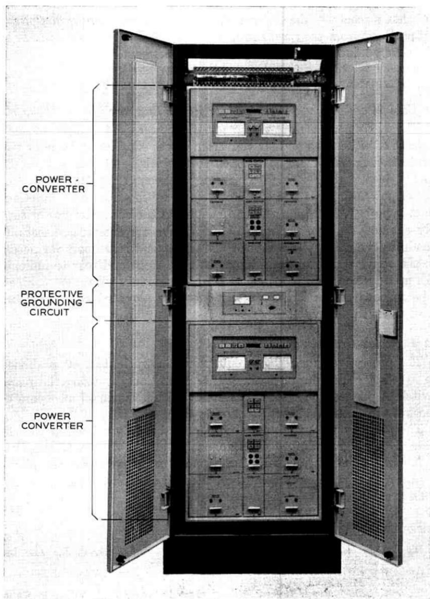
Fig. 10 — Power feed system equipment cabinet.
