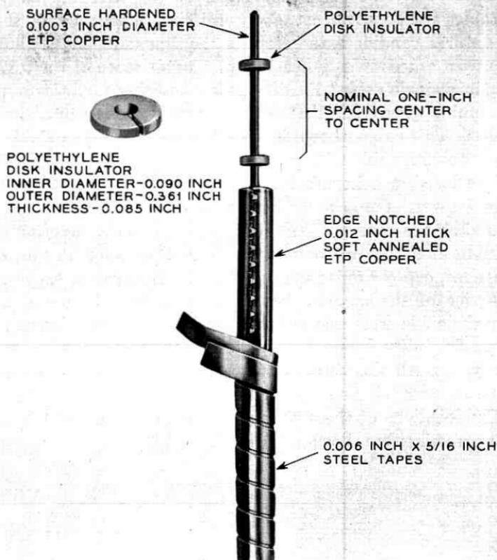
Fig. 1—Air dielectric disk-insulated 0.375 inch serrated-seam coaxial.
