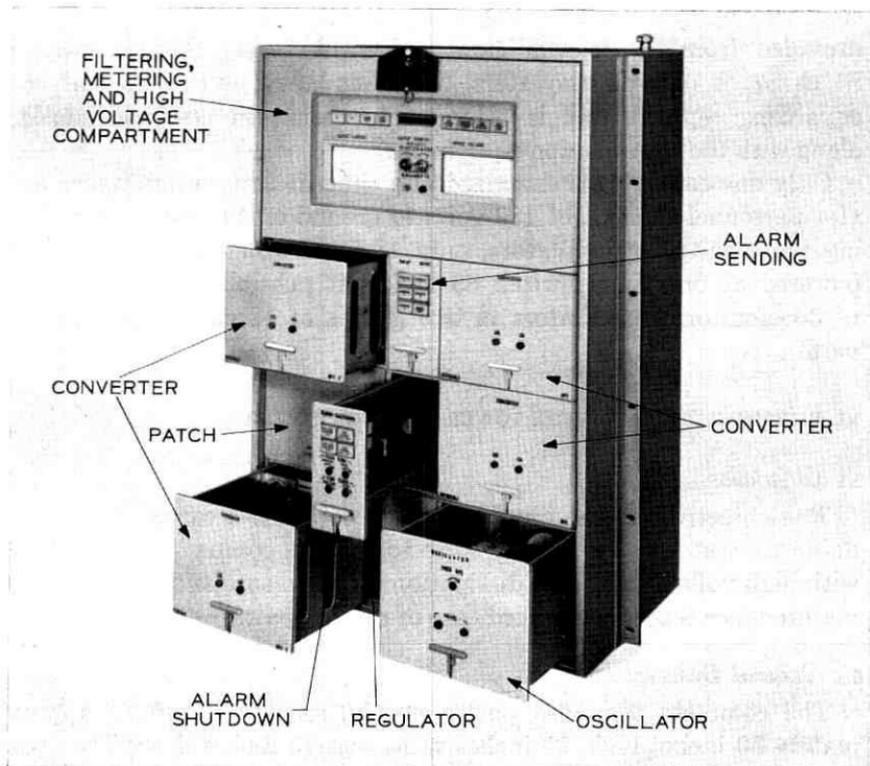
Fig. 7 — Power feed converter: Front view—plug-in units partially removed.
