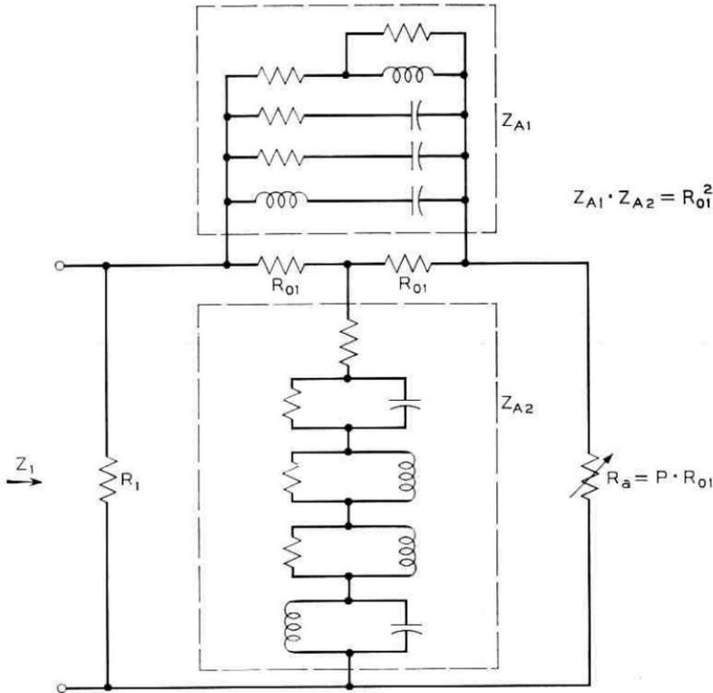
Fig. 24 — Preregulator network configuration.
