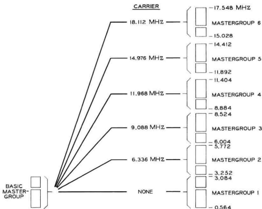
Fig. 1—Six-mastergroup line frequency spectrum.
