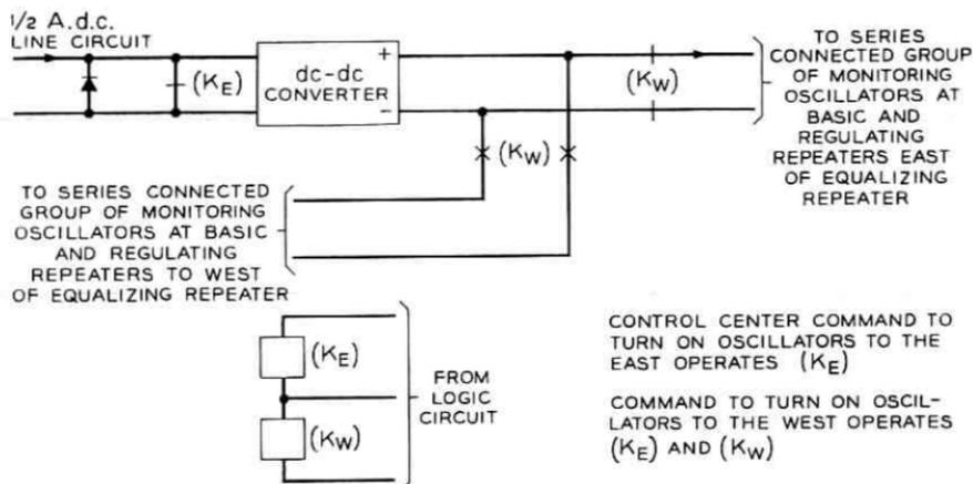
Fig. 23 — Monitoring oscillator power and switching circuit.
