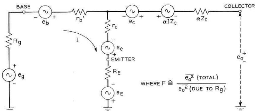
Fig. 10—Equivalent circuit for noise figure calculation of a common emitter stage with series local feedback ( $R_E$ ).
