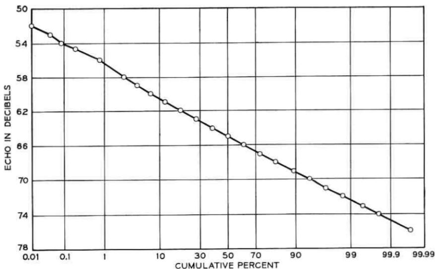
Fig. 4—Distribution of the worst internal echo (out) for 7,520 readings. (Average = 65.62 dB;  $\sigma = 3.48$ )
