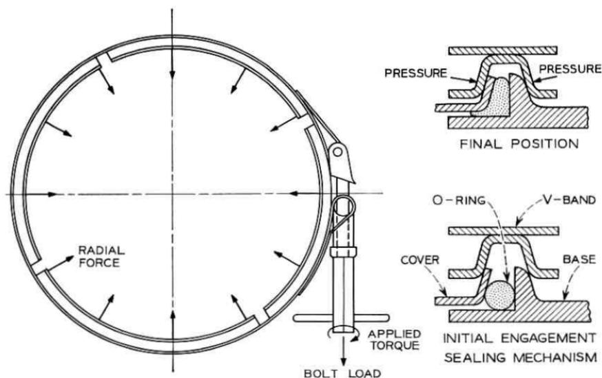
Fig. 18 — The O-ring-V-band sealing mechanism.
