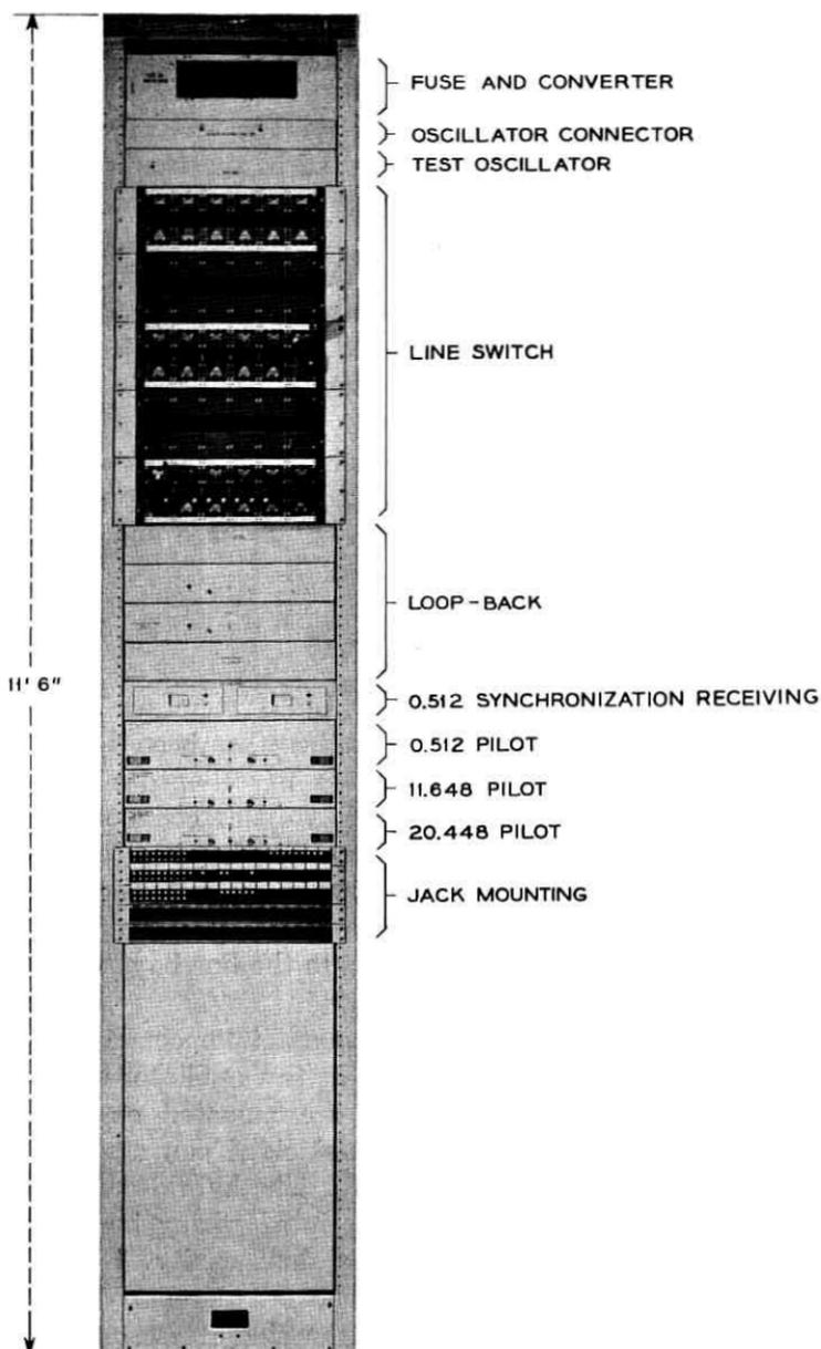
Fig. 48 — Control connecting bay equipment arrangement.
