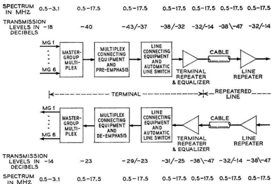
Fig. 6—L-4 transmission levels.
