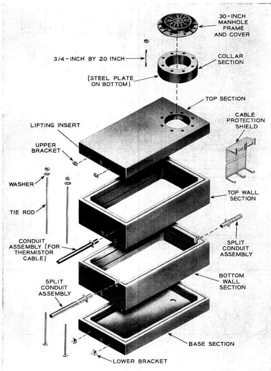
Fig. 16 — G manhole: exploded view.
