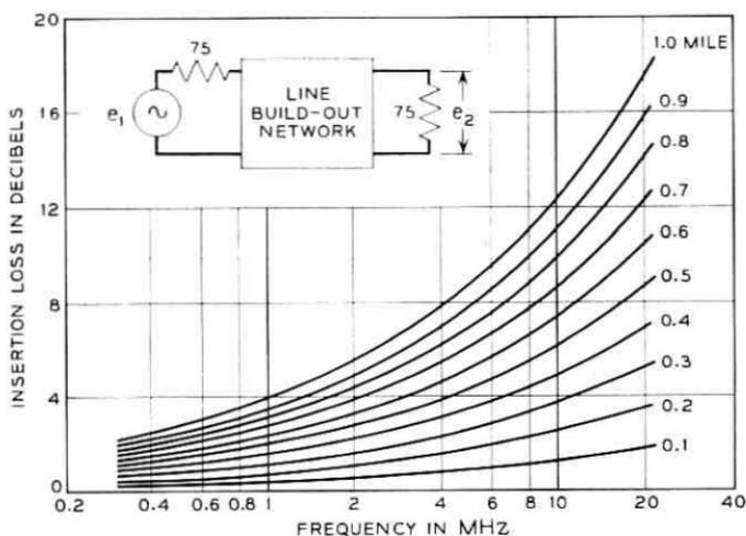
Fig. 14 — Insertion loss characteristics of line build-out networks (0.1 to 1.0 mile).
