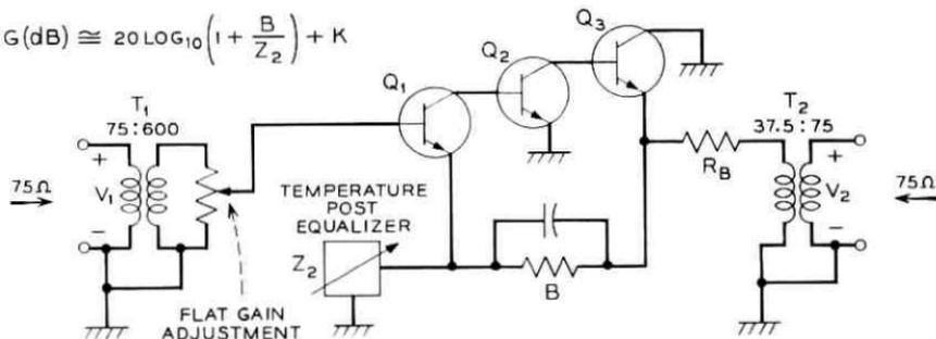
Fig. 27 — Simplified schematic diagram of regulating amplifier.
