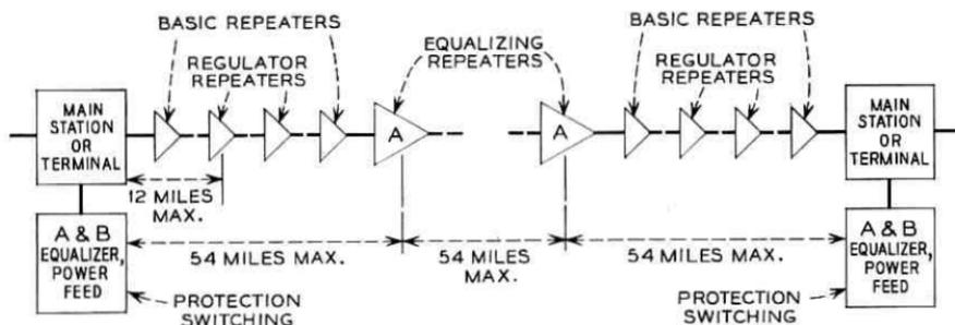
Fig. 2 — Typical L-4 repeatered line layout: maximum distance between main stations is 150 miles.
