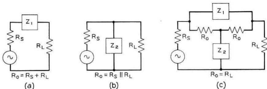
Fig. 12—Basic equalizer network configurations: (a) series, (b) shunt, (c) bridged-T.
