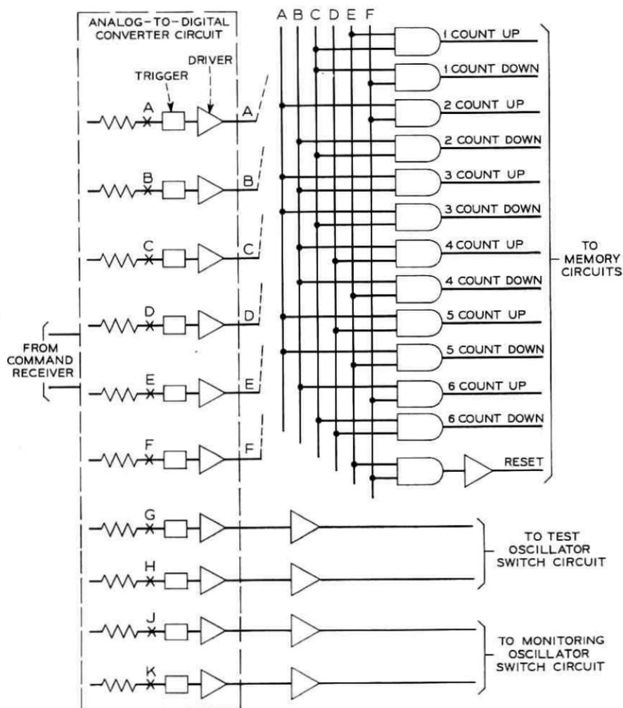
Fig. 20 — Block schematic of the A logic circuits.
