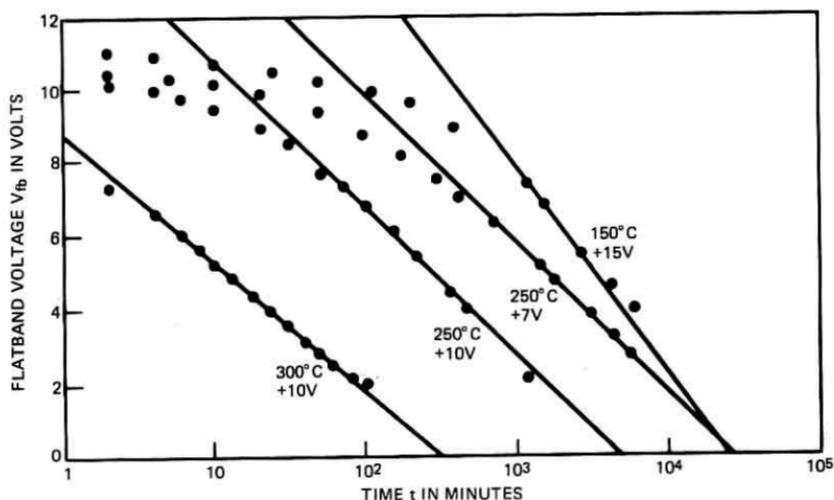
Fig. 4—Experimental results under four different conditions:  $T = 150^\circ\text{C}$ ,  $V_b = 15\text{ V}$ ;  $250^\circ\text{C}$ ,  $7\text{ V}$ ;  $250^\circ\text{C}$ ,  $10\text{ V}$ ;  $300^\circ\text{C}$ ,  $10\text{ V}$ . In each case, the element was charged by setting  $V_b = 50\text{ V}$  for  $100\ \mu\text{s}$ .
