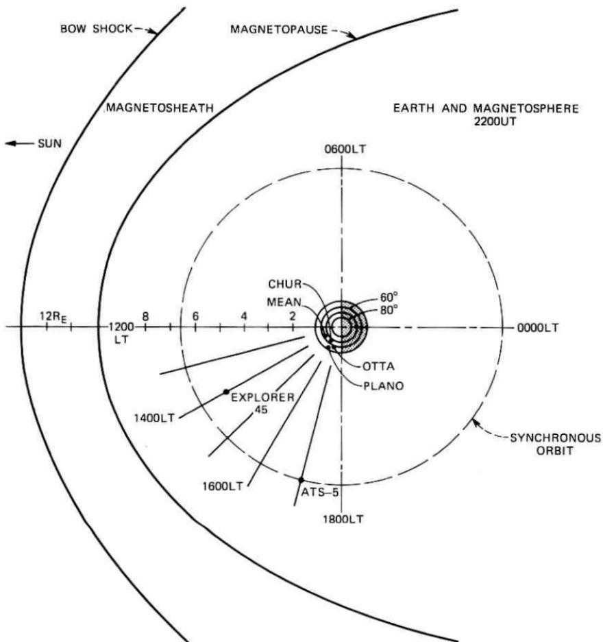
Fig. 1—View of earth and magnetospheric configuration in equatorial plane under normal solar wind flow conditions.
