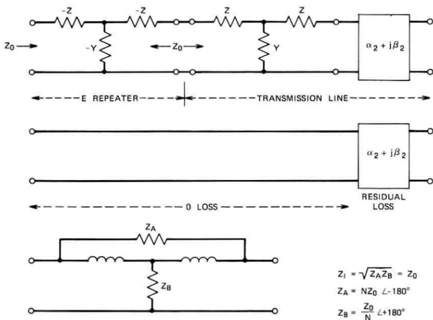
Fig. 21—Equivalent circuits for E-type negative-impedance repeaters.
