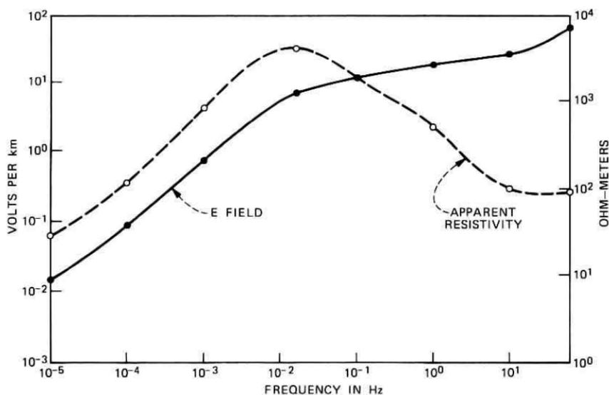
Fig. 7—Variation with frequency of apparent resistivity and surface electric field for the three-layer model of Fig. 6.
