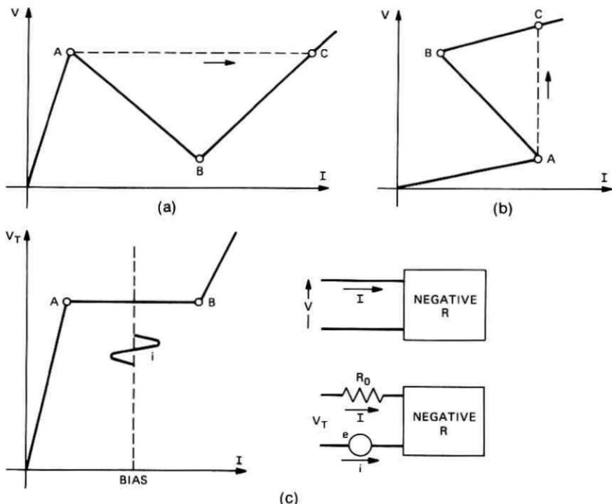
Fig. 2—Voltage-current curves for negative resistance.
