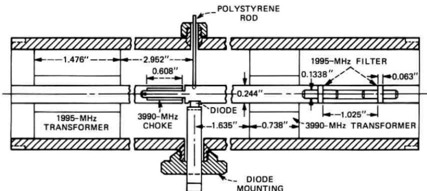
Fig. 1—Cross section of the 1995- to 3990-MHz doubler.
