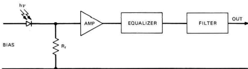
Fig. 1—Typical input circuit of an optical repeater.
