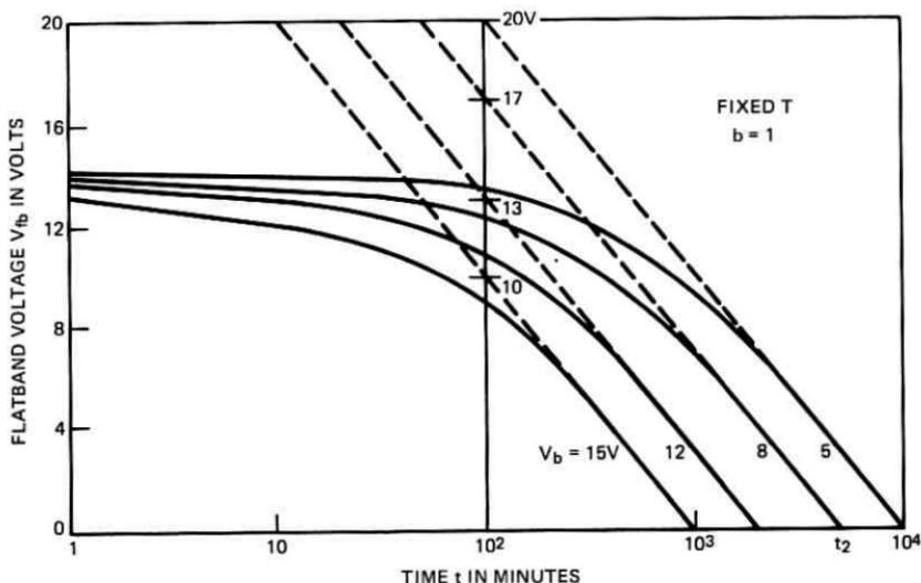
Fig. 2—Schematic illustrating a possible decay of the flatband voltage  $V_{fb}(t)$  as a function of  $\log_{10} (t/t_1)$  in a hypothetical device for four different applied biases  $V_b$  at a fixed temperature  $T$ . For simplicity, we set  $b = 1$ . Also shown are the envelope functions  $V_e(t)$  associated with each  $V_b$ .
