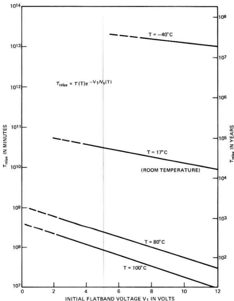
Fig. 6—The predicted roll-off or device relaxation time for zero-applied bias ( $V_b = 0$ ) and temperatures of  $-40^\circ\text{C}$ ,  $17^\circ\text{C}$ ,  $80^\circ\text{C}$ , and  $100^\circ\text{C}$  plotted as a function of "initial" flatband voltage  $V_1 = V(t_1)$ , where  $t_1 = 1$  minute.
