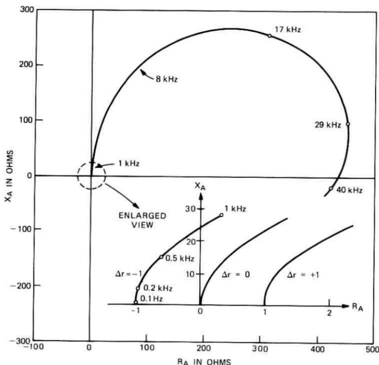
Fig. 13—Reactance vs resistance plot of impedance  $Z_A$  as frequency varies.  $Z_L$  is impedance of a pair of NIB units and  $Z_{sc}$  is the open circuit impedance of a half section of uniform line.
