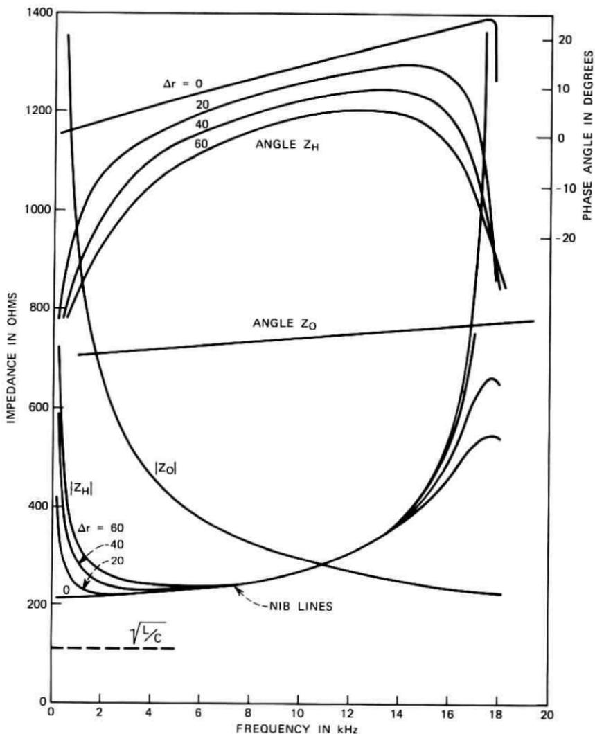
Fig. 6—Image impedance vs. frequency for a 26-gauge NIB line with 6000-foot booster spacing. Parameter  $\Delta r$  is the net resistance at very low frequencies per section of NIB line. The characteristic impedance  $Z_o$  of the line before the insertion of NIB units is also shown.
