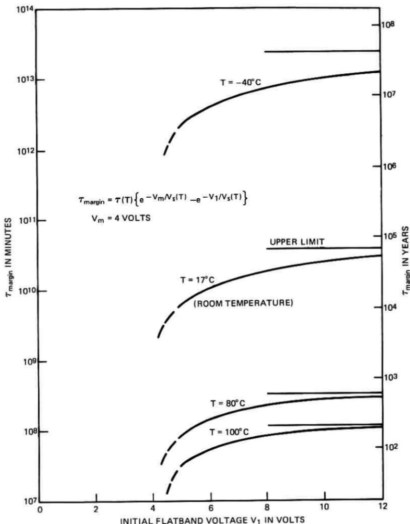
Fig. 7—The predicted margin time for zero-applied bias ( $V_b = 0$ ) and temperatures of  $-40^\circ\text{C}$ ,  $17^\circ\text{C}$ ,  $80^\circ\text{C}$ , and  $100^\circ\text{C}$  plotted as a function of "initial" flatband voltage  $V_1 = V(t)$ , where  $t_1 = 1$  minute. The horizontal line above each curve is the upper limit for  $\tau_{margin}$  as  $V_1$  is taken larger and larger.
