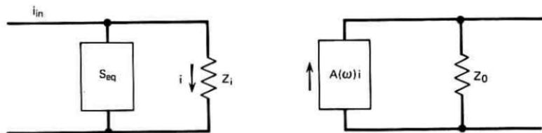
Fig. 3—Equivalent noise circuit.
