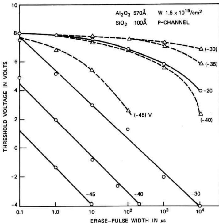
Fig. 6—Shifts in threshold voltage, initially at 8 V, after application of negative-gate-voltage pulses to p-channel IGFETs with dual-dielectric gate insulation consisting of 100-Å-thick SiO<sub>2</sub> and 570-Å-thick Al<sub>2</sub>O<sub>3</sub>. Solid lines apply to structures containing  $1.5 \times 10^{15}/\text{cm}^2$  of W at dual-dielectric interface; dashed lines apply to structures with no interfacial dopant.
