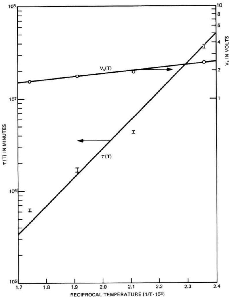
Fig. 5—Experimentally determined parameters  $\tau$  and  $V_s$  plotted versus  $1/T$  to determine the activation energies  $E_a$  and  $E_s$ .
