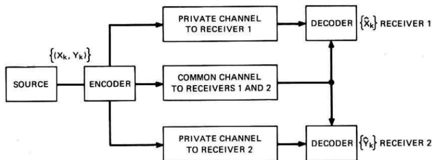
Fig. 2—Source coding for a network.
