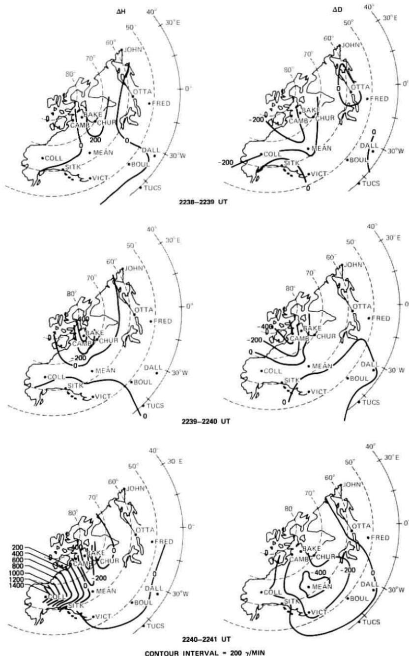
Fig. 3a—Minute-by-minute rate of change of magnetic field in the horizontal plane over North America from 2238 to 2241 UT.
