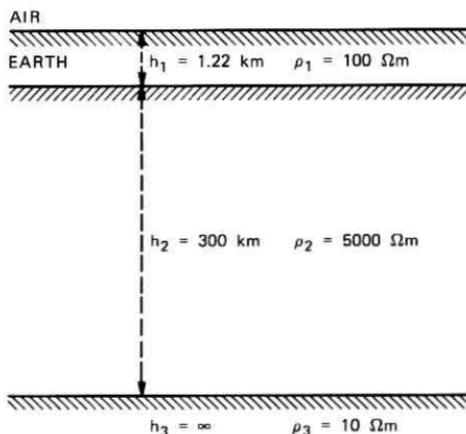
Fig. 6—Three-layer resistivity model for Plano, Illinois, vicinity.
