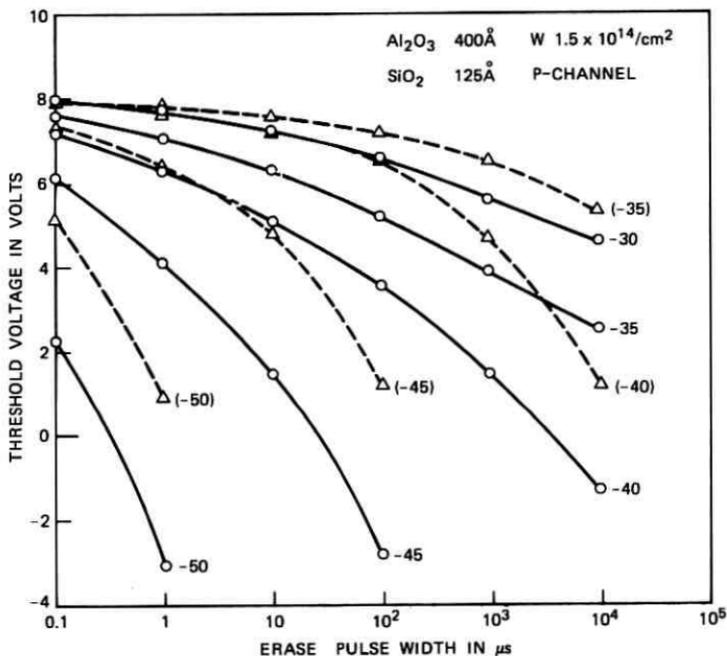
Fig. 8—Shifts in threshold voltage, initially at 8 V, after application of negative-gate-voltage pulses in p-channel IGFETs with dual-dielectric gate insulation of 125-Å-thick  $\text{SiO}_2$ , 400-Å-thick  $\text{Al}_2\text{O}_3$ . Solid lines apply to structure with  $1.5 \times 10^{14}/\text{cm}^2$  of  $W$  at dual-dielectric interface; dashed lines apply to structures with no interfacial dopant.
