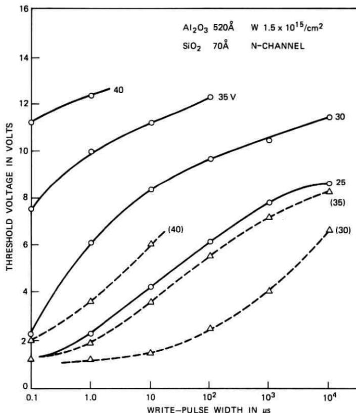
Fig. 3—Shifts in threshold voltage in n-channel IGFETs with dual-dielectric gate insulation consisting of 70-Å-thick SiO<sub>2</sub> and 520-Å-thick Al<sub>2</sub>O<sub>3</sub> after application of positive-gate-voltage pulses. Solid lines apply to structures containing 1.5 × 10<sup>15</sup>/cm<sup>2</sup> of W at dual-dielectric interface; dashed lines apply to structures with no interfacial dopant. The initial threshold voltages were at 1 volt.
