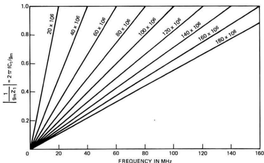
Fig. 9—Reciprocal gain vs frequency with gain bandwidth product ( $g_m/2\pi C_t$ ) as a parameter.
