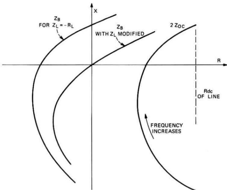
Fig. 15—Reactance vs resistance plots of  $Z_B$  and  $Z_{oc}$ .
