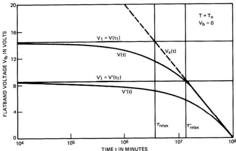
Fig. 3—Schematic illustrating a possible decay of the flatband voltage  $V(t)$  in a hypothetical device for room temperature ( $T = T_o$ ) and zero applied bias ( $V_b = 0$ ) for two different quantities of stored charge,  $V_1$  and  $V'_1$ . The size of the characteristic relaxation time  $\tau_{relax}$  is indicated for both cases. Note that  $V_1 - V_1^o = V'_1 - V_1^o = 0.69 V_s$ .
