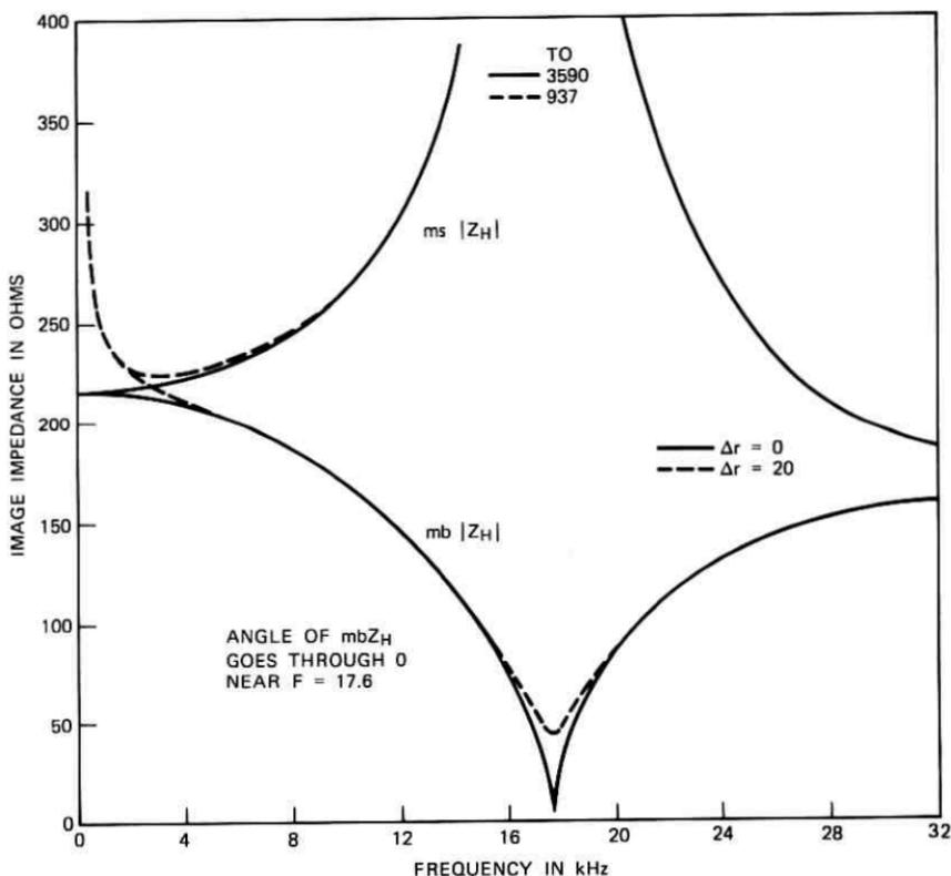
Fig. 12—The two image impedances  $Z_H$  of a NIB line.
