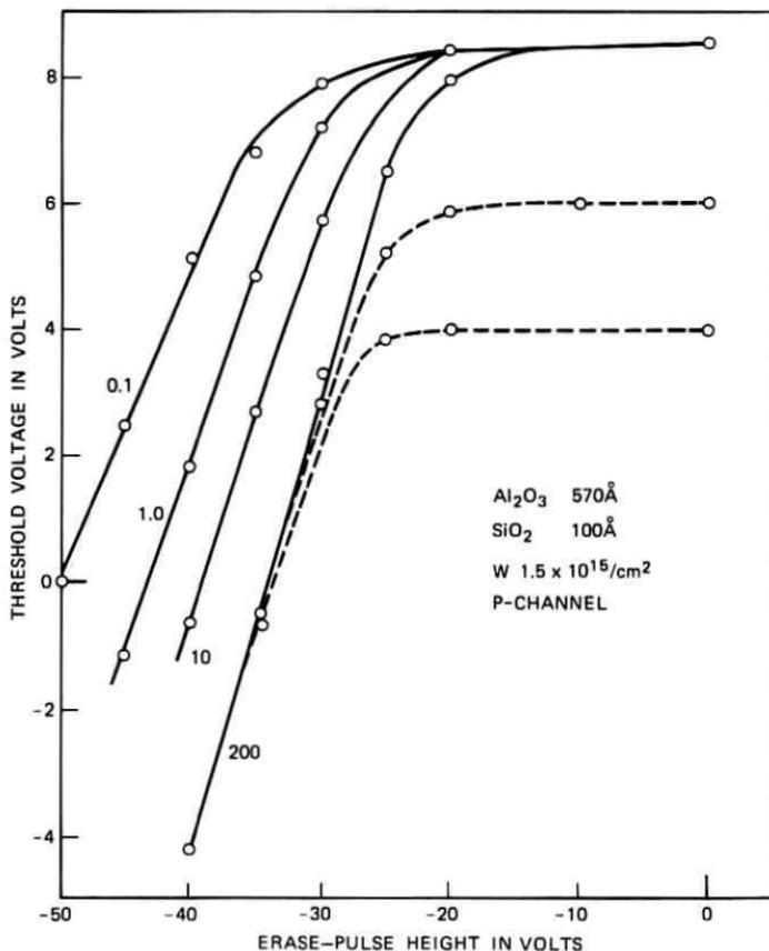
Fig. 7—Shifts in threshold voltages, initially at three different values, in IGFETs described in Fig. 4 after application of negative-gate-voltage pulses of 200- $\mu\text{s}$  duration and various pulse heights. Also shown are shifts in threshold voltages, initially at 8 V, after application of pulses of 10  $\mu\text{s}$ , 1.0  $\mu\text{s}$ , and 0.1  $\mu\text{s}$  in duration.
