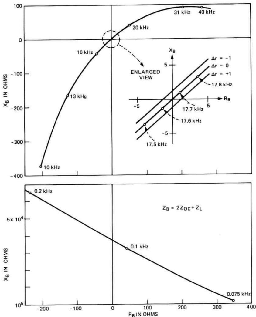
Fig. 14—Reactance vs resistance plot of impedance  $Z_B$  in which  $Z_{oc}$  is the open-circuit impedance of a half section of uniform line.
