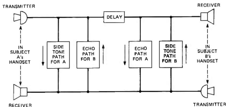
Fig. 11—Test system for the 1970 laboratory echo test.
