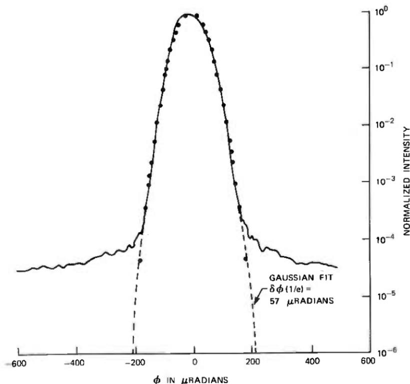
Fig. 16—Observed instrumental profile as measured by a tangential direction scan in the instrument's sagittal focal plane. The heavy dots and dashed curve are a best fit to the function  $\exp[-\varphi^2/\delta\varphi^2(1/e)]$ .
