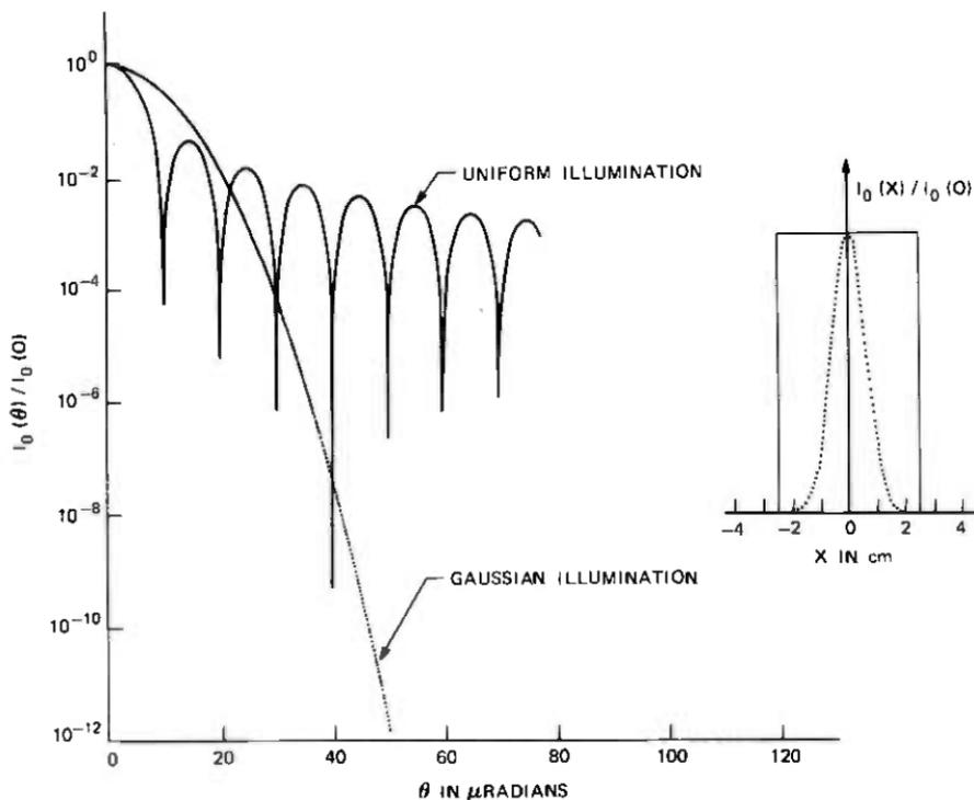
Fig. 8—Calculated instrumental profiles for uniform and gaussian illumination with  $b = 5.0$  cm and  $\sigma = 0.826$  cm. The  $b$  value corresponds to the maximum clear aperture of the MK VI instrument, while the  $\sigma$  value corresponds to the width of the gaussian illumination actually used in the present apparatus. Normalized illumination functions for each case are shown inset on a linear intensity scale.
