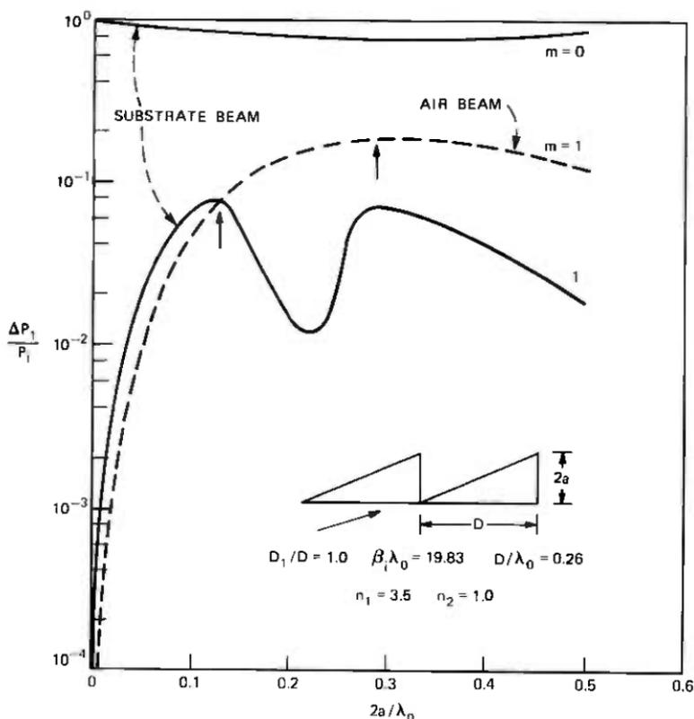
Fig. 10—Normalized scattered power into air (dotted line) and substrate (solid lines) for a grating with  $n_1 = 3.5$ ,  $n_2 = 1.0$ ,  $D/\lambda_0 = 0.26$ ,  $D_1/D = 1.0$ , and  $\beta_1\lambda_0 = 19.83$ . The arrows indicate the position of points where specular reflection from the grating teeth coincides with the grating condition.
