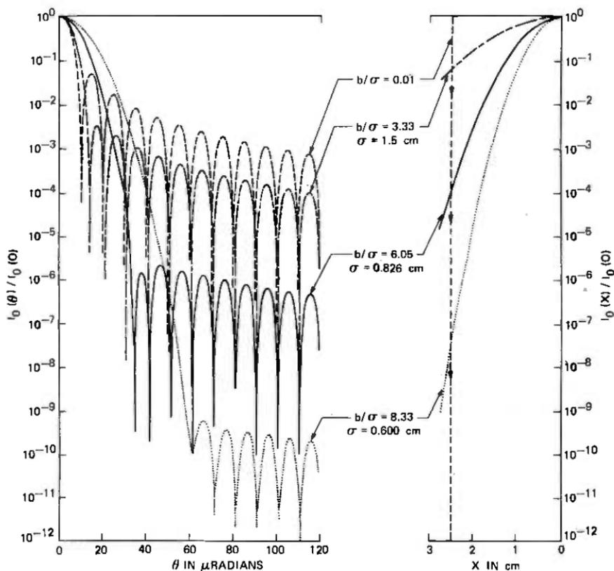
Fig. 9—Calculated instrumental profiles for truncated gaussian illumination and various values of  $(b/\sigma)$ . Also shown, on a logarithmic intensity scale, are the corresponding normalized illumination functions  $[I_0(x)/I_0(0)]$ . The curves labelled  $(b/\sigma) = 6.05$  are appropriate to the  $b$  and  $\sigma$  values used in the present apparatus.
