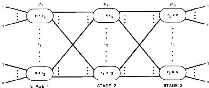
Fig. 1—Generalized three-step Clos network.
