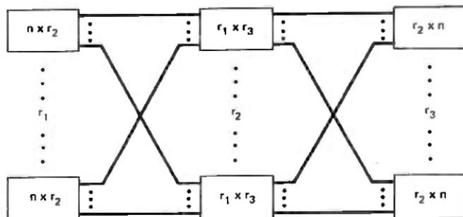
Fig. 2—Ordinary three-stage Clos network.
