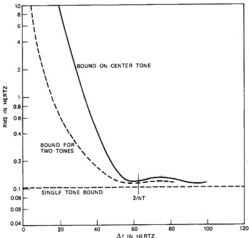
Fig. 1—Frequency estimation bound vs  $\Delta f$  for center of three equally spaced complex tones with worst relative phase and 20 dB s/n.  $N$  is 128.  $1/T$  is 4000 Hz. Corresponding single and double tone bounds also shown.
