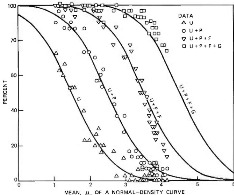
Fig. 16—1968 laboratory echo data percentages (noise = 28 dBnC) as a function of the Step 3 normal-density means compared with percentages predicted using the echo standard deviation, 0.888.
