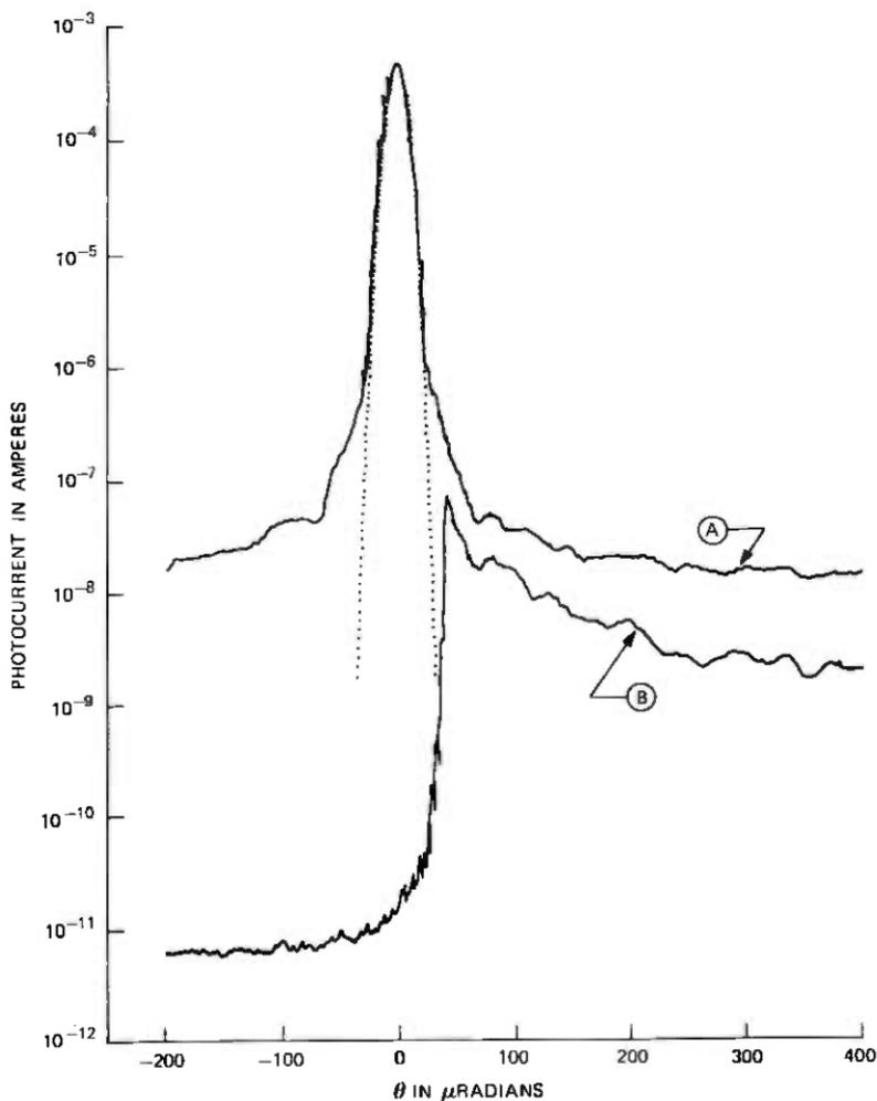
Fig. 4—Measured instrumental profiles for the MK VI apparatus in the region around  $\theta = 0$ . Curve B was obtained with the knife-edge,  $KE$ , occulting the direct beam, while curve A was measured with  $KE$  retracted. Dotted curve is best fit of the function  $\exp[-\theta^2/\delta\theta^2(1/e)]$  to the transmitted beam profile.
