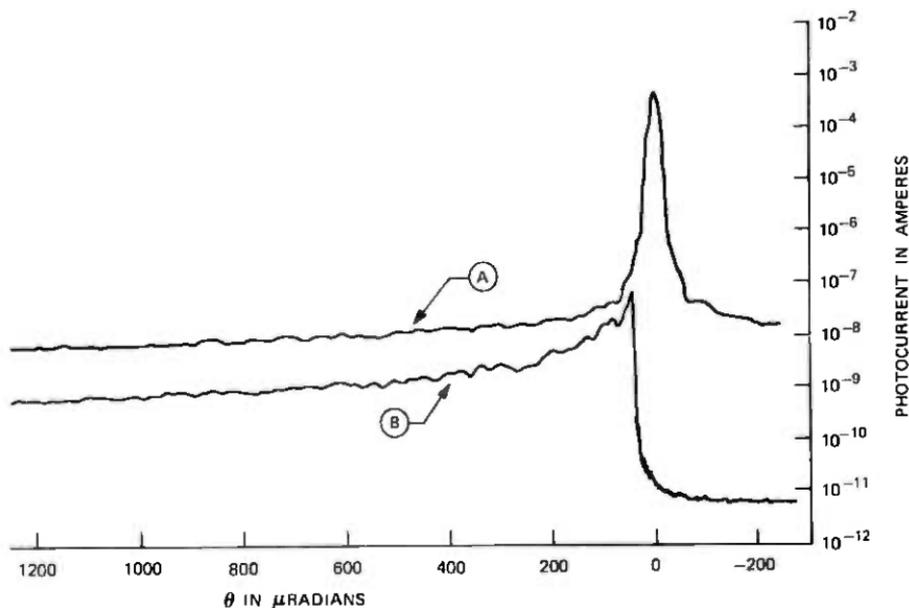
Fig. 3—Observed instrumental profiles for the MK VI apparatus plotted on a logarithmic intensity scale. Curve B was obtained with the knife-edge,  $KE$ , occulting the direct beam, while curve A was measured with  $KE$  retracted.
