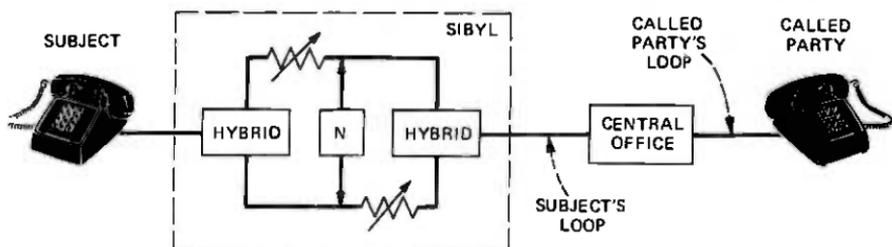
Fig. 8—Diagram of a telephone connection for the SIBYL tests.
