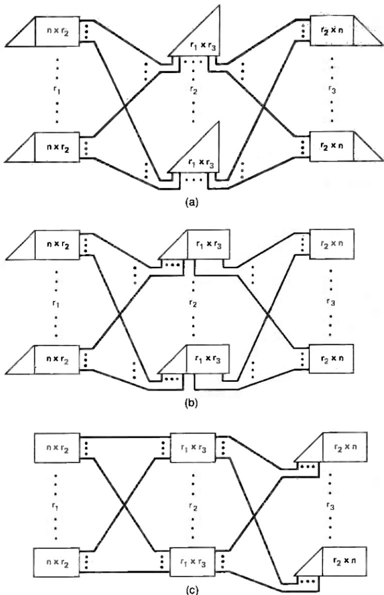
Fig. 3—Mixed three-stage Clos networks.
