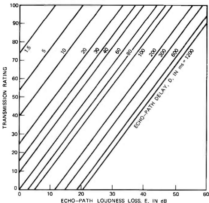
Fig. 2—Transmission rating for talker echo.
