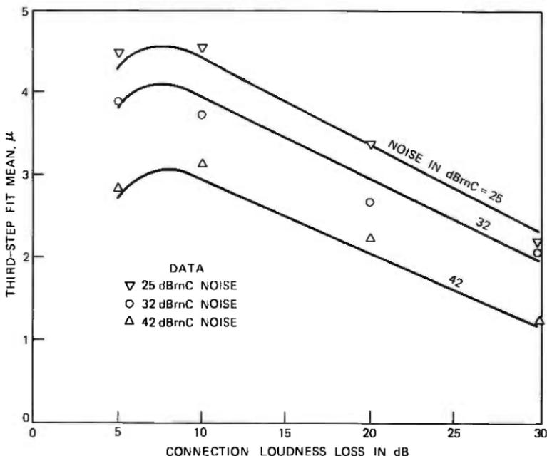
Fig. 23—HO2 loss-noise test, Step 3 means from data as a function of loudness loss and noise compared with means predicted from the loss-noise model at the HO2 base.
