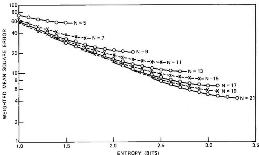
Fig. 4—Quantizer performance for Laplacian density and exponential weighting. Quantization noise is weighted by  $1/|\beta| \exp(-\beta|x|)$ , whereas the probability density is taken to be  $1/|\alpha| \exp(-\alpha|x|)$ . Such situations arise in quantization of the prediction errors in predictive coding of the television signals:  $\alpha = 0.1, \beta = 0.065$ .
