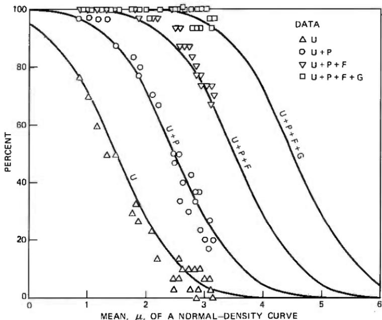
Fig. 17—1968 laboratory echo data percentages (noise=38 dBmC) as a function of the Step 3 normal-density means compared with percentages predicted using the echo standard deviation, 0.888.
