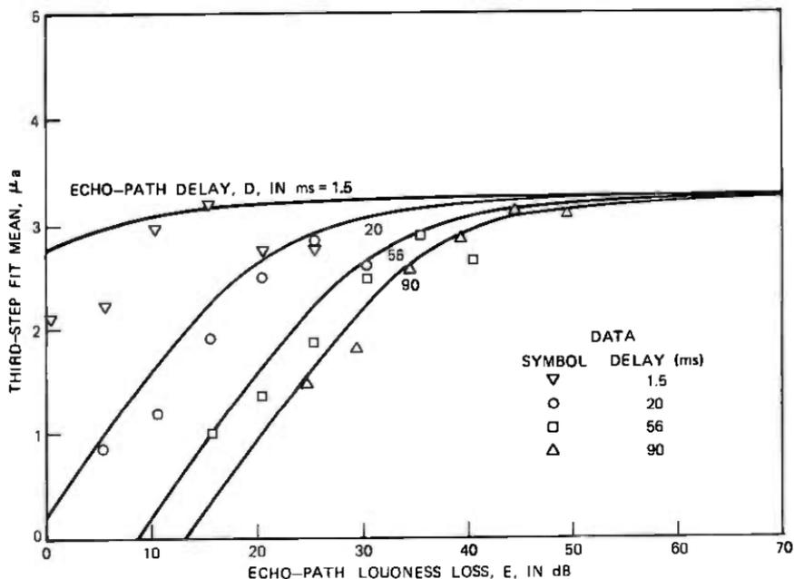
Fig. 26—1968 laboratory echo test (noise=38 dB<sub>rnc</sub>, loss=10 dB) Step 3 means from data as a function of echo-path loss and delay compared with means predicted from the loss-noise-echo model at the echo 1 base.
