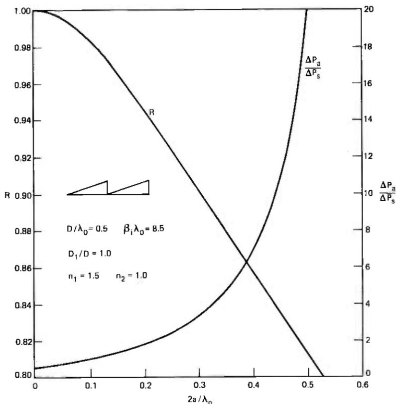
Fig. 9—Ratio of the powers  $\Delta P_a/\Delta P_s$  that are scattered into air and substrate and also the power reflection coefficient  $R$  of the zero-order beam in the substrate as functions of the normalized grating depth  $2a/\lambda_0$ . It is  $D/\lambda_0 = 0.5$ ,  $\beta_1\lambda_0 = 8.5$ ,  $D_1/D = 1.0$ ,  $n_1 = 1.5$ , and  $n_2 = 1.0$ .
