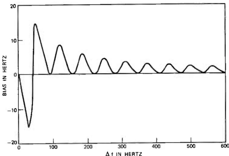
Fig. 4—Bias in peak frequency of  $|A(\omega)|$  from two equal-level, equal-phase complex tones vs difference frequency, without noise.  $N$  is 64.
