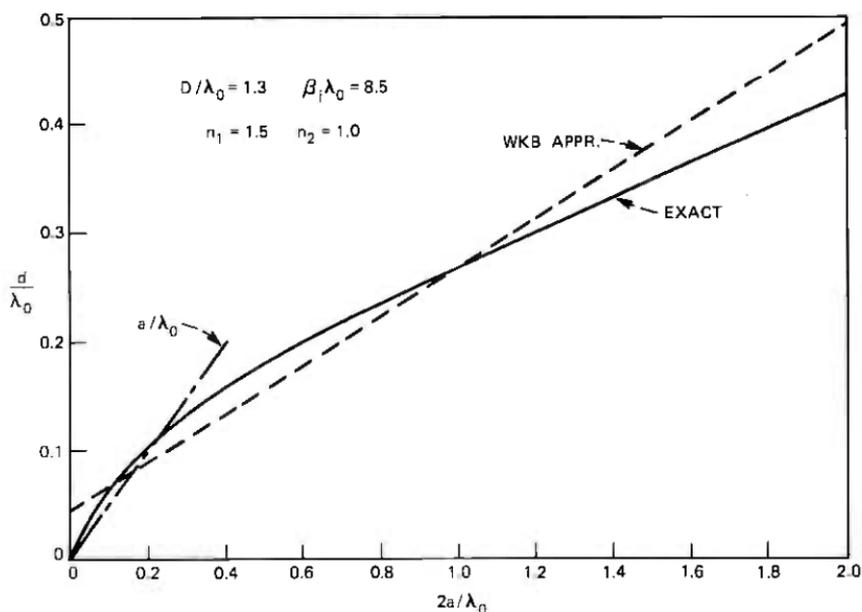
Fig. 12—Position  $d$  of the effective reflection plane as a function of grating amplitude  $2a$  for  $D/\lambda_0 = 1.3$ ,  $\beta_i \lambda_0 = 8.5$ ,  $n_1 = 1.5$ , and  $n_2 = 1.0$ . The effective reflection plane is practically independent of  $D_1$ . The solid line is obtained from the exact theory while the dotted line was computed from the wkb approximation.
