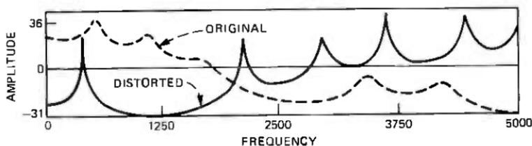
Fig. 5—Comparison of the distorted LPC spectra and the original LPC spectrum. Distance between the spectrum equals 3.0.
