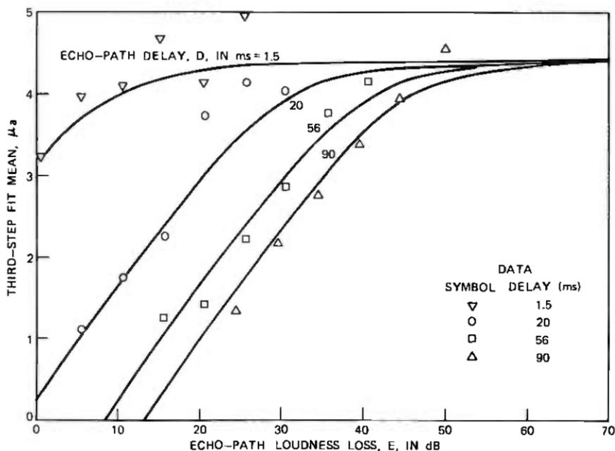
Fig. 24—1968 laboratory echo test (noise=18 dB<sub>rnc</sub>, loss=10 dB) Step 3 means from data as a function of echo-path loss and delay compared with means predicted from the loss-noise-echo model at the echo 1 base.
