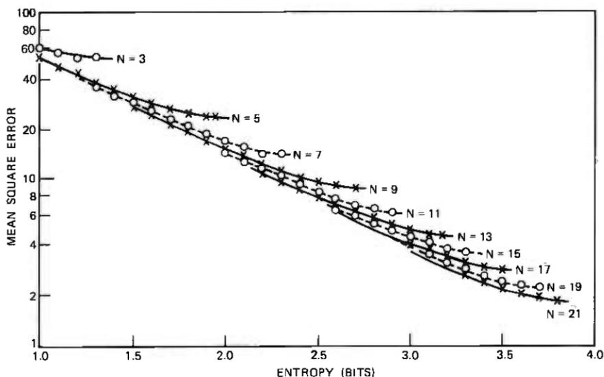
Fig. 2—Quantizer performance for Laplacian density.
