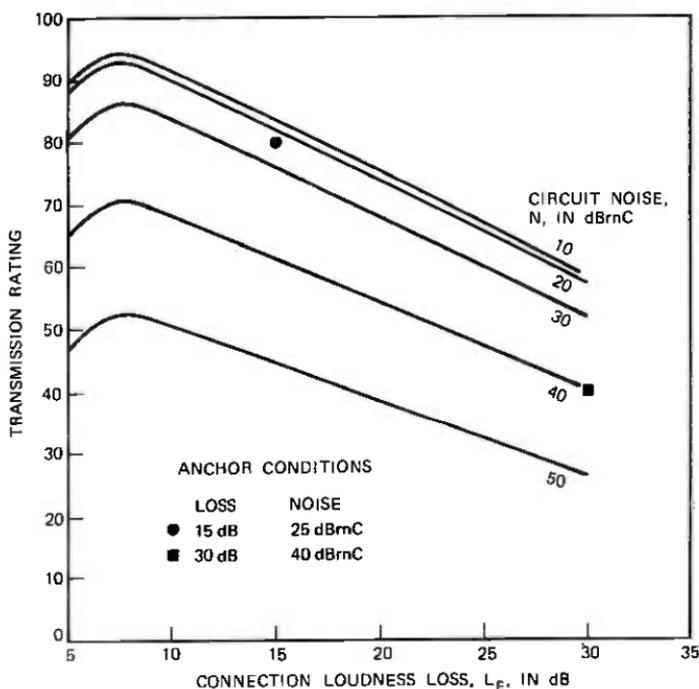
Fig. 1—Transmission rating for loss and noise.
