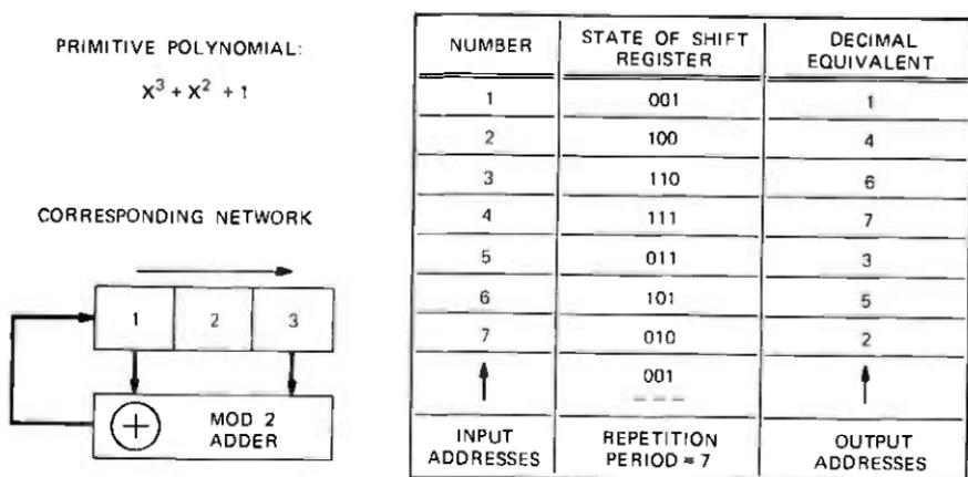
Fig. 2—Scrambler design with a three-stage shift register.
