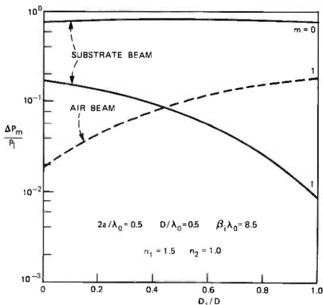
Fig. 8—Grating with only first order lobes.  $D/\lambda_0 = 0.5$ ,  $\beta_1\lambda_0 = 8.5$ ,  $n_1 = 1.5$ ,  $n_2 = 1.0$ , and  $2a/\lambda_0 = 0.5$ . The dotted line represents the relative scattered power in air; the solid lines represent the power in the substrate.
