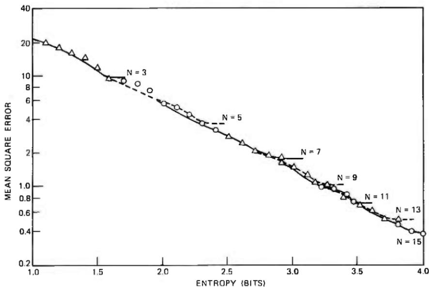
Fig. 1—Quantizer performance for uniform density. Minimum mean square error (MMSE) is plotted against entropy for a fixed number of levels ( $N$ ). Only odd-level quantizers are considered. For each fixed number of levels, MMSE decreases with entropy up to a certain point, after which there is no further decrease in mean square error.
