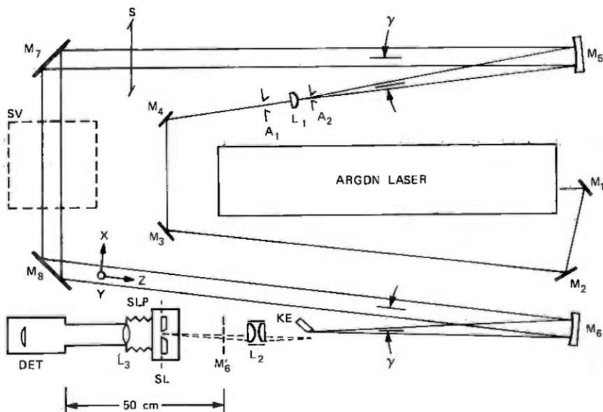
Fig. 1—Optical component layout of the MK VI small-angle-scattering instrument. Component sizes and spacings are shown approximately to scale.
