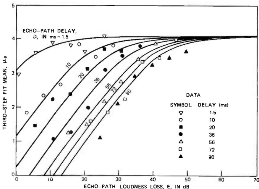
Fig. 25—1968 laboratory echo test (noise=28 dB<sub>rnc</sub>, loss=10 dB) Step 3 means from data as a function of echo-path loss and delay compared with means predicted from the loss-noise-echo model at the echo 1 base.
