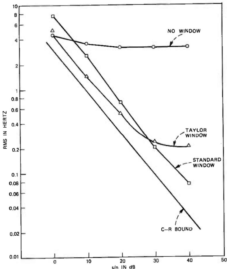
Fig. 7—Simulation results showing combined effects of bias and variance on frequency estimation for one of two complex tones. Frequency difference is 380 Hz; worst-phase was used for each window.  $N$  is 64.
