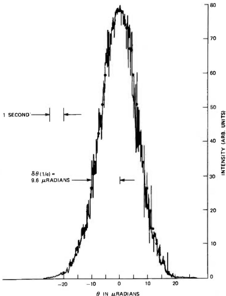
Fig. 15—Observed instrumental profile as measured by a tangential direction scan in the instrument's tangential focal plane. The heavy dots are a best fit to the function  $\exp[-\theta^2/\delta\theta^2(1/e)]$ .
