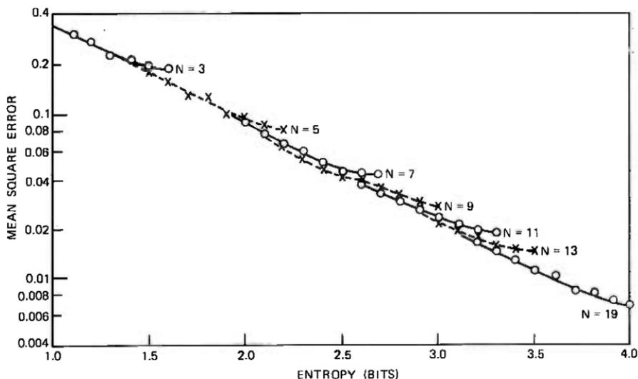
Fig. 3—Quantizer performance for gaussian density.
