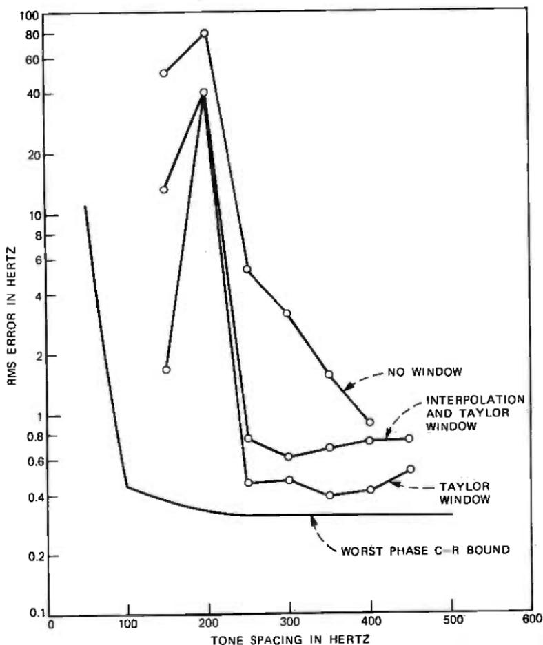
Fig. 8—Simulation results showing effects of Taylor window and interpolation algorithm upon frequency estimates of center tone of three equally spaced real tones. Center tone frequency is 2000 Hz. All have random phase.  $N$  is 128 and  $s/n$  is 20 dB.
