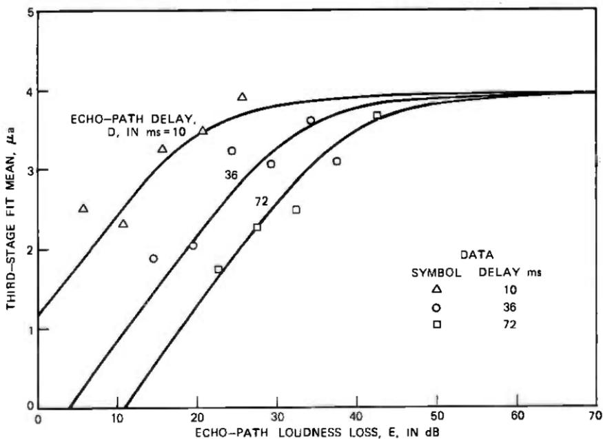
Fig. 27—sibilant echo test, Step 3 means from data as a function of echo-path loss and delay compared with means predicted from the loss-noise-echo model at the echo 1 base.
