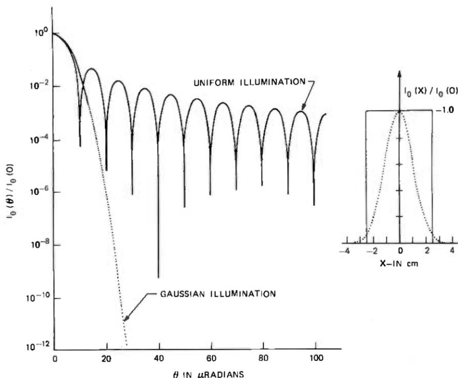
Fig. 7—Calculated instrumental profiles for uniform and gaussian illumination with  $b = 5.0$  cm and  $\sigma$  chosen to give equal values of  $\delta\theta(\frac{1}{2})$  for both profiles. The normalized illumination functions for each case are shown inset on a linear intensity scale.
