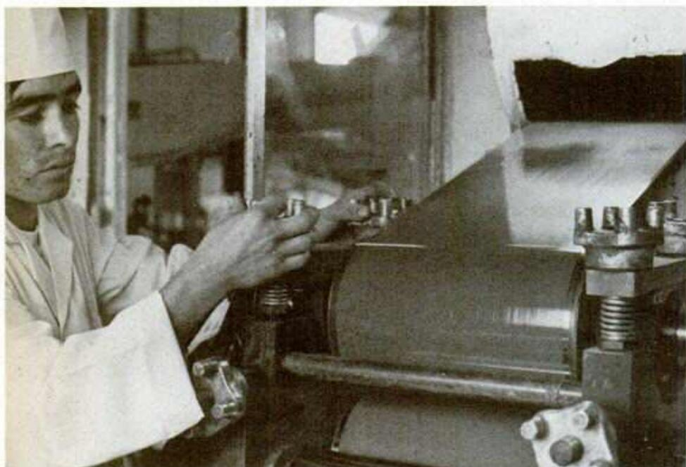
Technician checks the tension on a roll of tape—one of the key production steps.
