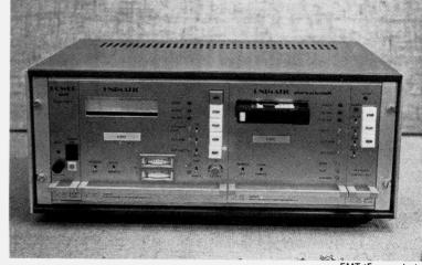
First view of prototypes of the EMT/Franz Unimatic studio record/playback system, using 1/4-inch BASF Unisette configuration, displays four of six plugin units for typical use, all built by Nordisk Elektroakustik in Denmark. From left in table-top module (rack mount also available) are power unit, recorder, playback unit and local/remote control panel.
