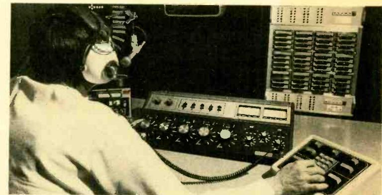
**Live Automation:** Air personality enters another cartridge for airplay on the Marc VII developed by IGM. Go-Cart unit is at left, built into the wall, and Instacart unit at right. TV screen is in the center. Keyboard under disk jockey's fingers is used to program all items and control information on the screen.
