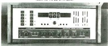
CROWN 9L-2 preamp controller, above, is claimed as first audio component designed to interface with a computer to form an automated FM radio programming system, for example; Soundcraftsmen SP4002 signal processor/ preamp provides octave-wide EQ, sub-sonic filtering, 3-way tape recorder dubbing, monitoring.
