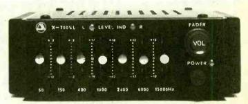
PYRAMID X700-VL amplifier/equalizer is one of smallest car units, offers 7band, center-detented slide tone controls, 44 watts RMS/channel, input sensitivity LEDs.
