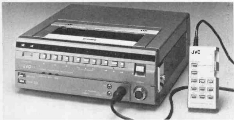
JVC's Vidstar HR-2200U is an ultra-lightweight, compact portable color videotape recorder. With battery pack, weight is 11.4 pounds. Among its features are slow motion playback, freeze frame and single frame advance.
