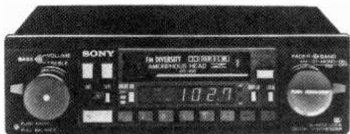
Sony Car Stereo's XR-100 model uses the diversity reception system to eliminate multipath distortion that occurs when direct and reflected FM signals are picked up at a single antenna. By placing two antennas in separate locations, the XR-100's microprocessor constantly uses the strongest signal. The unit also features an auto reverse cassette deck with an amorphous tape head. It retails for \$649.95.
