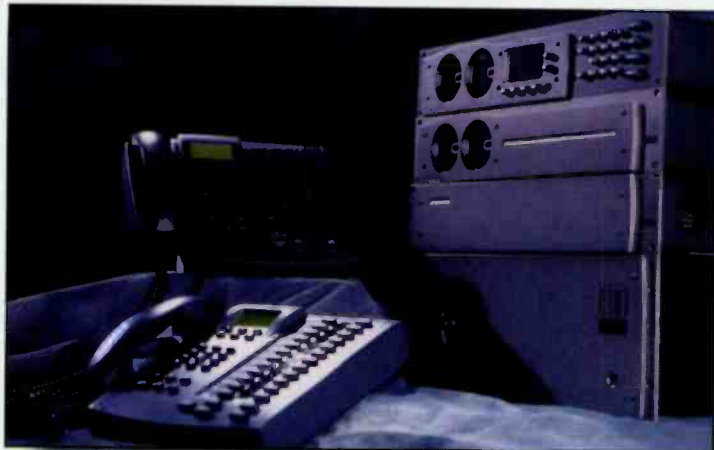
ISDN telephone systems and hybrids like the Telos 2101 provide improved audio response.
