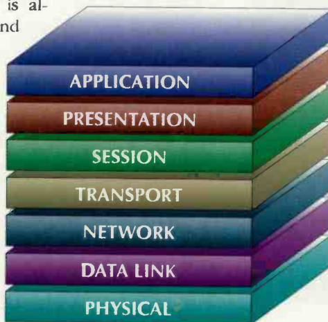
Figure 1. The OSI seven-layer model defines a standard set of network operating parameters.
