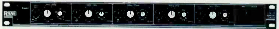
Equalizers have many different forms, functions and applications. Parametric equalizers, like this one from Rane, offer greater user flexibility but have fewer frequency bands than graphic equalizers.
